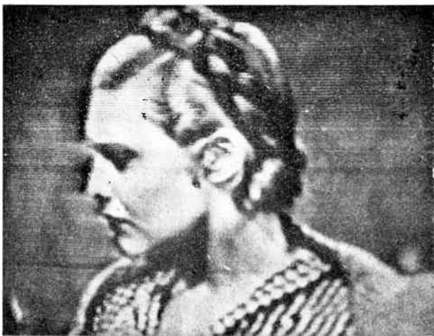
FIG. 21.—Showing the result of over-correction, and slight over-modulation.
