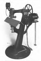
Fig. 13. Wire stitcher operated by a one-eighth horsepower motor. This motor is started and stopped by mesns of a snap switch in a similar manner to the one driving the numbering machine
