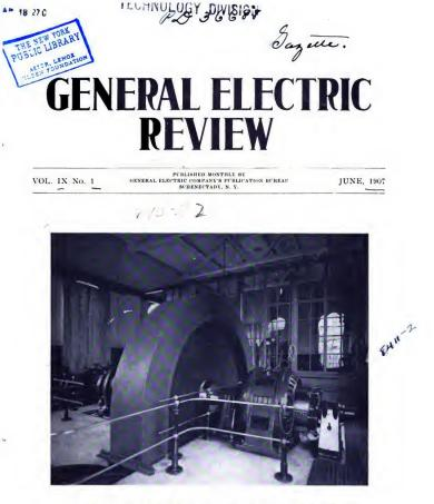
Sixteen Ton Flywheel Motor Generator for Hoisting Engine Plant at Wintershall Mine.
