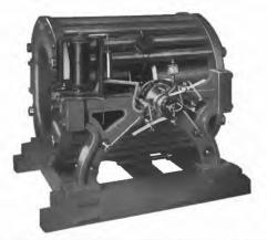
Fig. 2. Thomson-Houston Arc Light Dynamo, Showing Regulator and Brush Mechanism
