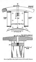
sively used by the General Electric Company. This is the patent to Parcelle, dated Nov. 24, 1891, No. 403,704, which covers a method of firmly fastening a laminated pole piece to a solid yoke.
