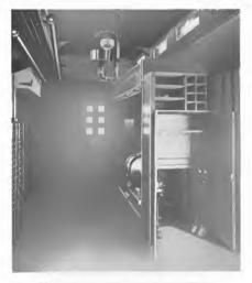
Fig. 1. 15 kw. D.C. Curtis Steam Turbine Installed in Baggage Car
