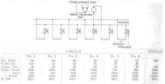
Fig. 1. Diagram of Connections and Table for Charging Group of Batteries from Motor Generator
