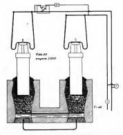
Fig. 7. Diagram Showing Electrical Connections of Keller Furnace with Two Hearths
