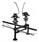
Fig. 7, A Skew Sketch Showing the Relative Connection of the Aluminum Arrester for a Non-Grounded Neutral Circuit, or a Circuit with the Neutral Grounded Through a Resistance
