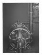
Fig. 2. 25 kw. 118 Volt D. C. Curtis Steam Turbine Installed in Baggage Car
