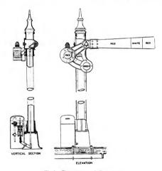
Fig. 5. Electro-pneumatic Semaphore
