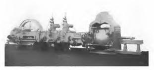
Later Type of Blowing Gas Engine as Built by The John Cockerill Works, Seraing, Belgium
