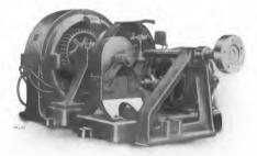
Fig. 4. Self-contained Set for Driving Cylinder Press. Push Button Control
