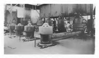
Fig. 5. 1-6-40-500-K-440 volt vertical motors, belted to Fuller mills, Plant No. 4, Universal Portland Cement Co. There are eight of these driven altogether. The bearings on these motors have given entire satisfaction in spite of the dust and grit that naturally tend to produce excessive wear
