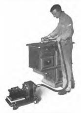
Fig. 1. Stove Polishing Apparatus Driven by 1 2 h.p. Single-Phase General Electric Motor
