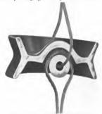
Fig. 3. Cross Section of Link Strain Insulator
