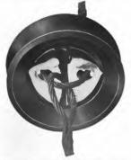
Fig. 4. Link Strain Insulator which has been broken under a load of five tons.
