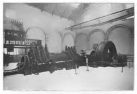
1200 H. P. Nurnberg Double-Acting Single Tandem Gas Engine Driving 825 Kw. Three Phase Alternator at Powell Duffryn Coal Co.
