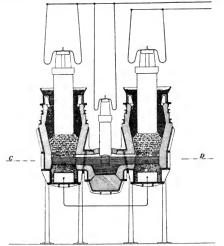
Fig. 9. Keller Electric High Furnace with a Plurality of Hearths
