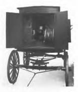
Fig. 1. Rear View of Portable Motor Driven Drainage Pump
