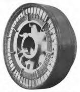
Fig. 7. Rear View of Armature Showing Equalizer Rings
