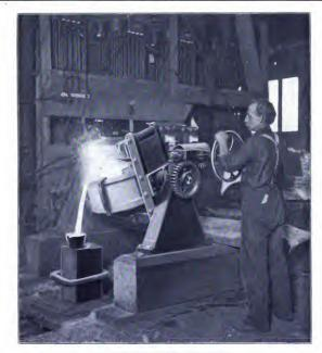
60 KW. INDUCTION FURNACE Copyrighted by American Electric Furnace Co.; reproduced by permission.)
