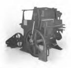
Fig 7 Thirty-eight inch paper cutter, driven by a standard compound wound motor, the controller being situated directly beneath the feed board
