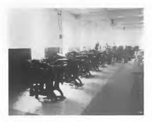
Fig. 12. Row of Gordon Job Presses driven by Individual Motors
