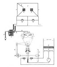
Fig. 2. Diagram of Automatic Regulator for Heroult Furnace
