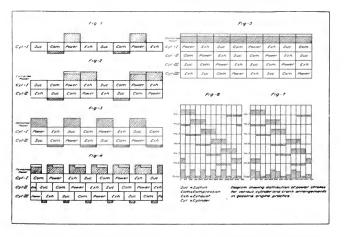
the relation of events in four-cycle engines having cylinders and eranks arranged according to the more usual practice met in explosion-engine design. No attempt is made to show the variation of pre-sure during the several strokes, but each is represented by a rectangle. The sectioned rectangles above the lines represent positive or useful work, while those below show negative effort in compressing the charge of vapor. Explosion strokes are indicated by in first case, but imbalanced in second.
