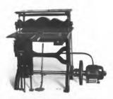
Fig 9. Perforator driven by a one half horsepower motor, the controller being attuated directly beneath the feed board
