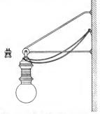
Fig. 1. Arc Lamp Bracket in Regular Use by The Detroit Edison Illuminating Co.
