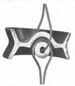
Fig 6. Cross Section of Link Strain Insulator
