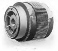
Fig. 3. Armature Partly Wound
