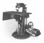
Fig. 8. Paging and numbering machine operated by a oneeighth horsepower motor. This motor is atopped and started by means of the snap switch shown at the side of the machine head
