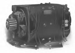
Fig. 3. GE-205 Commutating Pole Railway Motor
