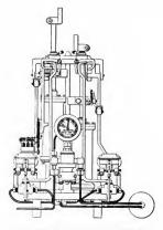
Fig. 7. Elevation of Two-arm Electro-gas Signal
