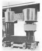
Fig. 4. Transformer of 736 Kw. Induction Furnace (Copyrighted by American Electric Furnace Co.; reproduced by permission)
