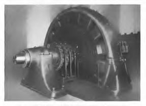
Fig. 1. 16 Pole, 2000 Kw., 188 R.P.M., 600 Volt Six-Phase Rotary Converter
