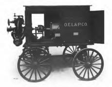
Fig. 2. Side View of Portable Motor Driven Pump
