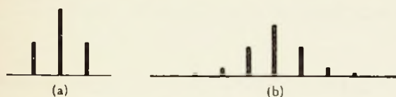
FIG. 100. Amplitude and frequency position of the components making up (a) a wave which is amplitude modulated by a sinusoid to m_a = 1.0 and (b) a wave which is frequency modulated by a sinusoid to m_f = 1.0 .
