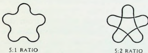
FIG. 46. Images obtained when a sinusoidal test signal having an integral relationship with the sweep frequency is applied to a polar-coordinate cathode-ray oscillograph.
