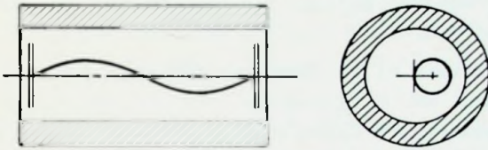
FIG. 31. Long focusing coil. The electron object lies on one of the planes at the end of the coil, and the image is formed on the other. The solid spiral line shows the path of the electron through the lens.
