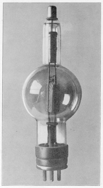
FIG. 1c.-250 watt power tube.
