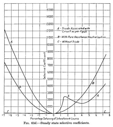
frequencies detuned by 1 or 2 per cent which results from the rapid increase of the reactance and the addition of resistance at frequencies slightly removed from the resonant frequency is illustrated by these curves.
