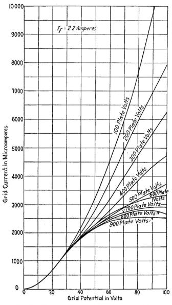
FIG. 7.-Characteristic curves of 100 watt power tube.
