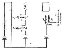
FIG. 66.-Grid circuit modulator.
