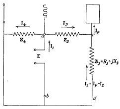
FIG. 64.—Generalized amplifier circuit.
