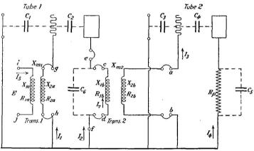
FIG. 79.-Two stage transformer coupled amplifier.
