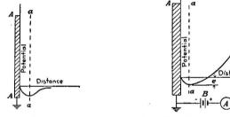
FIG. 2a.—Potential distribution near heated plate. FIG. 2b.—Potential distribution between hot plate and charged cold plate.
