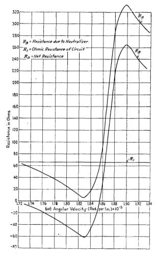
FIG. 63b.-Relation between resistance and impressed frequency.
