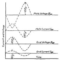
FIG. 19.—Potentials and currents in simple amplifier circuit.
