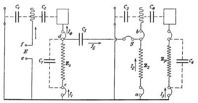
FIG. 76.-Two stage impedance coupled amplifier.
