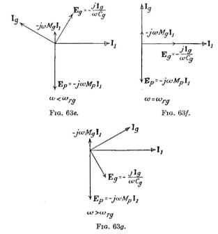
FIGS. 63e, f and g.—Approximate vector diagrams for the circuit of Fig. 63a Cases for which  $M_p$  is positive and  $M_g$  is negative.
