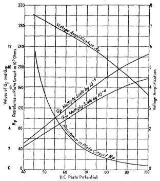
FIG. 78.—Variation of voltage amplification with output resistance when a source of constant plate potential is used.
