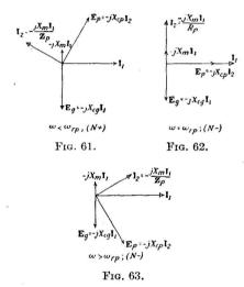
FIGS. 61, 62 and 63.—Approximate vector diagrams for the circuit of Fig. 57. Cases for which M is negative.
