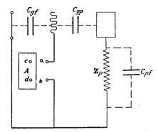
FIG. 72 .- Triode amplifier with impedance in the output circuit.
