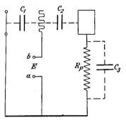
FIG. 75.—Triode amplifier with resistance in output circuit.
