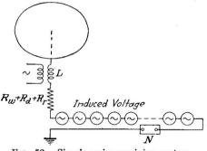
FIG. 52.-Simple series receiving system.
