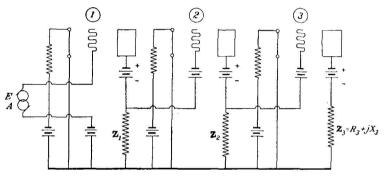
FIG. 15.-Impedance coupled amplifier.
