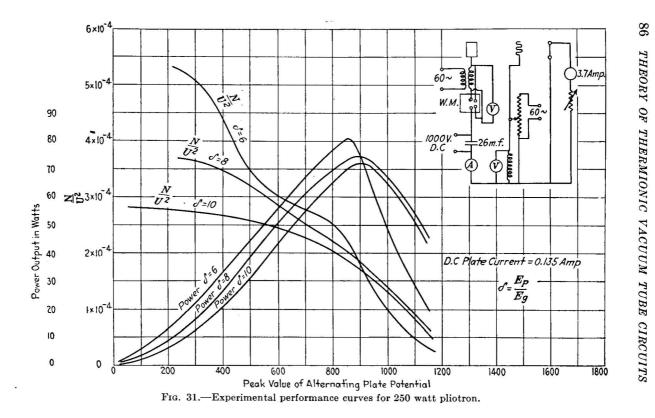
given by Fig. 30. The  $\frac{N}{U^2}$  curves can be obtained from these power curves by making use of Eq. (79), for
