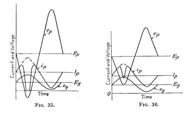
This follows from the discussion of Sec. 10, Chap. II. When these conditions are fulfilled, Eq. (5) shows that maximum power output obtains when the plate voltage and plate current have the largest feasible variation. Now the peak value of the plate alternating voltage should not exceed the continuous voltage applied to the plate, nor should it be of such a value as to make the total plate poten-
