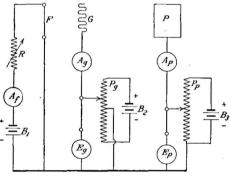
FIG. 5.-Circuit for obtaining characteristics.
