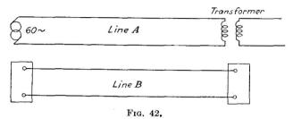
effect of line A upon line B. We will suppose that line A is a low-tension line so that the electrostatic effects can be neglected. The current in line A is the magnetizing current of the transformer and therefore this current has the form shown by Fig. 43. This current can be broken up into the two sine waves shown by Fig. 44 and a number of smaller
