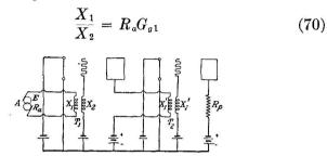
FIG. 18.-Transformer coupled amplifier.
