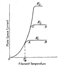
FIG. 4.—Characteristic curves of two element tube.
