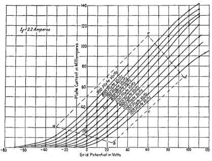
FIG. 6.-Characteristic curves for a 100 watt power tube.
