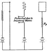
FIG. 68.-Demodulator circuit.
