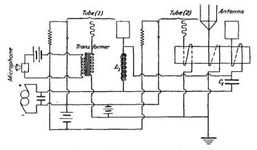
FIG. 69.-Plate circuit modulator.
