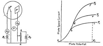
FIG. 3.—Connections for obtaining FIG. 3a.—Characteristic curves of two characteristics. element tube.
