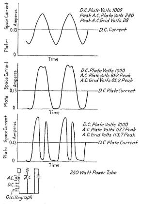
FIG. 37.—Oscillograms showing effect of increased plate voltage on plate current.
