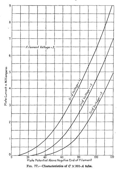
continuous potential impressed on the plate. If the plate voltage is to be 135 volts, the resistance in the plate circuit must be 0. If the plate voltage is to be 70, the plate space
