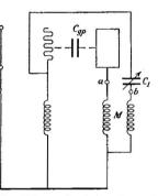
FIG. 81.—Scheme for balancing out the effects of plate to grid capacitance.
