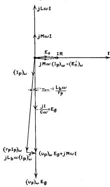
FIG. 185.--Vector diagram for the regenerative triode shown in Fig. 184.
