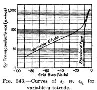
Fig. 343, taken from the paper by Ballantine and Snow.<sup>5</sup> Figure 344<sup>6</sup> shows the transconductance of a variable-u tube which is logarithmic over a larger range than the tube of Fig. 343 and is hence better adapted to logarithmic recording.
