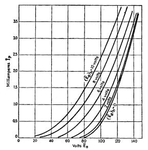
FIG. 301.—Plate-circuit detection characteristics or transrectification diagram. Triode ER201A.  $E_e = -9$  volts.
