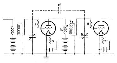
FIG. 256.--Neutralization through inherent capacitance.
