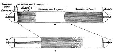
FIG. 6.—Electric discharge through a gas at reduced pressure.
