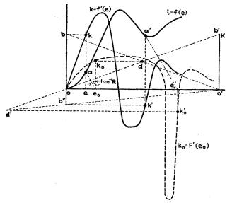
FIG. 293b.—Derivation of curve of  $k_0 = F'(e_0)$  from curve of k = f'(e).
