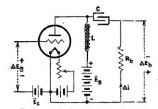
FIG. 161.-Resistance-loaded amplifier using parallel feed.
