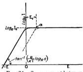
Fig. 24.—Space current between plane parallel electrodes as a function of retarding potentials.
