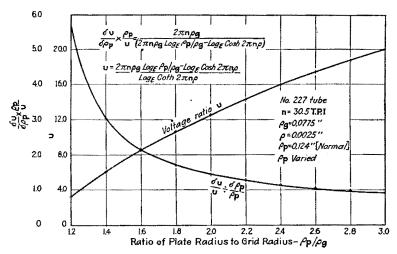
F1G. 83.—Variation of u with ratio of plate radius to grid radius for a triode having cylindrical electrodes. Plate radius varied.
