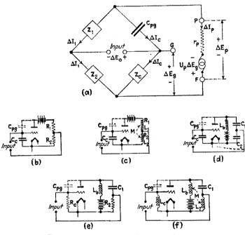
FIG. 247.-Neutralization by voltage balance.
