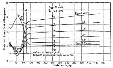
FIG. 327.—Curves of  $i_p$  vs.  $e_p$  and  $i_{a_2}$  vs.  $e_p$  for tetrode UY224. (R.C.A. Radiotron Handbook.)
