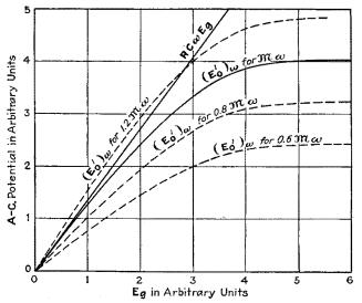
F10. 186.—Curves of  $C\omega RE_g$  and  $(E_0')_\omega$  vs.  $E_g$  for large-signal regeneration
