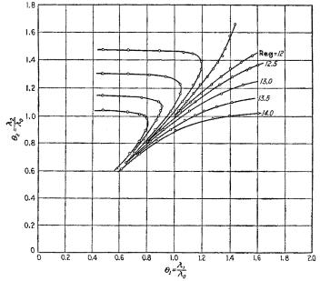
FIG. 224-2.—Experimental boundary curves. Effect of varying regeneration,  $\lambda_{\theta} = 600$  meters.
