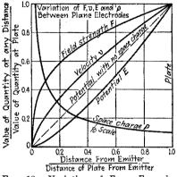
FIG. 19.—Variation of F,  $v_{i}E$ , and  $\rho$  between parallel plane electrodes.
