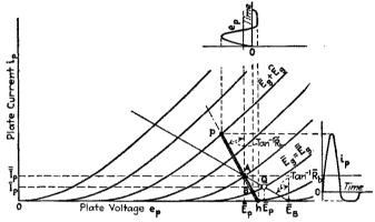
Fig. 105.—Path of operation on a curved region of the characteristic surface  $\vec{R}_b \neq \vec{R}_b$ .  $e_g = \vec{E}_g \sin \omega t$ .
