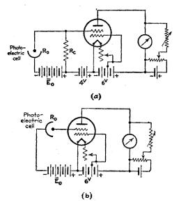
FIG. 346.-Use of low-grid-current tetrode.
