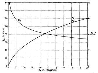
FIG. 228.—Variation of  $k_p/K_b$  and  $\vec{E}_p$  with  $R_b$  for a UX 240 triode.  $\vec{E}_c = -1.5$  volts.
