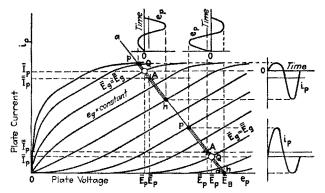
FIG. 104.—Paths of operation on curved regions of the characteristic surface. Pure resistance as plate load.  $R_b = R_b$ .  $e_q = \overline{E}_q \sin \omega t$ .
