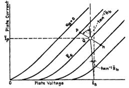
F10. 162.—Path of operation of resistance-loaded amplifier when  $\tilde{R}_b \neq \tilde{R}_b$ .
