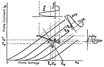
FIG. 102.—Path of operation on the plane region of the characteristic surface. Resistance load.  $\vec{R}_{b}, \neq \vec{R}_{b}$ . Grid voltage nonsinusoidal.
