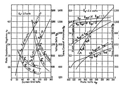
FIG. 330.—Equivalent triode coefficients of tetrode UY224, plotted against  $e_{g_2}$ . (R.C.A. Radiotron Handbook.)
