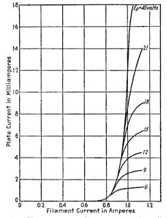
FIG. 29.-Plate current vs. filament current for a diode.
