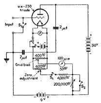
FIG. 318.—Vacuum-tube voltmeter  $u_p = 9.3$ ;  $C_{gf} = 3.7 \mu \mu f$ ;  $C_{pg} = 6.4 \mu \mu f$ .
