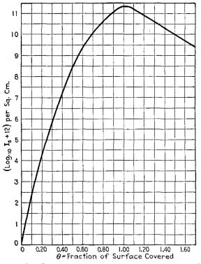
FIG. 39.—Log  $I_s$  vs.  $\theta$  for a film of barium on tungsten. (Becker.)
