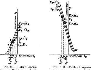
FIG. 99.—Path of operation on the  $i_p - e_q$  chart. Path on the plane region of the characteristic surface.  $\Delta e_q = \Delta E_q \sin \omega t$ .
