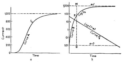
FIG. 40.-Rate of activation of thoriated-tungsten filaments. (Langmuir.)
