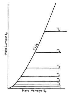
FIG. 27.-Plate current vs. plate voltage for the diode.
