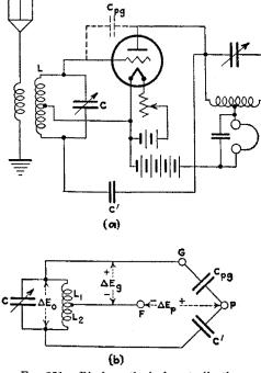
FIG. 251.—Rice's method of neutralization.
