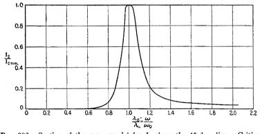
FIG. 206.—Section of the space model for  $I_2$  along the 45-deg. line. Critical coupling.  $\eta_1 = \eta_2 = 0.10$ .  $\tau = 0.10$ .
