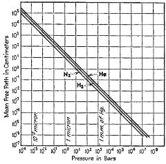
FIG. 3.—Mean free path of gas molecules of hydrogen, helium, and nitrogen at  $20^{\circ}$ C.
