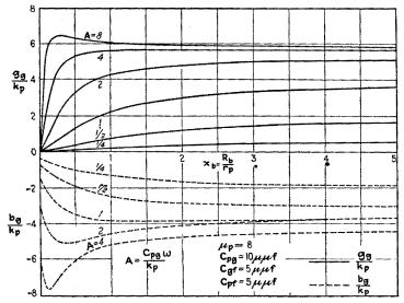
F16. 150.—Components of the input admittance of a triode when  $k_q = 0$  and  $B_b = 0$ .
