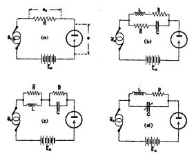
FIG. 294.-Circuits containing a nonlinear element.
