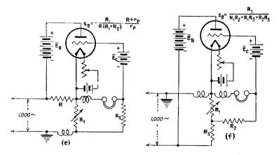
FIG. 123.—Circuits for the measurement of  $s_p$  and  $s_q$ .
