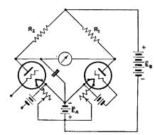
FIG. 315.—Bridge-type vacuum-tube voltmeter with balancing triode.
