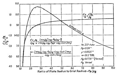
F1G. 84.—Variation of u with ratio of plate radius to grid radius for a triode having cylindrical electrodes. Grid radius varied.
