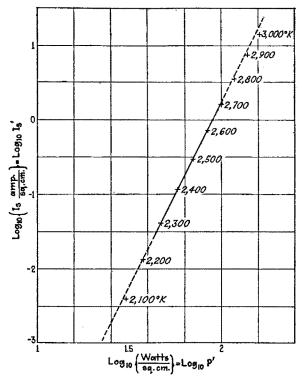
FIG. 43.-Emission-power curve for tungsten.
