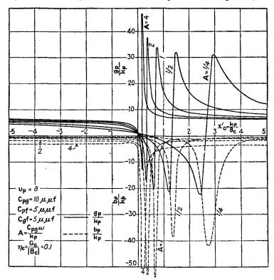
FIG. 154.—Components of the internal output admittance of a triode for various values of A when  $k_q = 0$ .
