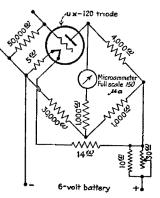
Fig. 316.—Portable bridgetype thermionic voltmeter. (General Electric Company.)
