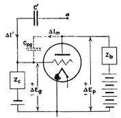
FIG. 252.—Neutralization by current balance.
