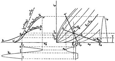
FIG. 299.—Curves for the path of operation for the plate circuit of a triode when  $\overline{R}_b \neq \widehat{R}_b$ .
