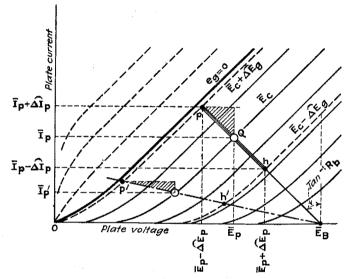
Fig. 160.—Path of operation of a triode used as an amplifier with a resistance load.
