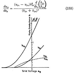
FIG. 87.-Ratio of plate conductances of two triodes.
