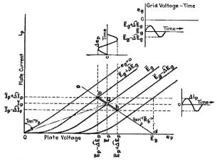
FIG. 97.—Path of operation on the  $i_p - e_p$  chart. Pure resistance as plate load. Path on the plane region of the characteristic surface.  $\Delta e_g = \Delta \hat{E}_g$ sin  $\omega t$ .
