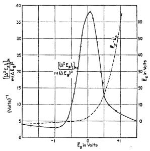
FIG. 284.—Grid-circuit detection.  $u_p = 20$ ;  $\overline{E}_B = 60$  volts;  $R_c = 2.94$  megohms;  $C_c = 200 \mu \mu$ f;  $w_l = 2\pi 1,000$  radians per second.
