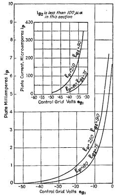
FIG. 341.—Curves of  $i_p$  vs.  $e_{q_1}$  for variable-u pentode, type 235 with suppressor grid. (*R.C.A. Radiotron Handbook.*)
