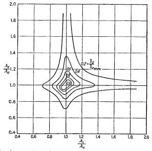
FIG. 197.—Contour lines of constant secondary current for critical coupling. ratio given by Eq. (396) has a single maximum at values of the independent variables
