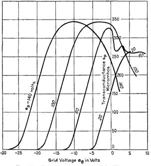
FIG. 66.---Transconductance of a triode (UV 201).
