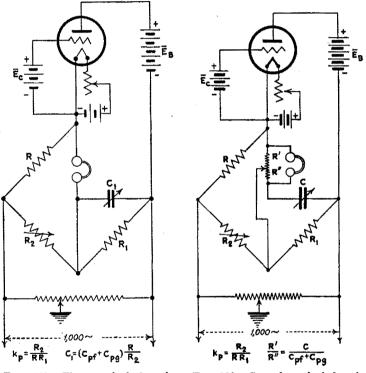
FIG. 119.—First method for the FIG. 120.—Second method for the measurement of  $k_p$ .
