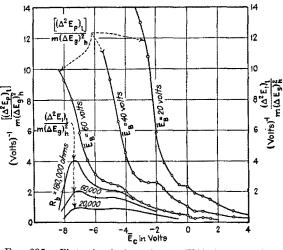
FIG. 285.—Plate-circuit detection. UX201A.  $u_p = 8.5$ .
