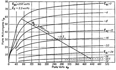
F10. 339.—Curves of  $i_p$  vs.  $e_p$  for pentode type 247 with suppressor grid.  $\vec{E}_{e_2} = 250$  volts;  $\vec{E}_{e_3} = 0$ . (R.C.A. Radiotron Handbook.)
