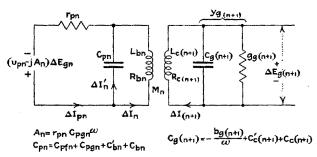
FIG. 241.--Equivalent a-c. circuits of the transformer-coupled amplifier.
