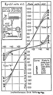
Fig. 337.-Characteristics of two tetrodes type 46 used as Class B amplifiers.
