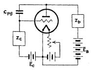
FIG. 179.—Circuits of a triode, with capacitance coupling between the grid and plate circuits.
