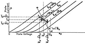
FIG. 101.—Path of operation on the plane region of the characteristic surface. Resistance load.  $\vec{R}_b \neq \vec{R}_b, \Delta e_g = \Delta \vec{E}_g \sin \omega t.$
