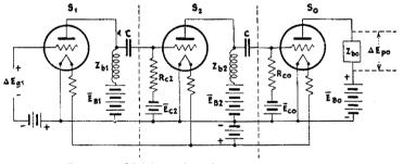
FIG. 236.-Multistage impedance-coupled amplifier.
