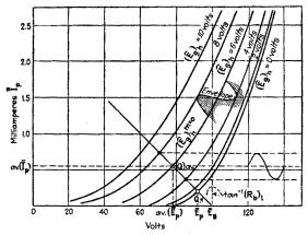
FIG. 304.--Rectification diagram and resistance line.
