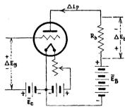
FIG. 158.—Triode with pure resistance as plate load.
