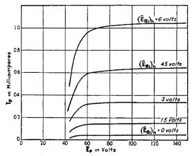
FIG. 333.—Plate-circuit detection characteristics of tetrode ER224.  $\vec{E}_A = 2.5$  volts;  $\vec{E}_{\theta_2} = 45$  volts;  $\vec{E}_{\theta_1} = -4.5$  volts.
