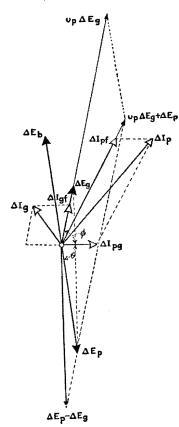
FIG. 114.—Vector diagram of an oscillator with back.
