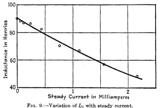
FIG. 5.—Variation of Li with steady current.
