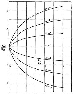
FIG. 141.—Values of  $[g_0]/k_g$  for  $X_b = 0$  and negligible tube capacitances.
