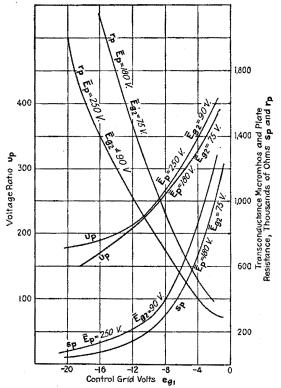
FIG. 342.—Equivalent triode coefficients of variable-u pentode, type 235. (R.C.A. Radiotron Handbook.)
