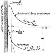
FIG. 32.—Schottky's picture of the The resultant potential has a force and potential near a surface of metal. No external impressed force.
