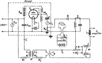
FIG. 271.-Measurement of detection by diode.
