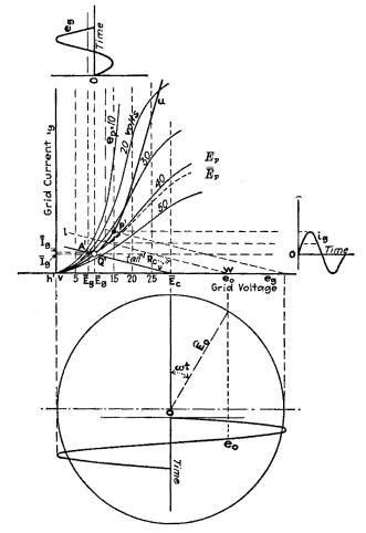
FIG. 108.—Path of operation on the grid-current surface when  $\tilde{R}_b = \tilde{R}_b$  and  $\tilde{R}_c = \tilde{R}_c$ .
