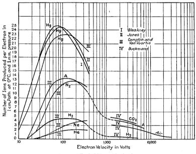
FIG. 5.-Probability of ionization.
