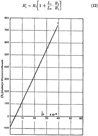
FIG. 10.—Determination of the distributed capacitance of the secondary winding of transformer AD1.
