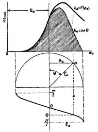
FIG. 290.—Calculation of the amplitude of the fundamental component of current from the curve of  $k_0$ .
