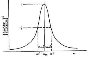
FIG. 166.—Variation of  $(V.A.)_{\omega}$  with frequency for an amplifier having a tuned plate load.
