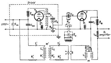
FIG. 282.—Measurement of detection by a triode.
