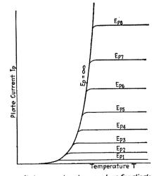
Plate current vs temperature for diode FIG. 28.—Plate current vs. temperature for the diode.
