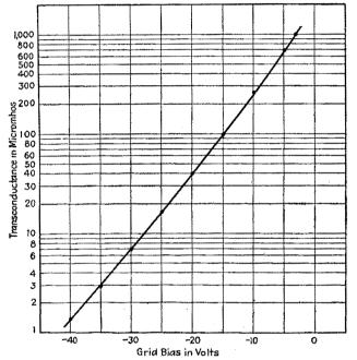
FIG. 344.—Transconductance of an exponential tetrode. (Ballantine.)
