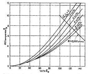
FIG. 310.—Grid-circuit detection characteristics or transrectification diagram. Triode ER201A.
