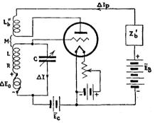
FIG. 174.—Circuits of a regenerative triode.
