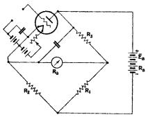
FIG. 314.—Bridge arrangement of vacuumtube voltmeter.
