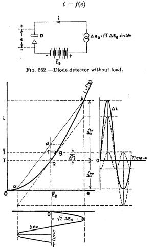
FIG. 263.—Rectification by two-electrode non-linear circuit element without load.
