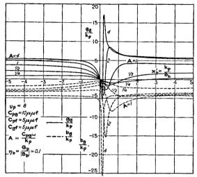
FIG. 152.—Components of the input admittance of a triode when  $k_g = 0$ .  $\eta_b = \frac{G_b}{[B_b]}$  for various values of A.
