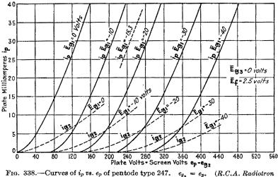
FIG. 338.—Curves of  $i_p$  vs.  $e_p$  of pentode type 247.  $e_{\sigma_2} = e_p$ . (R.C.A. Radiotron Handbook.)
