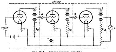
FIG. 234.-Direct-current amplifier.
