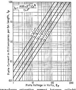
FIG. 21.—Space-charge saturation current between cylindrical electrodes.  $\beta^2 = 1.$
