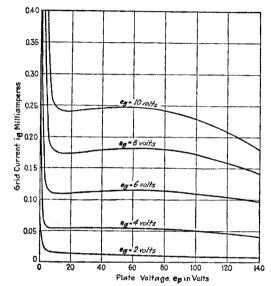
FIG. 65.—Static characteristic curves of a triode.  $i_{q} - e_{p}$  curves for constant grid voltage (UV 201).
