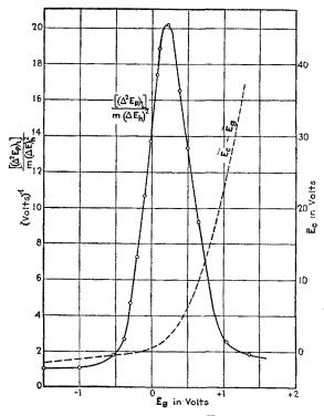
FIG. 283.—Grid-circuit detection.  $u_p = 8.5$ ;  $\overline{E}_B = 60$  volts;  $R_c = 2.94$  megohms;  $C_c = 200\mu\mu$ f;  $w_l = 2\pi 1,000$  radians per second.
