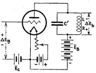
FIG. 165.—Amplifier with a tuned plate load.
