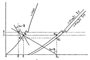
FIG. 295.—Curves of  $i = F(e_0, \overline{I})$  derived from curve of i = f(e), showing transformation of a kink in the curve.
