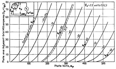
FIG. 335.—Curves of  $i_p + i_{a_2}$  vs.  $e_p$  for tetrode type 46. (R.C.A. Radiotron Handbook.)
