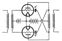
FIG. 257.-Neutralization of "push-pull" amplifier.
