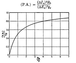
FIG. 159.—Variation of (V.A.) of an amplifier with the resistance of the plate load.
