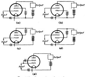
FIG. 320.-Connections of tetrodes.
