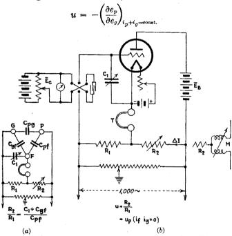
FIG. 116.—First method for the measurement of u, and  $u_p$  (if  $i_q = 0$ ).
