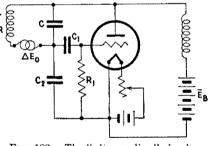
FIG. 183.—The "ultra-audion" circuits.
