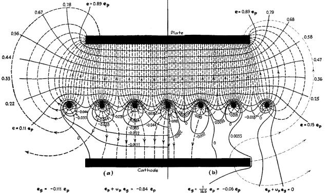
FIG. 75.-Equipotential lines and lines of force in a triode having plane electrodes. Paths of electrons shown in red.
