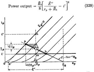
F1G. 171.—Construction for maximum undistorted power output when  $\overline{E}_B$  is given.
