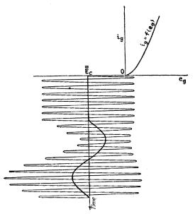
FIG. 307.-Grid-circuit detection with large-signal voltage.
