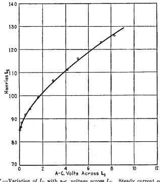
Fig. 7.—Variation of  $L_1$  with a.c. voltage across  $L_1$ . Steady current equal to zero. (Transformer AD1.)
