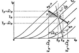
FIG. 167.—Path of operation of an amplifier having a tuned plate load set at resonance.
