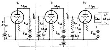
FIG. 225.-Multistage resistance-coupled amplifier.
