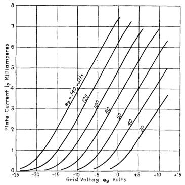
FIG. 63.—Static characteristic curves of a triode.  $i_p - e_q$  curves for constant plate voltage (UV 201).
