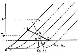
FIG. 172.—Construction for maximum undistorted power output when  $\overline{E}_{p}$  is given.
