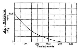
FIG. 173.---Transient current in circuit of Fig. 161.
