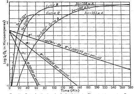
FIG. 41.—Rate of activation of a thorized-tungsten filament at temperature  $T_a$  after flashing at 2800° K. (Langmuir.)
