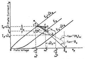
FIG. 103.—Path of operation on the plane region of the characteristic surface.  $\vec{R}_b \neq \vec{R}_b$  and  $X_b \neq 0$ .  $\Delta e_q = \Delta \vec{E}_q \sin \omega t$ . Arrows give direction for capacitive reactance.
