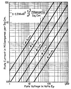
FIG. 18.—Space-charge saturation current between parallel plane electrodes.
