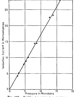
FIG. 137.--Positive-ion current vs. pressure.
