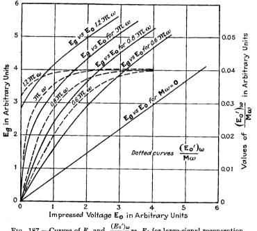
F13. 187.—Curves of  $E_{\sigma}$  and  $\frac{(E_0')\omega}{M\omega}$  vs.  $E_0$  for large-signal regeneration.
