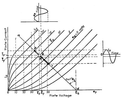
FIG. 107.—Path of operation on the plate-current surface when  $\tilde{R}_b = \bar{R}_b$  and  $\tilde{R}_c = \bar{R}_c$ . Grid current not zero.
