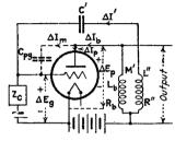
FIG. 254.—Neutralization by current balance (Hazeltine).
