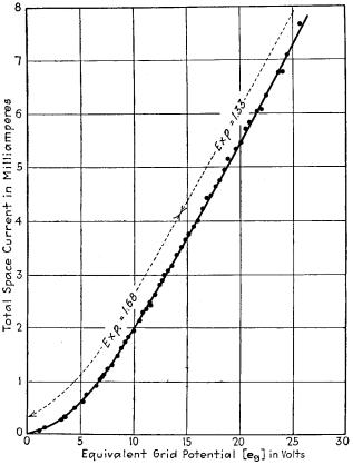
FIG. 55.—Total space current vs. equivalent grid voltage. Tungsten filament (UV 201). D = 0.181.
