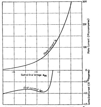
FIG. 345.—Average characteristics of tetrode type FP54.  $\overline{E}_f = 2.5$  volts;  $\overline{E}_{g_1} = 4$  volts;  $\overline{E}_p = 6$  volts.
