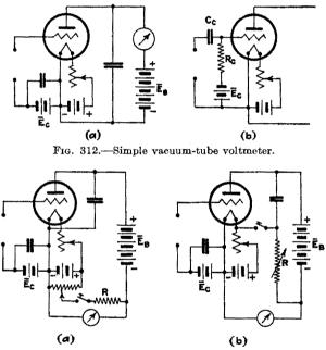
FIG. 313.-Vacuum-tube voltmeter with zero adjustment.
