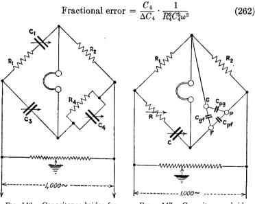
FIG. 146.—Capacitance bridge for the measurement of the capacitance of a leaky condenser.
