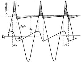
FIG. 308.-Voltages and grid current in grid-circuit detection.
