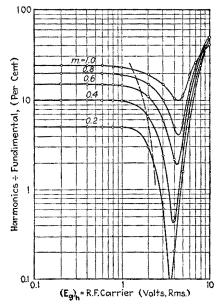
FIG. 305.—Distortion in plate-circuit detection. (Ballantine.) Triode 201A.  $\tilde{E}_B = 90$  volts;  $\tilde{E}_c = -4$  volts;  $R_b = 100,000$  ohms;  $w_l/2\pi = 400$  cycles per second.
