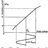
FIG. 273.—Characteristic of oscillator.
