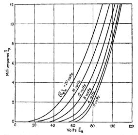
FIG. 302.—Plate-circuit detector characteristics or transrectification diagram. Triode ER171A.  $E_c = -22.5$  volts.
