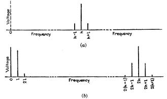
FIG. 266.—(a) Frequencies before detection.  $m = \frac{1}{2}$ . (b) Frequencies added by detection.
