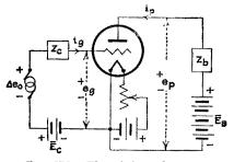
FIG. 278.-The triode as detector.
