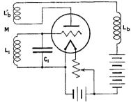
FIG. 246.—Hartley's method of reducing feed-back.
