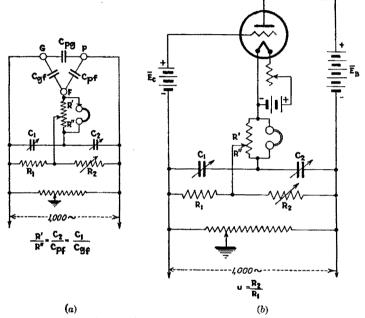
FIG. 117.—Second method for the measurement of  $u_i$  and  $u_p$  (if  $i_q = 0$ ).
