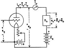
FIG. 111.-A triode and its plate load.
