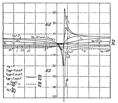
FIG. 155.—Components of the internal output admittance of a triode for various values of  $\eta_c$  when  $k_g = 0$ .  $\eta_c = G_c/[B_c]$ .
