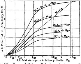
FIG. 190.—Curves of  $(E_0')_{\omega}$  vs.  $E_{\sigma}$  for large-signal regeneration.
