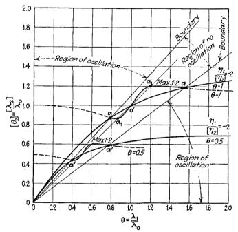
FIG. 211.—Oscillation boundary lines for constant regenerative effect. Condition of constant  $\eta$ .  $[\tau] = 0.5$ .  $\eta_1 = 0.4$ .  $[\eta_2] = -0.2$ .
