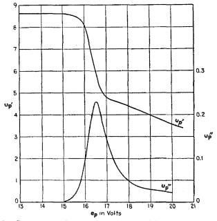
FIG. 130.—Components of  $\mathbf{u}_p$  for a triode containing gas.  $\mathbf{u}_p = u'_p + ju''_p$  $e_q = 0.$
