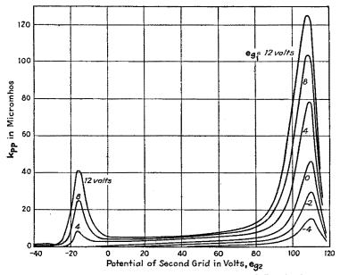
Fig. 321.—Curves of  $k_{pp}$  vs.  $e_{q_n}$  for a tetrode. (French Bigril tube.)
