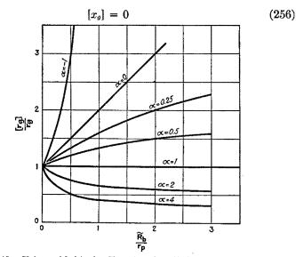
FIG. 140.—Values of  $[r_g]/r_g$  for  $X_b = 0$  and negligible tube capacitances.
