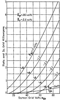
FIG. 325.—Curves of  $i_p$  vs.  $e_{a_1}$  for tetrode UY224. (R.C.A. Radiotron Handbook).
