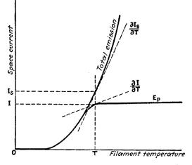
FIG. 48.-Space current vs. temperature of cathode.
