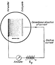
FIG. 15.—Diagrammatic illustration of space charge.
