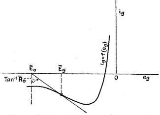
FIG. 347.-Grid-circuit diagram of low-grid-current tetrode.
