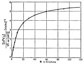
F1G. 275.—Variation of voltage of detection across series resistance R as R is varied. Carborundum detector.  $E_B = 0.62$  volt. Crystal positive.
