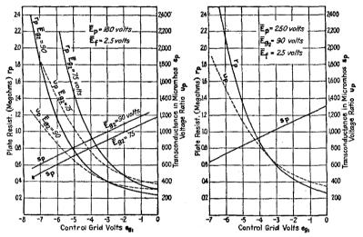
FIG. 328.—Equivalent triode coefficients of tetrode UY224 plotted against  $e_{q_r}$ . (R.C.A. Radiotron Handbook.)
