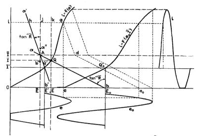
FIG. 296.—Method of the derivation of the curve of  $i = F(e_0, \bar{I})$  from the curve of i = f(e) when  $\bar{R} \neq \tilde{R}$ .
