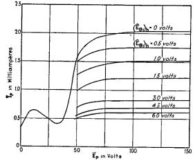
FIG. 334.—Grid-circuit detection characteristics of tetrode ER224.  $\vec{E}_A = 2.5$  volts;  $\vec{E}_{\nu_a} = 45$  volts.
