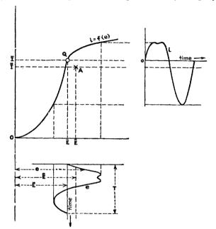
FIG. 4.—Characteristic of a conductor whose resistance is a function of the current.
