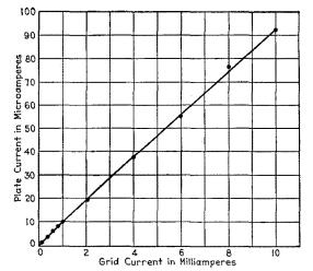
FIG. 136.—Positive-ion current vs. grid current for constant grid and plate voltages.
