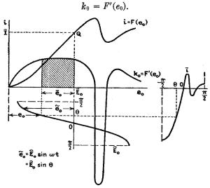
FIG. 289.—Calculation of i from  $k_0$  when a sinusoidal e.m.f. is impressed in the circuit.
