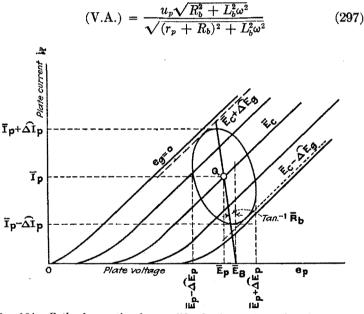
FIG. 164.—Path of operation for amplifier having an inductive plate load.
