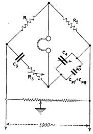
FIG. 145.—Capacitance bridge.
