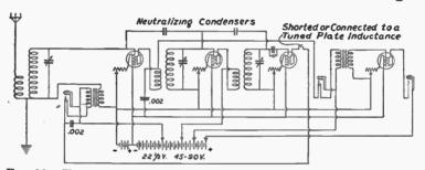
Fig. 92.—Hook-up for a three-tube reflex neutrodyne receiver with an additional stage of audio-frequency amplification and jacks.
