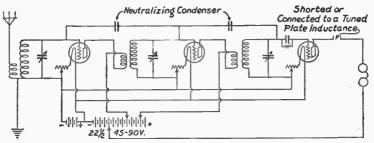
Fig. 90.—Hook-t? for a three-tube neutrodyne receiver.
