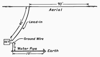
Fig. 4.—Method of calculating the physical length of an aerial circuit.
