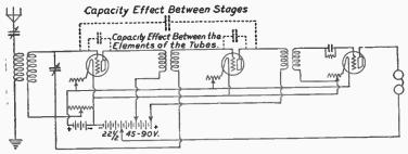
Fig. 89.—Graphic representation of the capacity effects which result from coupling together stages of radio-frequency amplification.
