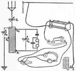
Fig. 40.—Hook-up for a three slide tuning coll in a crystal detector set.
