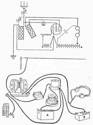
Fig. 64.—Hook-up for regenerative effect with two honeycomb colls.
