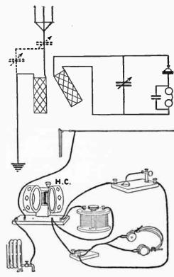
FIG. 43.—HOOK-UP FOR TWO HONEYCOMB COILS
