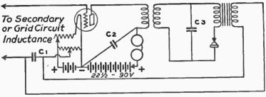
Fig. 85.—Hook-up for a one-tube reflex set with a crystal detector.
