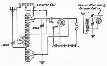
Fig. 74.—Hook-up for the Reinartz tuner with detector.
