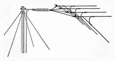
Fig. 8.—Aerial with metal spreaders requiring only a single insulator at each end. Note method of connecting the lead-in to the flat top. Note also eased off bends to reduce brush discharge in transmitting.
