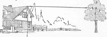
Fig. 11.—Complete installation of an inverted L single wire receiving aerial. Note connections of the lightning arrester and the lead-in. Note also method of suspending aerial with pulley, rope and weight, to avoid possibility of aerial breaking in a wind.
