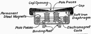
Fig. 20.—Cross section view showing the parts of a receiver. as the recording device of the transmitter is vibrating at the sending station; and these vibrations of the receiver diaphragm create the sound waves which strike the ear.
