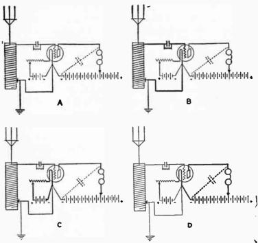
Fig. 49.—Four illustrations of the hook-up shown in Fig. 48. A shows the aerial circuit in heavy lines; 'B, the segondary or grid circuit in heavy lines; C, the filament circuit in heavy lines; and D, the plate circuit in heavy lines
