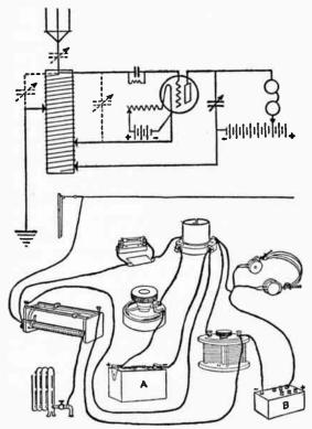
Fig. 60.—Hook-up for a three-slide tuning coll in a regenerative set.
