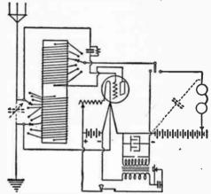
Fig. 104.—Use of a spark coll to increase the power of the receiver type of transmitter.
