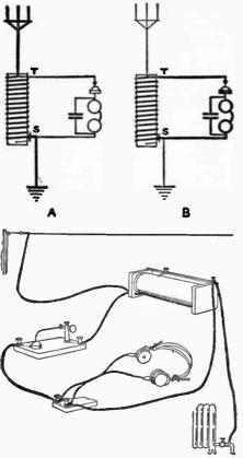
Fig. 21.—Circuits of the crystal detector hook-up. A. Primary in heavy lines. B. Secondary in heavy lines.
