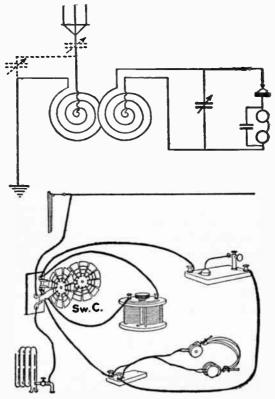
Fig. 44.—Hook-up for a crystal detector set with two spiderweb colls.
