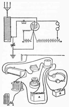
Fig. 58.—Hook-up for a single slide tuning coll in a regenerative set.
