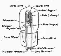
Fig. 47.—The three element vacuum tube.
