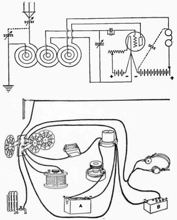
Fig. 66.—Hook-up for three spiderwes coils in a regenerative set. a third condenser may be used in the tickler circuit, as suggested for the preceding hook-ups.
