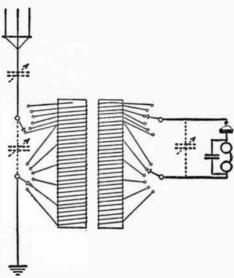
teur, if possible, in Fig. 39.—Hook-up for a loose coupler order to ascertain with four switches, in a crystal detector for set.
