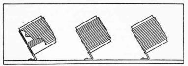
Fig. 91.—Diagram indicating how coils in a neutrodyne receiver are inclined in order to reduce inductive coupling, with the first coil cut away to show the position of the primary winding.
