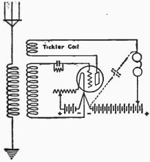
Fig. 56.—Hook-up for a regenerative set using a loose coupler with a tickler coll.
