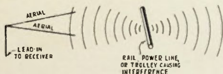
Fig. 87—A horizontal "V" antenna erected at right angles to an interfering power line, trolley line, etc., will help to reduce interference caused by direct induction. The lead-in is taken from the "V" end, as shown.
