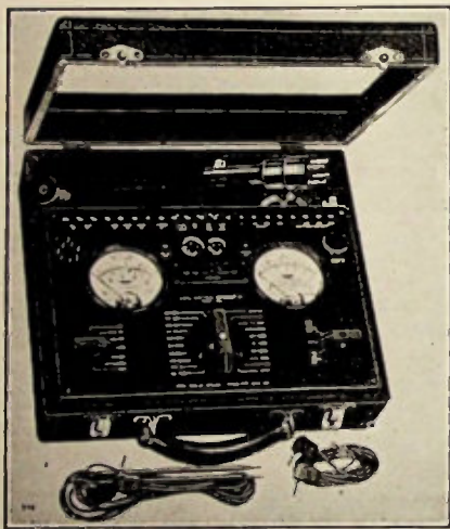
Fig. 32—A typical set analyzer employing two meters, a main selector switch at the center, and two switches at the sides. The cable and adapters are in the compartment at the rear. (Pattern 444.) See Fig. 33 for the circuit diagram.
