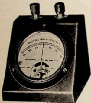
Fig. 5—A modern D.C. galvanometer or milliammeter built in portable form. This employs the Weston movement shown in detail in Fig. 4. This particular instrument is mounted on a type of portable mounting base, which is very convenient in laboratory work.
