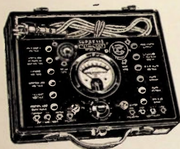
Fig. 31—A typical radio set tester and analyzer arranged in a portable carrying case. A single copper-oxide type meter, with a specially designed switching arrangement performs all the necessary tests. The dummy plug and cable are in the compartment at the rear. The circuit diagram is shown in Fig. 31A. (Supreme Model 90.)
