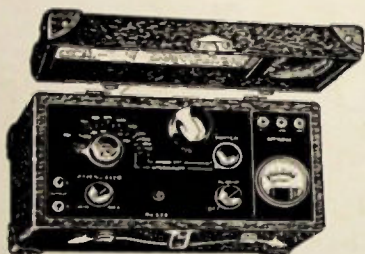
Fig. 67—A typical portable test oscillator with built-in output meter at the right. The schematic circuit diagram is shown in Fig. 66.
