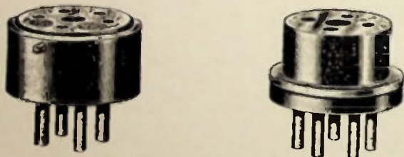
Fig. 36A—Typical adapters for use with set analyzers. The one at the left enables a 5-prong analyzer plug to be inserted into a 4-prong tube socket—the "cathode" terminal remaining unconnected. That on the right is for adapting a 4-prong plug to a 5-prong socket.
