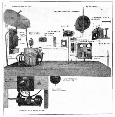
Fig. 39 .--- The Arc Transmitter.
