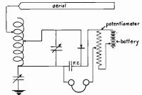
Fig. 59.—Conductively Coupled Receiver with a Crystal Detector and Potentiometer.
