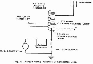
absorbs when operating. When the key is depressed, two auxiliary contacts in series with the resistance are opened, causing a momentary arc to be formed, which is blown between the copper and carbon electrodes. This ignites the arc and oscillations are produced as olng as the key is depressed. As soon as the signalling key is up, the arc is again shunted by the resistance.
