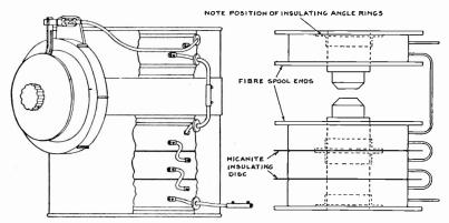
Fig. 48 .--- Views of Arc Chamber.
