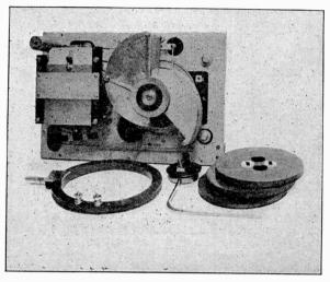
Fig. 9.—Kolster Decremeter and Wavemeter (Interlor View. (Courtesy of the Bureau of Standards.)
