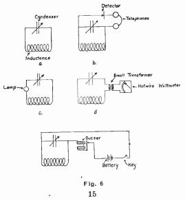
The calibration of the wave meter may be reduced in two ways—either by engraving the wave lengths of the meter for different condenser settings directly on the condenser scale or a curve of the wave lengths for different readings of the condenser in degrees may be plotted and drawn.
