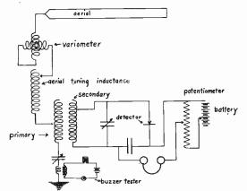
Fig. 60 .- Inductively (or Magnetically) Coupled Receiver.
