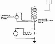
Fig. 43.-Connection of Chopper Commutator.
