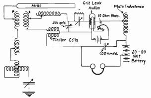
Fig. 72.-Wiring Diagram for a Regenerative Audion Hook-up.
