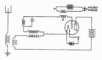
Fig. 55-B.—Diagram of simple microphone transmitter.
