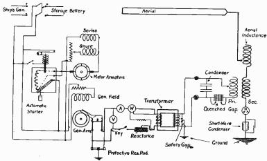
Fig. 11.-Fundamental Circuit Diagram of Transmitter.
