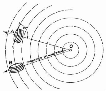
Fig. 73.—Showing Coll in Two Positions Relative to Field of Transmitting Antenna. (Courtesy of Robinson's Manual of Radio Telegraphy.)
