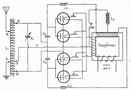
Fig. 54.—A Self-rectifying C. W. Tube Transmitter Operated on 60 Cycle A. C. (By Courtesy of the Q. S. T. Magazine.)
