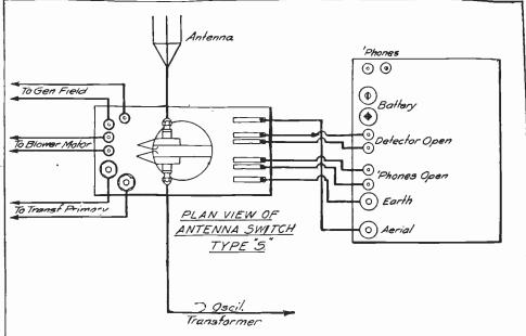
Fig. 36 .- Connections of Type "\$" Antenna Switch.
