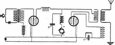
Fig. 55.—Modulating Circuit for a Radiophone Transmitter. (Courtesy of the Wireless Age.)
