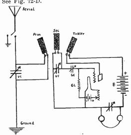
Fig. 72-D.—DeForest honeycomb coil type of receiver.
