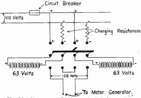
Fig. 76.-Charge and Discharge Switch Connections.
