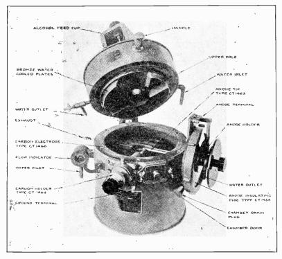
Fig. 46 .- View of Interior of an Arc Chamber.
