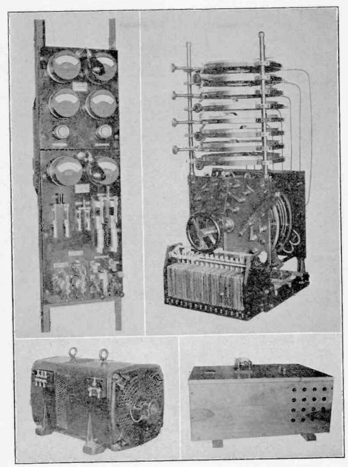
Fig. 10.-1/2 K. W. Transmitter with Motor Generator and Transformer at the Bottom.
