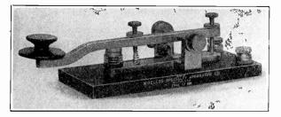
Fig. 26.—Wireless Telegraph Key.
