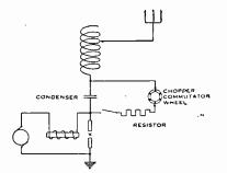
Fig. 44.—Connection of Chopper Commutator and Resistor.
