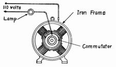
Fig. 25.-Test for Grounded Coil.
