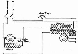
Fig. 17.—Motor Generator with Compound Generator Field Windings.
