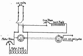
Fig. 16 .- Shunt Wound Motor and Shunt Generator.
