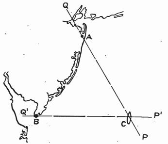
Fig. 75.—Method of Determining Absolute Direction and Location of Transmitting Station. (Courtesy of Robinson's Manuai of Radio Telegraphy.) Question 210. In the rotation through of a coil used for direction finding purposes, what takes place?
