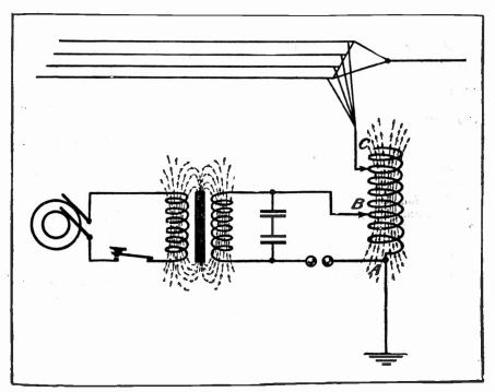
Fig. 28.—Conductively Coupled Transmitter.
