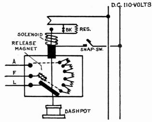
Fig. 19.-Cutler Hammer Automatic Motor Starter.
