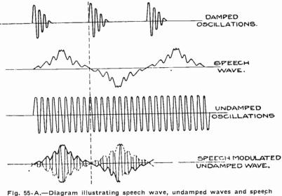
Fig. 55-A.—Diagram illustrating speech wave, undamped waves and spe modulation.
