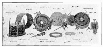
Fig. 47.—Exploded View of Arc Transmitter.
