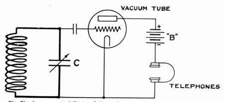
Fig. 74.—Arrangement of Tuning Coil and Detector. (The A or Filament Battery is Omitted Here. See Figure 66 for These Connections.) (Courtesy of Robinson's Manual of Radio Telegraphy.)
