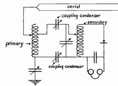
Fig. 61 .--- Statically (or Capacity) Coupled Receiver
