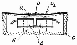
Fig. 65.—Constructive Features of a Telephone Receiver.
