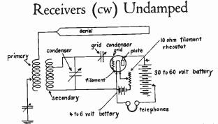
Fig. 66.—Receiving Circuit Diagram with an Audion Detector.
