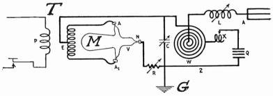
Fig. 38.-Simpson Impulse Transmitter.
