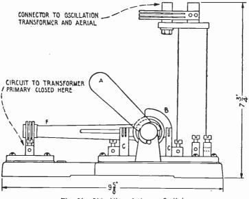
Fig. 34.—Side View Antenna Switch.
