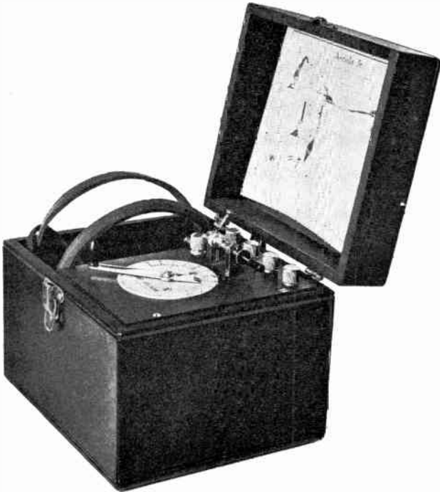
Plate IV.— Above: Crystal detector; Wireless Specialty Apparatus Company . Below: "Aeriola, Jr." crystal-detector receiving set; Westinghouse Electric & Manufacturing Co.
