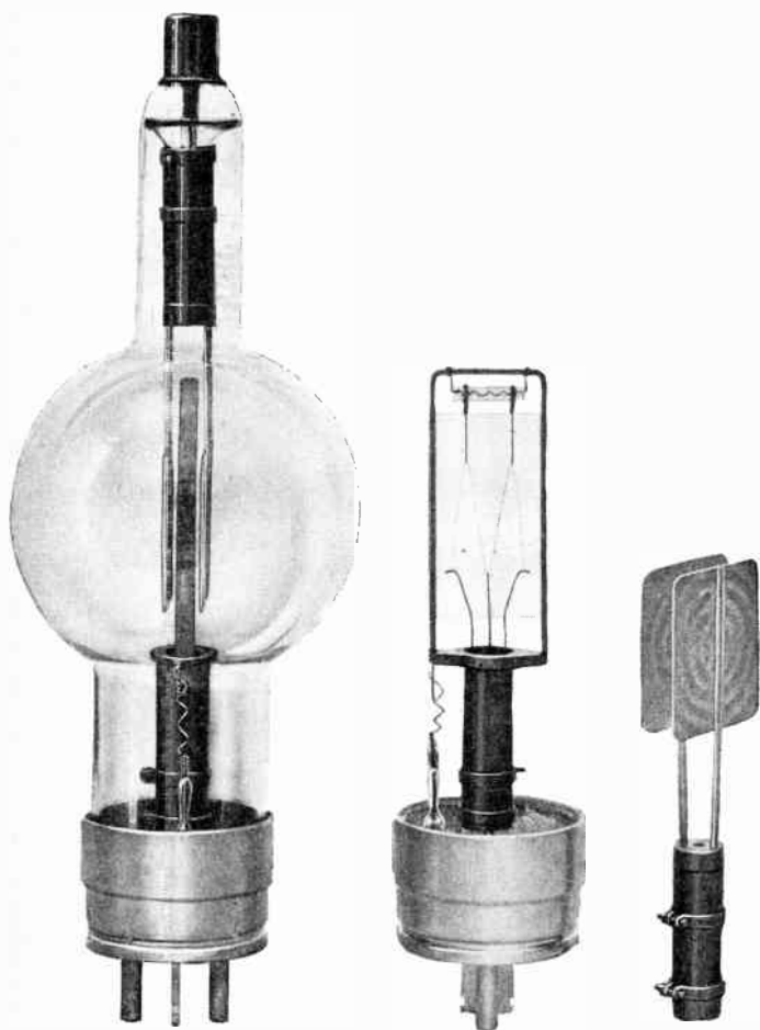
Plate XII.— Radiotron transmitting tube; Radio Corporation of America.
