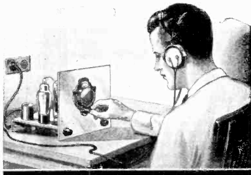
Regeneration control at lower right and large vernier tuning dial are main controls on this short wave set.
