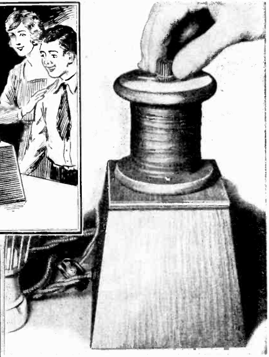
Fig. 2. Here is the completed electromagnet, set atop its mounting, with core inserted. With 110-volt current on, it is ready to perform a number of amusing stunts.
