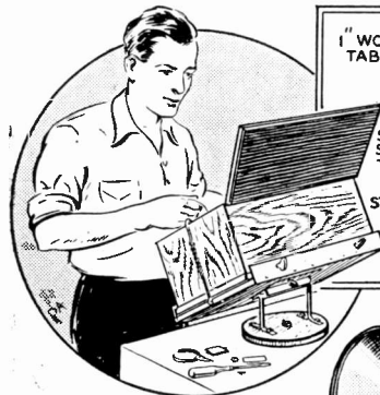
Adjustable radio set cradle shown above makes trouble-hunting easier, for set can be tilted or turned to any convenient position. Pad thumb-screws and metal side plate to prevent scratches on cabinet.
