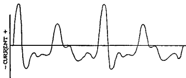
Fig. 188.—Wave Form for the Sound of “A” as in “Father”
