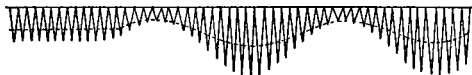
CONTINUOUS WAVES MODULATED AND RECTIFIED DOTTED LINE SHOWS AVERAGE CURRENT THROUGH TELEPHONE RECEIVER.
