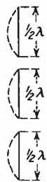
FIG. 313.—End view of arrays stacked one above the other and excited in phase.
