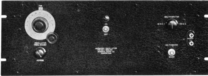
FIGURE 15. Panel view of the TYPE 618-A Harmonic Oscillator. The oscillator frequency is controlled by the dial and knob at the left; the multivibrator switch is at the right
