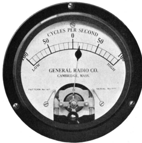
FIGURE 26. The indicating element of the General Radio frequency monitor for radio broadcasting stations
