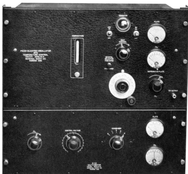
FIGURE 13. A photograph of the Class C-10 Standard-Frequency Assembly. This assembly is made up of a highly stable piezo-electric oscillator and a multivibrator
