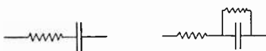
Fig. 96. At left, diagram showing a perfect condenser in series with a resistance; at right, showing how the actual resistance of a condenser may be in series or in parallel with a condenser.
