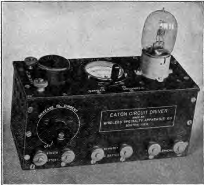
Fig. 24. —This Wireless Special Set Contains an Oscillating Circuit Which Can Be Connected to the Secondary.
