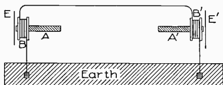
Fig. 77. Simplest Form of Electric Telephone.
