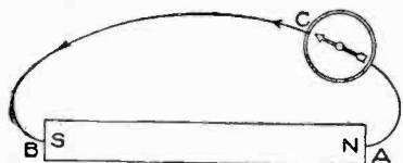
Fig. 7. Direction of Magnetic Lines of Force.
