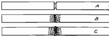
Fig. 12. Illustrating Action of Pieces in Electric Welding.
