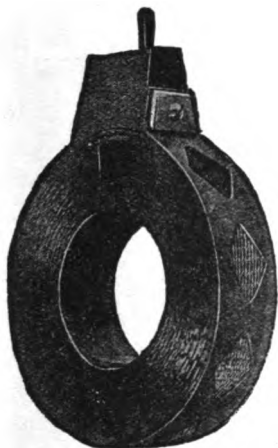
Fig. 18—Honeycomb Coils represent one of the most important recent advances in Experimental Work
