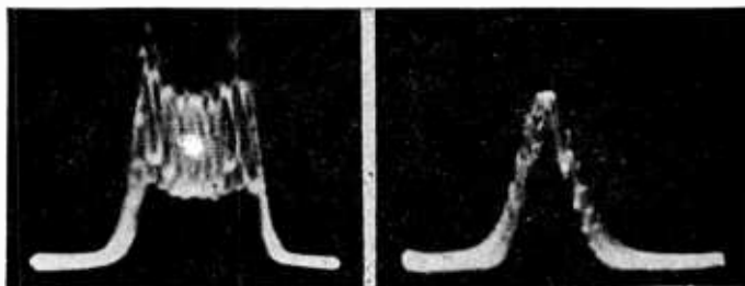
Figs. 293, left, 294, right. The output of the frequency modulated oscillator, used for making the resonance curve of Fig. 293, was also modulated at 400 cycles. The curve of Fig. 294 shows the presence of another carrier voltage that is beating against the frequency modulated signal, zero beat being at the mean frequency.
