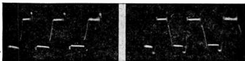
Figs. 370, left, 371, right. Similar oscillograms taken across S1 and the center tap and S2 and the center tap are shown in Figs. 370 and 371 respectively.
