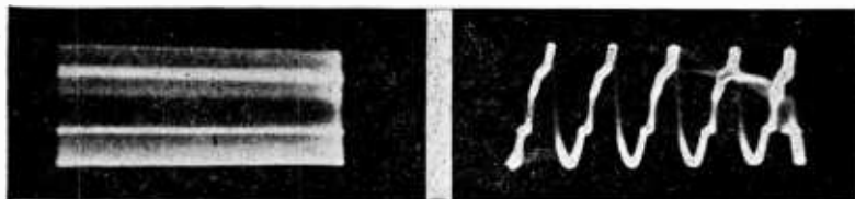
Figs. 225, left, 226, right. A 100-kc. unmodulated carrier was fed to the special amplifier of Fig. 224 and the streaked pattern of Fig. 225 was obtained. These light and dark horizontal lines in the pattern indicate that harmonics are present in the output of the oscillator. In Fig. 226 several cycles of this output wave are shown and the irregularities of the wave can be seen to correspond with the streaks in the pattern of Fig. 225.
