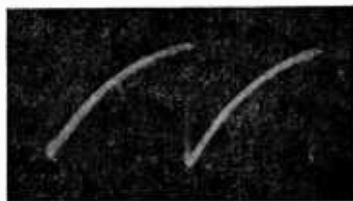
Fig. 31. Two cycles of the voltage wave taken across the output terminals of Fig. 30. The charging portion of the cycle is the sloping line and the vertical line is the discharge from maximum voltage to zero.
