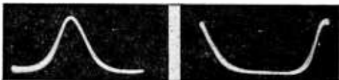
Figs. 316, left, 317, right. Curves showing correct and incorrect polarity of impulse generator signal appear at left and right.
