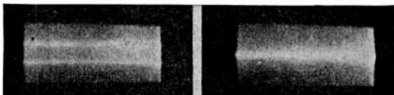
Figs. 384, left, 384-A, right. Two block patterns are here shown. That of Fig. 384 has fifty percent. modulation and that of Fig. 384-A is modulated one hundred percent.
