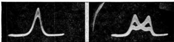
Figs. 291, left, 292, right. Both the resonance curves shown here have their lines broad because of the presence of an appreciable amount of carrier voltage.
