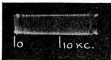
Fig. 337. An oscillogram of the output of the a-f. frequency modulator. Note that it is linear over the band from 0 to 10 kc.
