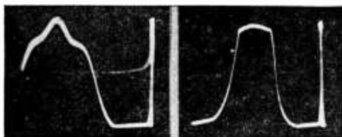
Figs. 318, left, 319, right. When the frequency modulator setting was incorrect, the curve of Fig. 318 was obtained. Overloading of the tubes in the resonated amplifier under test, caused the distortion in Fig. 319.
