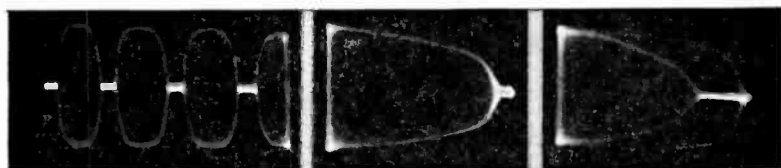
The wave envelope and trapezoid patterns are shown in Figs. 398 (left) and 399 (middle). Fig. 400 (right) shows the type of trapezoid pattern secured when the audio voltage for the horizontal displacement is secured from the input to the speech amplifier, instead of from the modulator, as in Fig. 399.
