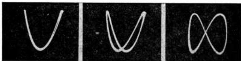
Fig. 96. A, left, B, middle, C, right. Lissajous figures showing a 2-1 ratio.
