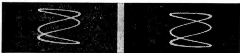
Fig. 97. C, left, D, right. 3-1 ratio patterns obtained by using two different phase relationships.
