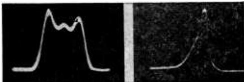
Figs. 284, left, 285, right. Two oscillograms of asymmetrical resonance curves. The lack of symmetry in the curve of Fig. 285 was caused by regeneration.
