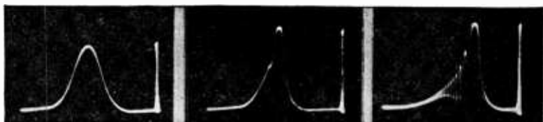
Figs. 320, left, 321, middle, 322, right. A correct resonance curve for a single-peaked system with minimum regeneration is shown in Fig. 320. An increase in regeneration caused the curve to become asymmetrical, see Fig. 321. Actual generation of oscillations is indicated in Fig. 322.
