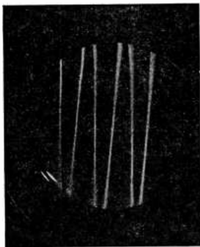
Fig. 85. The same wave as was shown in Figs. 83 and 84 is illustrated at the right. When this photograph was made the vertical amplitude voltage was increased so that the peaks of the wave were entirely off the screen, and the pattern is useless for observation of the shape of the wave.
