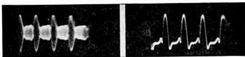
Fig. 235-A, left, Fig. 235-B, right. A. The modulated output waveform of the same oscillator used for generating waves shown in Fig. 234. The frequency here is 600 kc. B. The a-f. signal resulting from demodulation of A.
