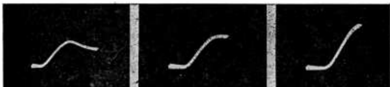
Fig. 129, left, Fig. 130, middle, Fig. 131, right. Grid voltage-plate current characteristics made by varying filament current and holding grid and plate voltages constant. Fig. 129 was made with the filament current too low. Note the lengthened curve of Fig. 130 caused by increasing the filament current. Fig. 131 shows the characteristic when the filament current was increased beyond its rated value.
