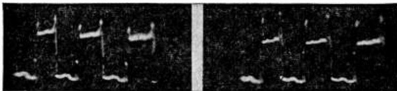
Figs. 365, left, 366, right. Resistance was added into the "A" contact circuit of Fig. 353. Fig. 365 was made with 1 ohm in the circuit and Fig. 366 with 2 ohms.
