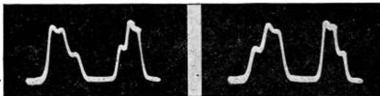
Fig. 266, left, Fig. 267, right. These oscillograms are examples of asymmetrical resonance curves, like those which were developed in Figs. 263 and 264. The differences between these curves are explained in the text.
