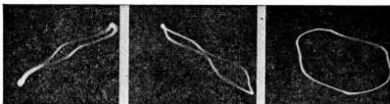
Fig. 95. E, left, F, middle, G, right. The three Lissajous figures here shown indicate a 1-1 ratio. One of the voltages impressed on the plates was not a pure sine wave; hence the distortion.
