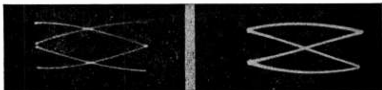
Fig. 77. The sweep frequency is four times the signal's frequency in both patterns. While these two patterns are useless for studying the character of the waveform, they can be used for frequency calibration.
