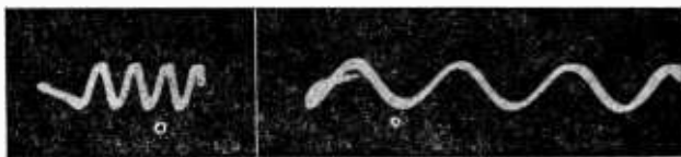
Fig. 86, left, Fig. 87, right. The same wave is shown in both illustrations with the same vertical deflection voltage applied. The horizontal deflection voltage has been increased in Fig. 87, so that the wave appears to be much flatter.
