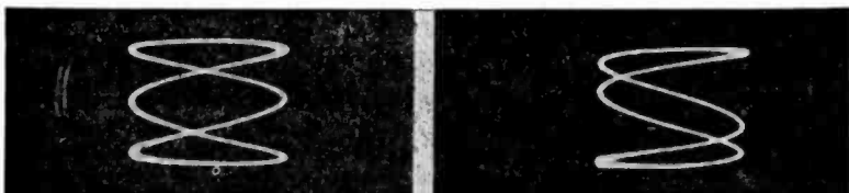
Fig. 97. E, left, F, right. The 3-1 pattern in E was photographed with a phase difference between the waves of 90^\circ , and that of F above 90^\circ .
