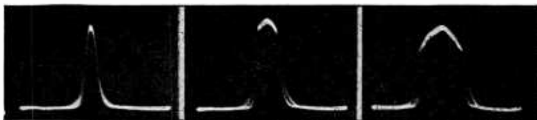
Figs. 296, left, 297, middle, 298, right. The resonance curve in Fig. 296 was made when the frequency modulated signal input to the circuit under test was the correct strength. The distortion in Fig. 297 was due to too strong a signal with resultant overloading of the tubes. Compare the spreading of the curve, indicating change in resonance when the signal is increased still further, as shown in Fig. 298.
