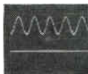
AT PLUG P1 P1 #9-(UPPER) LEFT OUTPUT 0.57V P/P (0.5 MILLISEC.) P1 #8-(LOWER) RIGHT OUTPUT 0.85V P/P (0.5 MILLISEC.)
