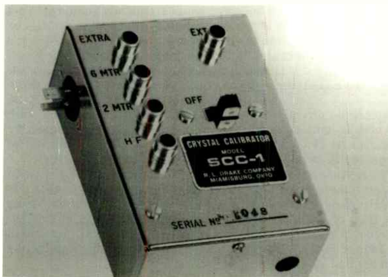
Fig. 4-8. This wide-range calibrator provides markers at 50-kHz intervals up to and including the high VHF band. (Courtesy R. L. Drake Co.)
