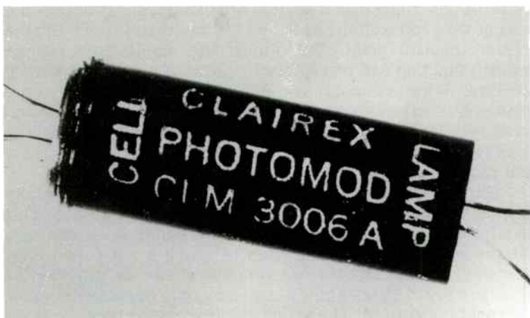
Fig. 4-3. Typical lamp-photocell module suitable for remoting a potentiometer. The module is about 1\frac{1}{4} inches long and \frac{3}{8} -inch in diameter.
