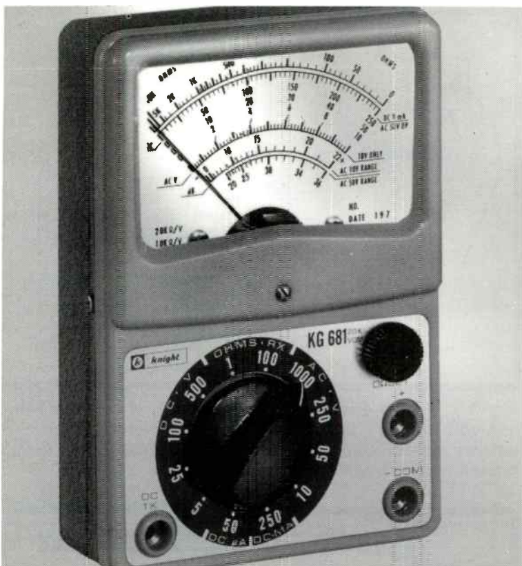
Fig. 1-5. A typical, simple volt-ohmmeter, such as this one, costs from $8 to $10.
