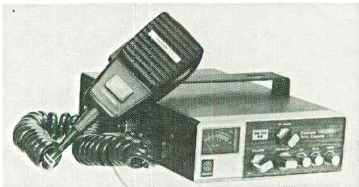
Fig. 4-3. Fanon Fanfare 190 DF CB set which uses the Resdel REC86345 PLL IC in its PLL synthesizer.
