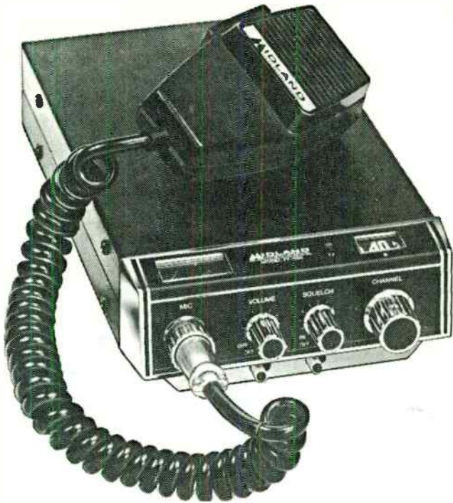
Fig. 5-4. The Midland 77-830 CB radio (courtesy of Midland International Corp.).
