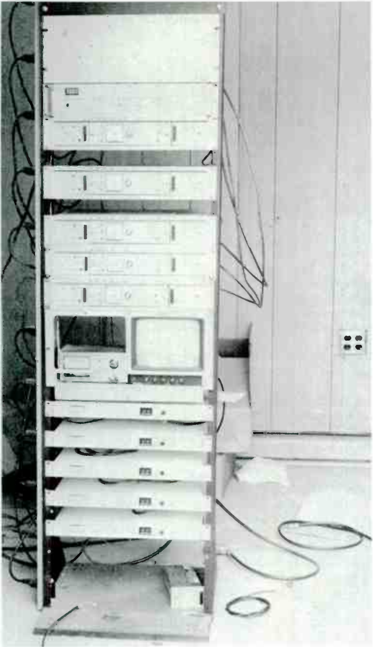
Fig. 11-3. The instrumentation rack contains receivers, modulators, monitors, and amplifiers.
