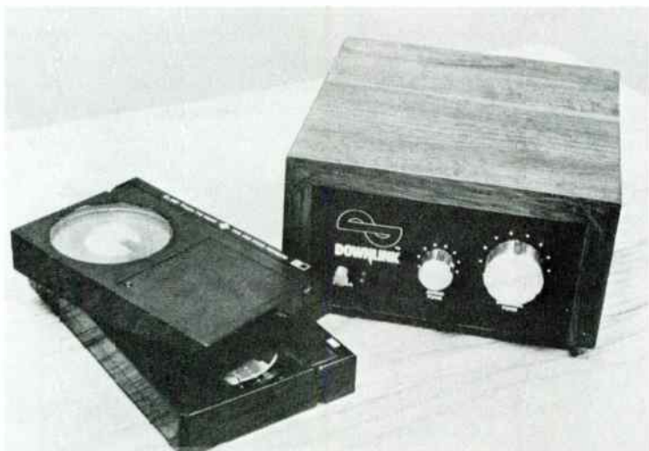
Fig. 7-17. Shown here is the receiver section with the remote console (courtesy Downlink, Inc.).
