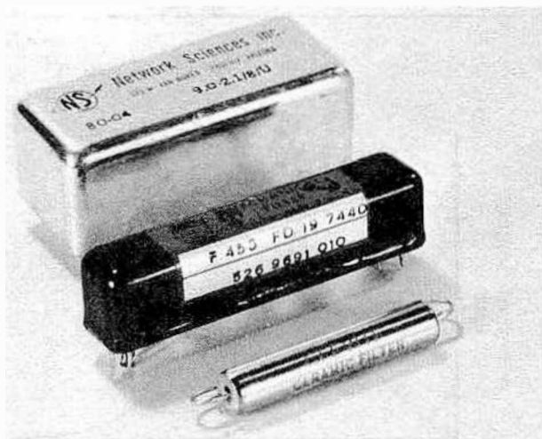
Fig. 4-26. Three types of modern i-f filters: Crystal lattice (top), mechanical (center), and ceramic (bottom).
