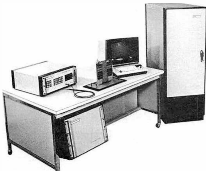
Fig. 23-1. Diagnostic computer used for automatic testing of module-boards.
