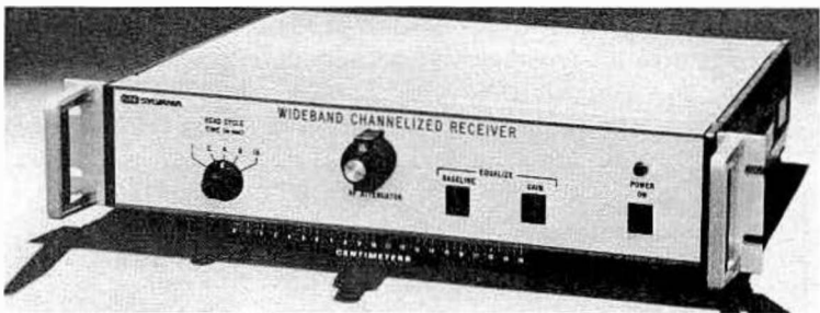
Fig. 25-3. A Bragg-Cell receiver developed by GTE-Sylvania (courtesy of GTE-Sylvania).
