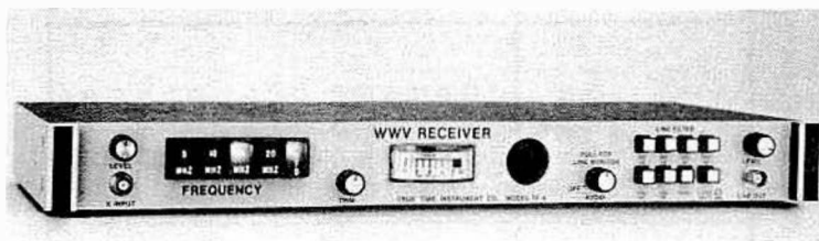
Fig. 11-1. This dedicated receiver is intended for WWV reception on one of the four selected frequencies. Automatic scanning of the receiving frequencies allows the unit to determine which frequency has the most usable signal and locks onto it. Careful system design shows that a double-conversion approach was used having the first i-f at 45 MHz followed by a second i-f at 4.6 MHz (courtesy of Kinemetrics, Inc. True Time Division).
