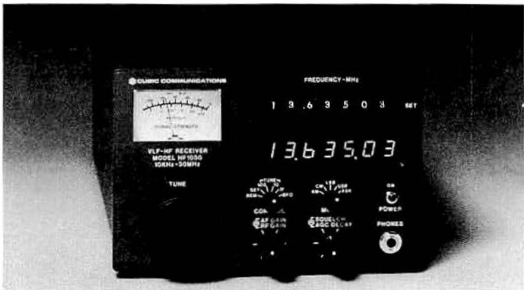
Fig. 18-5. Model HF-1030 general coverage communications receiver features a fast switching synthesizer (25 msec switching/settling speed) with a resolution of 10 Hz. The intercept point is +20 dBm (courtesy of Cubic Communications).
