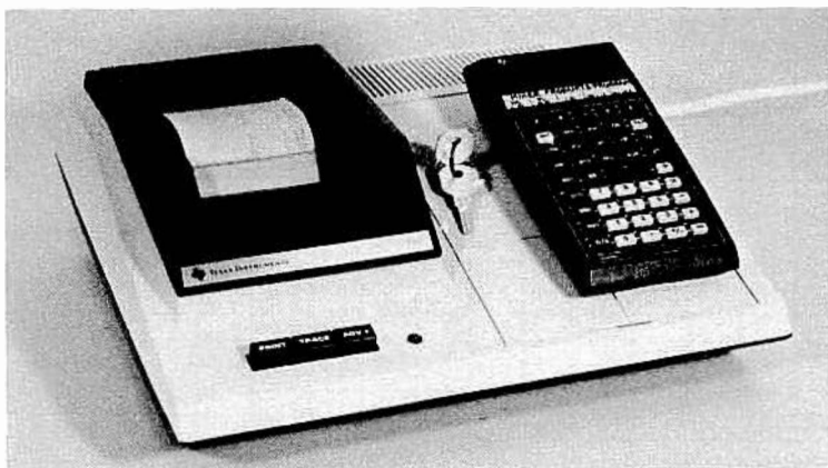
Fig. 11-8. The TI-59 programmable calculator and a PC-100 printer-plotter are used to analyze the intermodulation products that may exist in a radio receiver.
