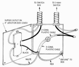
Fig. V-5. Connections at garage cable input. It includes a duplex outlet at the entrance junction box.
