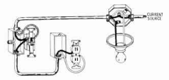
Fig. 4-7. Wiring system when the feed line comes into the ceiling fixture box. Note the three wires from the fixture to the switch. If the feed line comes into the outlet box, only two wires would be needed between switch and fixture.
