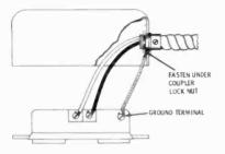
Fig. 3-6. On safety duplex outlets, the ground terminal is connected internally to the mounting ears. For added safety, connect a wire from the external ground terminal to a tight screw or nut on the outlet box.
