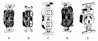
Fig. 2-10. Here are some of the various types of outlets. Most are double (duplex), since two fit the same box. A is the most commonly used duplex outlet. B is slotted to take some of the older plugs. Chas spring-loaded rotatable covers to keep children from poking metal objects into the terminals. D is for use with the three-prong safety plug, but also takes the standard two-prong plug. E is called a "crowfoot" outlet, for 240-volt wall outlets.
