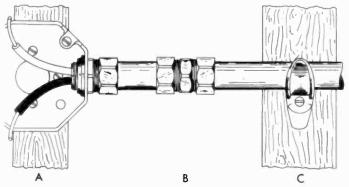
Fig. 4-5. Details of conduit installed in a junction box (A). Also shown is double-ended coupler (B) for splicing lengths of conduit, and bracket (C) for supporting long lengths.
