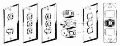
Fig. 2-9. A pilot light, a toggle switch and an outlet are available in what is called "interchangeable" devices. They may be used in any combination of two or three. They crimp to a special plate (shown at right) for mounting to an outlet box.
