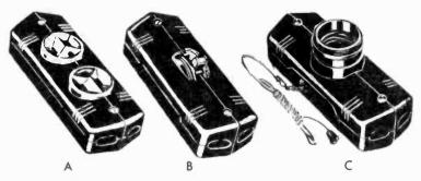
Fig. 2-13. Devices used for surface wiring where exposed wiring is not objectionable. They interconnect with plastic covered cable tacked in place. A is a duplex outlet. B is a toggle switch, used with C, a light bulb outlet.
