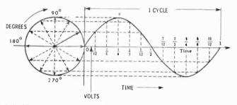
Fig. 1-4. Alternating current changes shown graphically. The curve is plotted against degrees of rotation (of a generator, for example) versus time. The speed of the generator produces 60 cycles per second. The curve is called a "sine wave."
