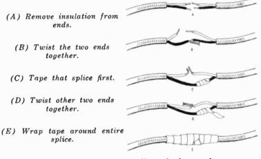
Fig. 3-3. It is easy to splice a broken cord.
