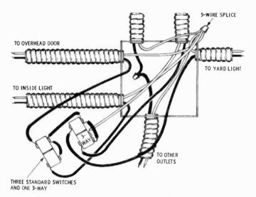
Fig. V-6. Distribution junction box with three-way switch plus three individual light switches.
