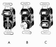
drive away. Another switch has a pushbar on the front; push once for "on," push again for "off." This type (Fig. 2-7B) takes the same front wall plate as the toggle switch.
