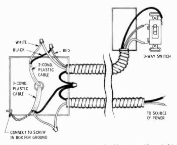
Fig. V-3. In-house wiring to underground cable to provide switching of lights from house to garage, plus separate power for outlets in garage.
