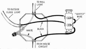
Fig. IV-5. Change a single switch to two switches: one for the original inside light, and the other for the new floodlight.
