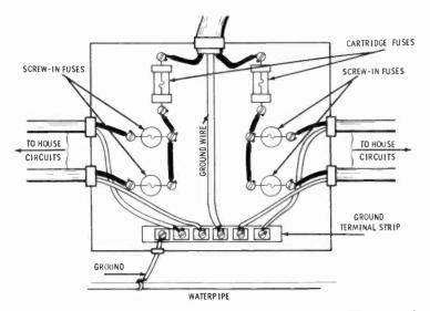
Fig. 1-6. A typical "60-ampere service" box, using fuses. The 240-volt service is brought into the top of the box by the power company. 60-ampere cartridge fuses protect the main incoming line. 15-ampere screw-in fuses protect the separate circuit branches against overload. Note that the "neutral" (colored white) lines are not fused.
