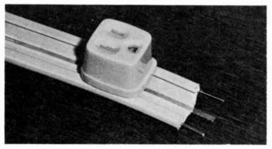
Fig. III-3. Detail of "Electrostrip" surface-wiring cable. Center ribbon is "ground" strip. Outlet twists into grooves and contacts currentcarrying wires and ground strip.
