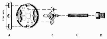
Fig. 2-17. Fittings used to hang fixtures from ceiling boxes. A is a strap for fixtures, that mount with two wide-spaced screws. B is a stud that screws to the box and accepts the nipple at C and is used on center-bolt mountings. D is an extension nipple.
