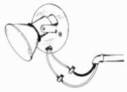
The box must have a black and a white wire coming into it for a source of power. Splice the white wire from the conduit you installed to the white wire in the box. The black lead from the conduit connects to one side of the new switch installed. The other terminal of the switch is "jumpered" to the terminal of the other switch to which the black wire already in the box is connected. Install the second switch to the same wires removed from the original switch (Fig. IV-5).
