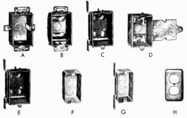
Fig. 2-4. Small boxes used to hold switches and outlets. A has pull-up side ears that hold the box to plasterboard and Sheetrock. B is fastened to the lathing in plaster walls with the top and bottom ears. Both of these boxes are for "old work." C, D, and E have brackets welded on for attaching to wall studs in "new work." F and G are for exposed mounting, such as at work benches; H is a metal cover for
