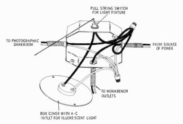
Fig. I-4. Wiring of junction box above workbench. This illustration shows couplers on the flexible armored cable. The switch is installed by drilling a hole of the proper size in one of the knockout forms.
