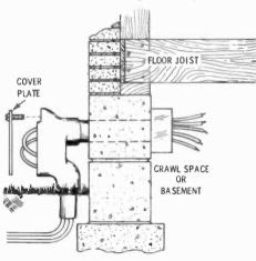
the vertical sections of the thin-wall conduit and out through the elbows. Make the bend at the bottom of the thin-wall sections as gradual as you can to prevent the edges of the conduit from cutting into the plastic. At the entrance elbows, bend the cable and push them through into the house at one end, and into the garage at the other end (Fig. V-2). Leave enough cable out the junction boxes to work with. Put the covers back on the elbows. Push the dirt back into the ditch and tamp it down.
