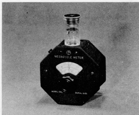
Fig. 10-12. Low-frequency oscillator head for the Megacycle Meter. Courtesy Measurements Div., McGraw-Edison Company.
