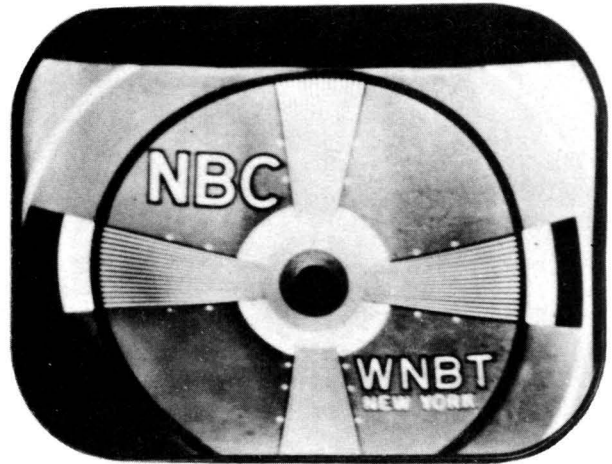
Fig. 117. Focus Coil and Ion Trap Misaligned
