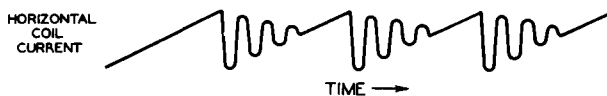
Fig. 74. Horizontal Deflection Coil Oscillation Which Would Occur If Damping Tube Were Not Used
