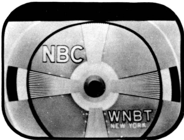
Fig. 129. Vertical Centering Control Mis-adjusted
