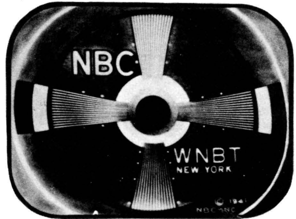
Fig. 242. Station Test Pattern Showing the Effect of Misadjustment of the Contrast Control. Photo Courtesy National Broadcasting Company and the R. C. A. Service Company, Inc.
