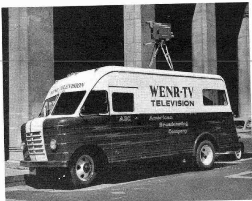
Fig. 7. Typical Remote Pickup Unit. (Photo Courtesy WENR)
