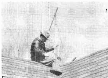
Fig. 73. Portable Receiver Used to Determine Orientation of the Antenna.
