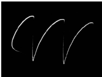
Fig. 4-9. Nonlinear sawtooth waveform.
