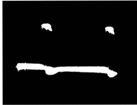
Fig. 5-6. Jitter in a 15,750-cps signal.
