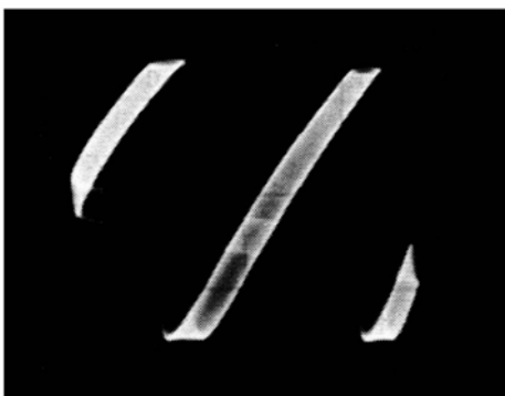
Fig. 5-14. Sawtooth pattern with 60-cycle hum.
