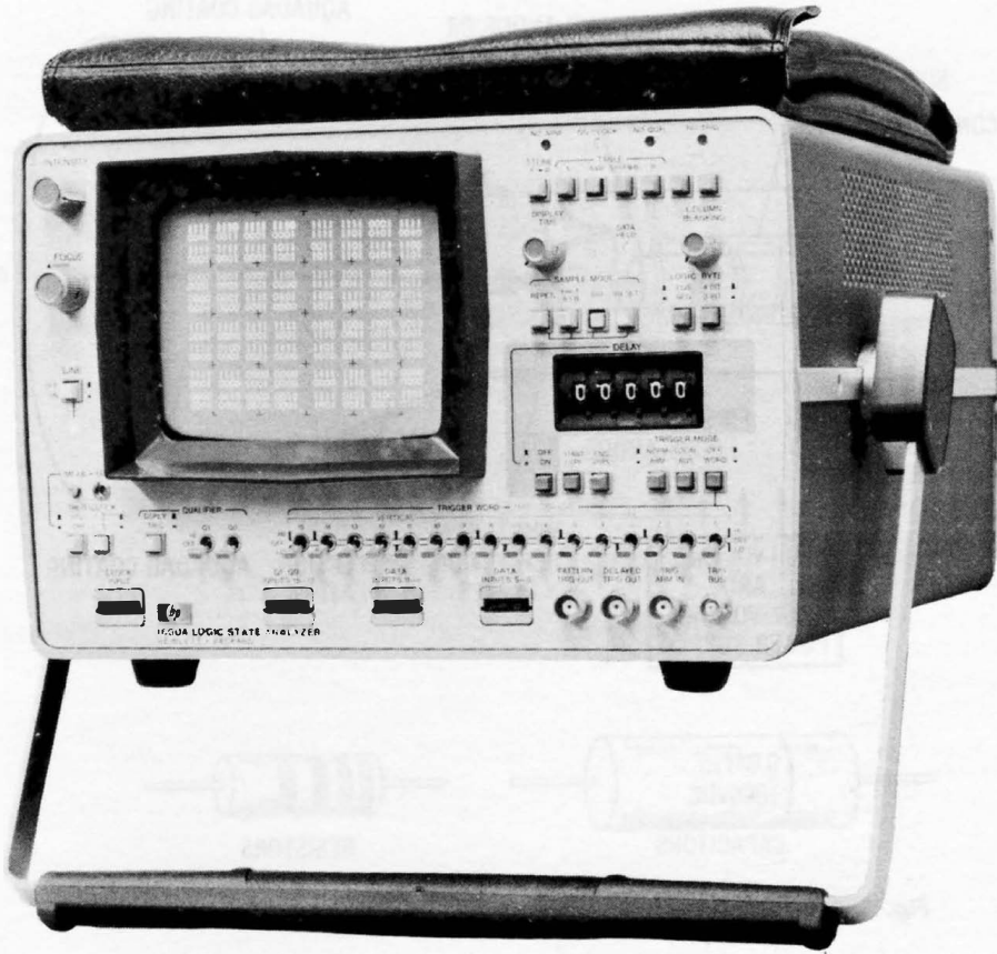
Fig. 1-2. A logic-state analyzer oscilloscope used as a data-domain display.
