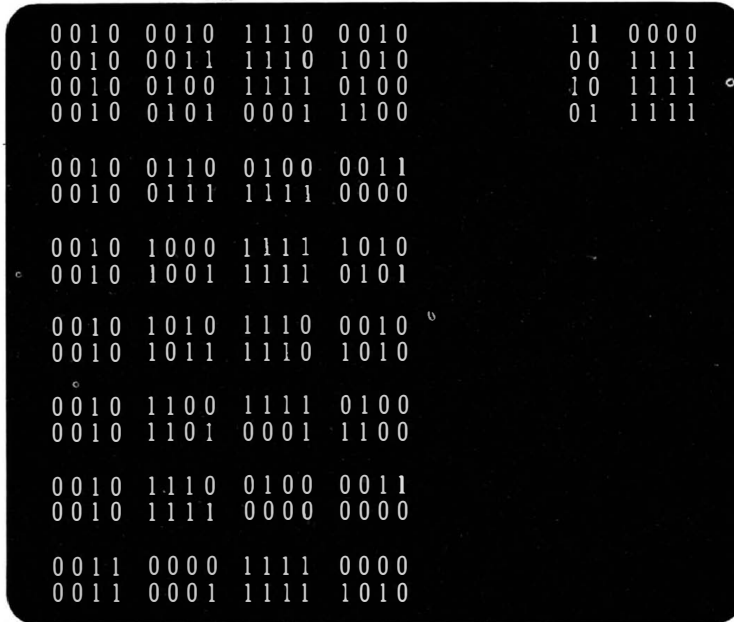
(B) Check of a dual-clock operation displayed on screen of a data-domain analyzer.
