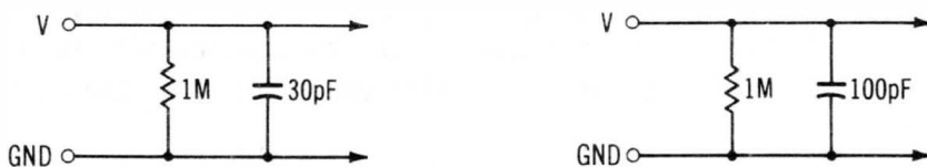
(A) Capacitance present at the vertical input terminal on the front panel. (B) Total input capacitance present due to use of a coaxial cable probe.
