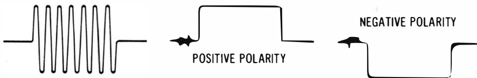
Fig. 6-12. Demodulated output waveform is “tuned upside down” if polarity of detector diode is reversed.
