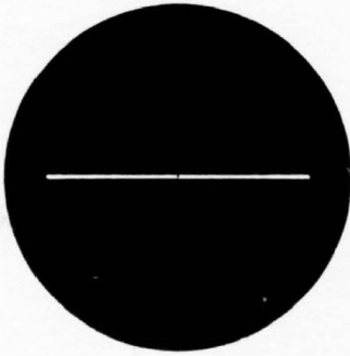
(A) Horizontal base line is displayed in absence of signal input.
