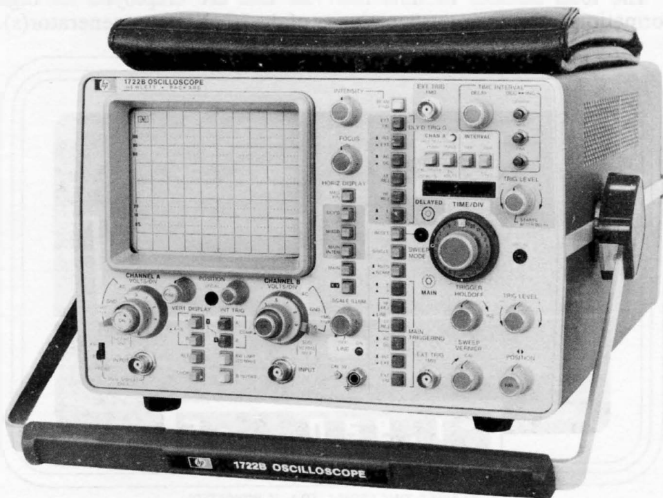
Fig. 1-10. Parallax error is avoided in this oscilloscope by having the graticule ruled on the inside surface of the crt.
