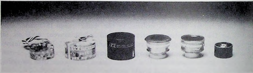
Fig. 9.10 Generation 2 and 3 image intensifier components.
