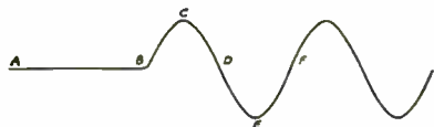
Fig. 63. From A to B, no modulating voltage exists. At B the 400-cycle voltage starts and the points C, D, E, and F show peak and zero voltages.
