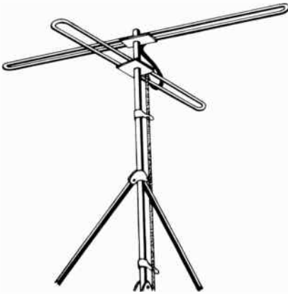
Fig. 4-2. Fm antenna with two folded dipoles.
