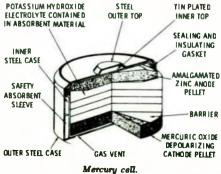
anode and a mercuric-oxide cathode in a potassium-hydroxide electrolyte. This cell offers a higher capacity than the alkaline or zinc-carbon cells and a much flatter voltage-discharge characteristic.
