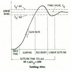
from the initial value to within a specified window around the final value in response to a voltage or current step on the tuning input port.
