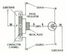
Insulated gate field-effect transistor.
