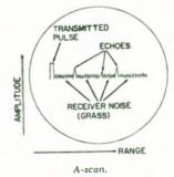
A-scan-Also called A-display. On a cathode-ray indicator, a presentation in which time (range or distance) is one co-ordinate (horizontal) and signals appear as perpendicular deflections to the time scale (vertical).
