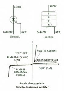
are anode cathode and gate. 4. A silicon rectifier having a pnpn structure that blocks current in both directions unless it is triggered into forward conduction by a pulse applied to its gate electrode. The rectifier stops conducting only if the forward current falls below the holding current.
