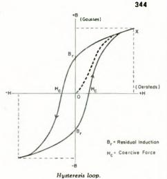
induction; one when the magnetizing force is increasing, the other when it is decreasing.
