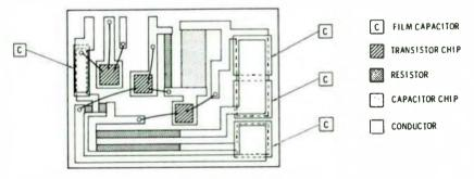
Thick-film hybrid integrated circuit.
