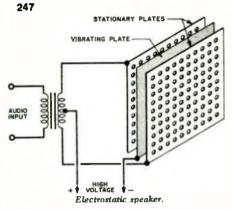
the mechanical forces are produced by the action of electrostatic fields.
