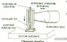
ultrasonic brazing-See Ultrasonic Soldering.
