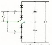
VOLTS D.C -4X PEAK VOLTS A'C Voltage quadrupler.
