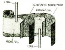
Capacitor (internal construction).
