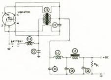
Synchronous-vibrator power supply.
