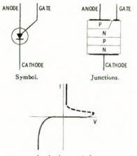
Anode characteristic. Complementary silicon controlled rectifier.
