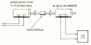
DC VOLTMETER (WITH DC TACHOMETER) OR FREQUENCY METER (WITH AC TACHOMETER) CALIBRATED IN RPM
