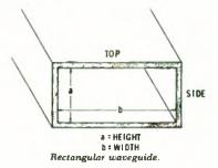
with the dimensions of the sides in a ratio of 2:1. With dimensions so proportioned, the dominant mode has a freespace wavelength range between one and two times the longer side dimension. Rectangular waveguide normally can be used only over less than octave ranges.
