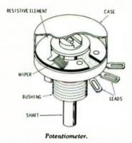
contact arm so that portion of the potential applied between its ends may be selected. 4. A variable voltage divider used for measuring an unknown electromotive force or potential difference by balancing it, in whole or in part, by a known potential difference. 5. An instrument used to measure or compare voltages.
