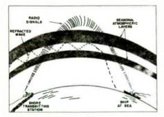
Refraction (of radio waves).
