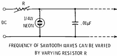
FREQUENCY OF SAWTOOTH WAVES CAN BE VARIED BY VARYING RESISTOR R
