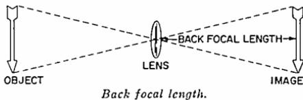
**back focal length**—Distance from the center of a lens to its principal focus on the side of the lens away from the object.
