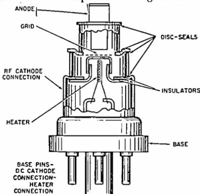
*Cutaway view of lighthouse tube.*
