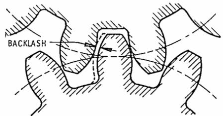
**backlash**—1. In a potentiometer, the maximum difference that occurs in shaft position when the shaft is moved to the same actual output-ratio point from opposite directions. Resolution and contact-width effects must be excluded from this measure. 2. The shortest distance between nondriving tooth surfaces of adjacent teeth in mating gears or the amount of clearance between the teeth of mating gears. Usually measured at the common pitch circle.
