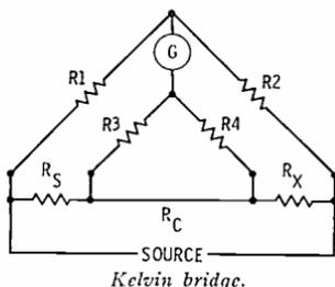
**Kelvin bridge**—Also called a double or Thomson bridge. A seven-arm bridge for comparing the resistances of two 4-terminal resistors or networks. Their adjacent potential terminals are spanned by a pair of auxiliary resistance arms of known ratio, and they are connected in series by a conductor joining their adjacent current terminals.
