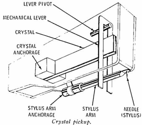
**crystal pickup**—Also called piezoelectric pickup. A phonograph pickup which depends for its operation on the generation of an electric charge by the deformation of a body (usually crystalline) having piezoelectric properties.
