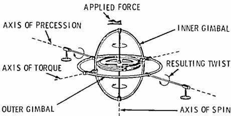
*Precession of a gyroscope.*
