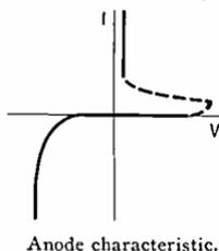
Anode characteristic. Complementary silicon controlled rectifier.
