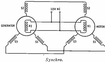
**synchro**—A small motorlike device containing a stator and a rotor and capable of transforming an angular-position input into an electrical output or an electrical input into an angular output. When several synchros are correctly connected together, all rotors will line up at the same angle of rotation.
