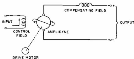
**amplidyne**—A special direct-current generator used extensively in servo systems as a power amplifier. The response of its output voltage to changes in field excitation is very rapid, and its amplification factor is high.
