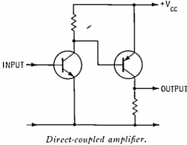
**direct-coupled transistor logic**—A NOR-gate type of bipolar logic in which the output of one gate is coupled directly to the input of the succeeding gate. This form of logic evolved into resistor-transistor logic because of the difficulty in mass producing transistors within the close tolerances necessary for direct coupling. Abbreviated DCTL.
