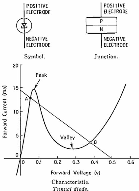
and a negative-resistance region above a minimum level of applied voltage. With the addition of suitable external circuits, it can be used as an oscillator or amplifier. Also called Esaki diode.
