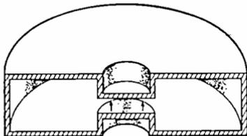
*X-band reflex-klystron resonant cavity.*
