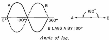
**angle of lag**—The angular phase difference between one sinusoidal function and a sec-
