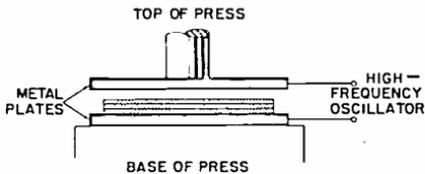
**dielectric heating**—A method of raising the temperature of a nominally insulating material by sandwiching it between two plates to which an rf voltage is applied. The material acts as a dielectric, and its internal losses cause it to heat up.
