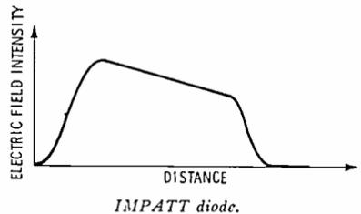
so constructed that the active region is very close to a good heat sink. For the same reason, the bias supply must be a constant-current type.
