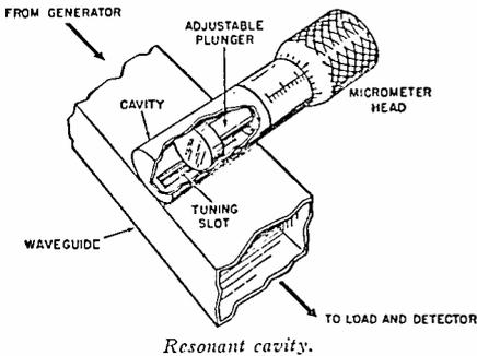
**resonant cavity**—A form of resonant circuit in which the current is distributed on the inner surface of an enclosed chamber. By making the chamber of the proper dimensions, it is possible to give the circuit a high  $Q$  at microwave frequencies. The resonant frequency can be changed by adjusting screws which protrude into the cavity, or by changing the shape of the cavity.
