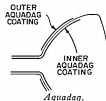
**aquadag**—A conductive graphite coating on the inner side walls of some cathode-ray tubes. It serves as an electrostatic shield or as a postdeflection and an accelerating anode. Also applied to outer walls and grounded; here it serves, with the inner coating, as a capacitor to filter the applied high voltage.
