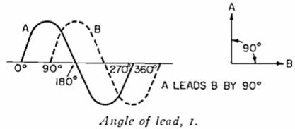
**angle of lead**—1. The time or angle by which one alternating electrical quantity leads another of the same cyclic period. 2. The angle through which the commutator brushes of a generator or motor must be moved from the normal position to prevent sparking.
