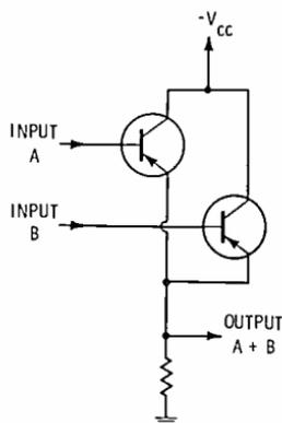
OR gate (using transistors).
