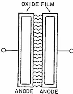
*Nonpolarized electrolytic capacitor.*
