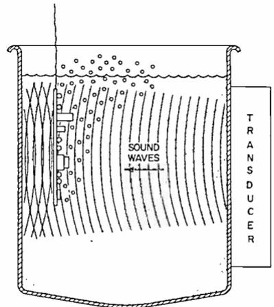
**ultrasonic cleaning tank**—A heavy-gage, polished stainless-steel tank with transducers mounted on the bottom or sides.
