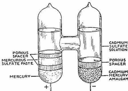
**standard cell**—A primary cell which serves as a standard of voltage.
