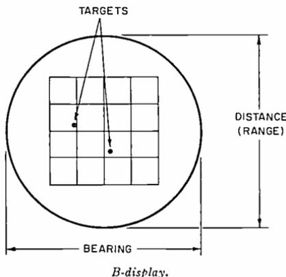
**B-display**—On a radarscope, a type of presentation in which the target appears as a bright spot. Its bearing is indicated by the horizontal coordinate and its range by the vertical coordinate.
