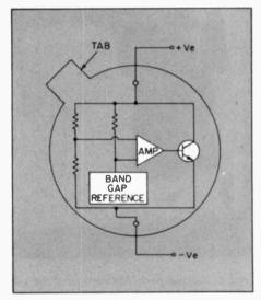
Here is an internal schematic of the band gap zener diode, which serves as the heart of the calibrator. Use the tab on the case as the reference point for making circuit connections. No heatsink is required here.
