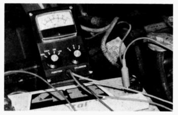
Here the Dwell/Tach's voltmeter function is being utilized to test a battery. If you look closely, you'll see that the meter is reading a nominal 12-volts.
