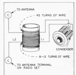
Cure the interference problems common to older, less sensitive receivers with this simple wave trap.
