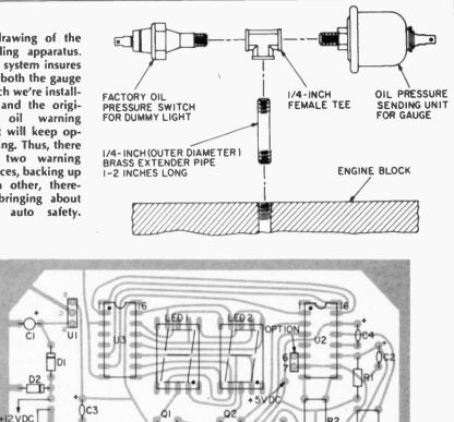
Parts layout for the Digital Oil Pressure gauge. There are relatively few components to worry about, those that there are, are relatively well-spaced. VCR's on other side.
