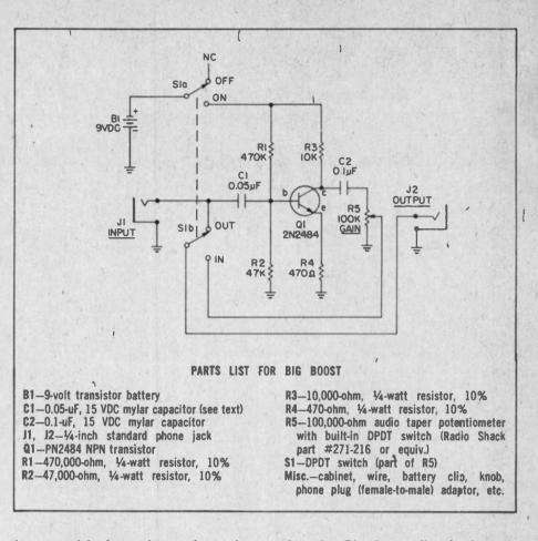
ing a special *phone plug-to-phone plug* adaptor sold at music instrument shops. You can use the adaptor for either the input or output. If desired, you can plug the Big Boost directly into an electric guitar or keyboard output jack, and then use a regular patch cord to the amplifier's input.
