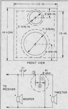
Crossover diagram for woofer and tweeter balancing. These components are included in the Speakerlab kit.
