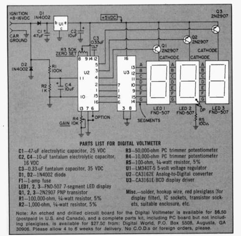
these chips (CA3162E and CA3161E) are aligned as shown on the diagram. Note the notch mark on the chips and the corresponding notch mark on the schematic, or the "1" on pin 1 on top of the plastic case. All manufacturers use one or both of these base reference directional indicators.
