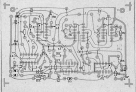
Printed circuit board for FasTouch. This is the exact size PC board that you'll need to build FasTouch. Remember, when doing PC boards, always use the foil side layout.
