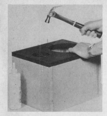
The inner speaker enclosure box must be assembled carefully. Make certain that all edges are square and flush.
