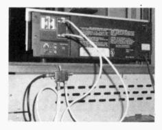
The DPDT switched splitter is attached to the main TV set. Note the wiring layout.
