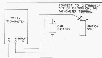
Fig. 6. This is the wiring setup utilized tor final calibration. A well-regulated 12-volt power supply is a necessity here. Alternatively, you can use the car's battery if it is fully charged.
