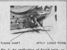
Fig. 2. An application of liquid rosin, usualy found in most TV repair supply shops will help to eradicate the dial cord slippage.
