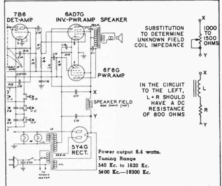
When you want to substitute a modern speaker for an old one that had a speaker field coil, you need to replace the lost impedance in the circuit. Unlike this schematic of a Zenith Model 75681/2 many old-time schematics don't always include the value of the coil. Determine this with the top circuit and replace it with the bottom one.
