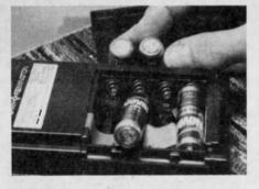
**Corroded Battery Terminals.** When batteries are left unused for a long period of time, they begin to leak and corrode around the battery terminals. Try to keep fresh batteries in the calculator to prevent corroded terminals. Replacement with leak-proof and long life batteries helps, but after a long
