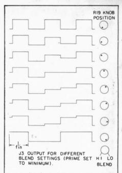
Here is the chart of the various waveform configurations made possible by varying settings on the "blend" and "prime" controls. Although designed for use through a three-octave range, if used with an electric guitar, false harmonics can be generated by forceful strumming, thus raising the outputs by one full octave automatically.
