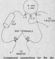
Component connections for the doit-yourself version of the crossover circuit. Pay close attention to speaker polarity when wiring this balancing unit.
