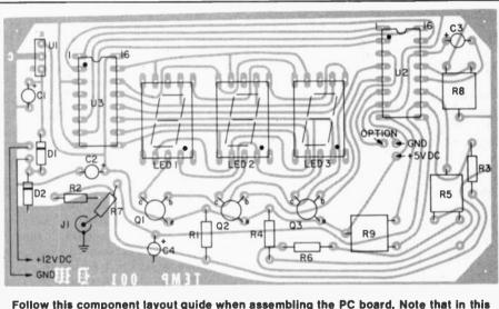
Follow this component layout guide when assembling the PC board. Note that in this diagram, U1 is installed on top of the board. Depending upon your space requirements, it can go on top or bottom, but be careful not to reverse the pin connections.
