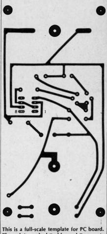
The points marked "solder pads" on parts layout need no holes etched or drilled.
