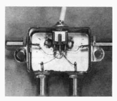
Line splitters are easily modified to take a switch. This switching ability is vital.
