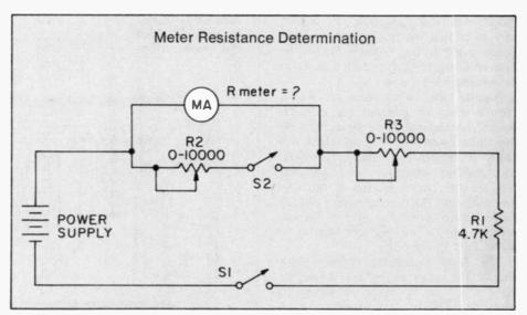
To determine the internal resistance of a meter construct a circuit like the one illustrated above. If you don't have the parts in your junk box then check an electronics surplus outlet.
