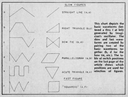
the same magnitude and frequency is fed to the other input. On the scope's screen there appears either an elliptical or circular trace, depending upon the 'phase relationship between the two signals. With non-sinusoidal waveforms driving the X and Y inputs, other geometrical displays can be created.
