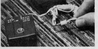
The most common fault with AC adapter jacks is defective contacts. If spraying with tuner cleaner doesn't help, you may have to replace either the jack or the plug that goes into it. Both of these repairs are easy to do.
