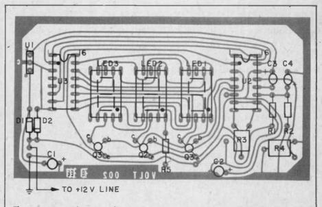
The component placement diagram for the PC board shows all IC and capacitor polarities. Take special care to observe them during assembly phases of project.
