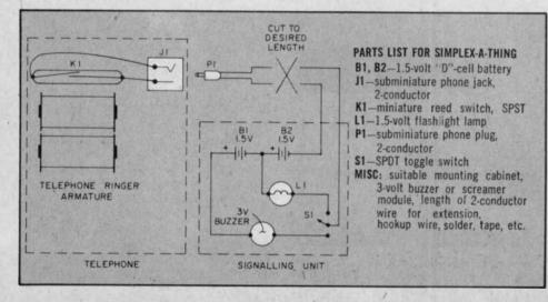
The switch is triggered even if you turn the regular telephone bell off to provide completely silent signalling by means of a blinker light.
