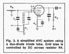
In the simplified circuit of fig. 4, the action of the AVC voltage is easier to understand. The voltage across R4 is applied to C3 through R3. These resistors have high values, typically a half to one megohm, so that with a given
