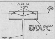
Fig. 6. A drop of plastic cement placed on the stops of the dial pointer will usually prevent the pointer from slipping around.
