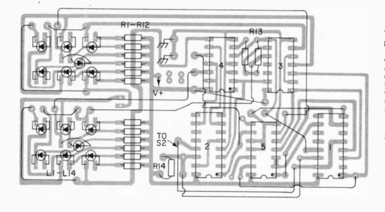
The parts overlay diagram shows the placement of components on the PC board. As in all projects using a number of delicate ICs care must be taken with the pins and with the use of soldering irons too near to the chips. Digi Dice is a project to gladden a gambler.
