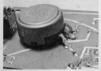
To prevent a shock hazard caused by the pins sticking up on the top side of the printed circuit board, R1's terminals are tack-soldered to the pads on the etched side of the board. A strong physical connection is assured by through-the-board mounting of R1's shaft. meter as you would for black and white printing—as we'll show you at the end of this article.
