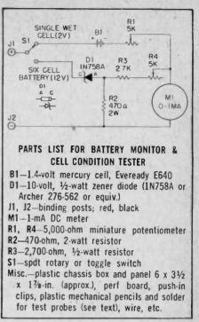
to cut out the M1 mounting hole in the panel and install the meter in approximately the same position shown in the panel photo. Then locate and mount S1, J1 and J2. Cut a section of perf board to size, and drill two holes to fit the M1 terminal screws to mount the board. Install the perf board to the meter terminals with two solder lugs supplied with the meter.
