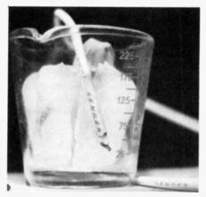
Use a setup like this for the low end calibration of the temperature gauge. See text.
