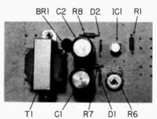
This is the parts location when our PC board is used. To get a free template of the PC board, send a Self-Addressed Stamped Envelope to BUDGET ELECTRONICS, Davis Publications, Color Analyzer, 380 Lexington Ave., New York, N.Y. 10017.
