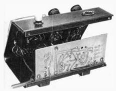
Rear view of author's color analyzer shows vertical mounting of the circuit hoard.
