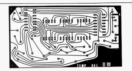
Here is the full-scale etching template for the printed circuit board. See the parts tist for ordering information on a ready-to-go board if you don't etch your own.
