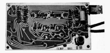
The foil side of the completed board shows U1 mounted from the underside. If pins are reversed, U2 and U3 will be ruined.
