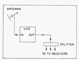
Shown here in its simplest form, this VCR system carries signal from the antenna, to the VCR itself, and then to the various TVs.
