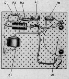
Perf board showing components including location of meter as dashed line. Mercury cell battery will last its shelf life, which is generally two years for a fresh battery. Eliminate D1, R2, R3, R4, and S1 for a dunk-test only meter. 2-V is center scale.
