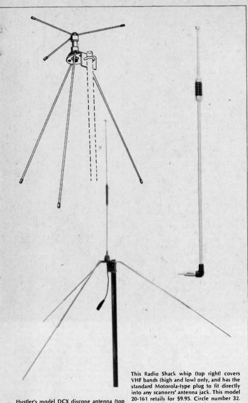
Hustler's model DCX discone antenna (top left) is an excellent, wide-range utility unit for continuous coverage from 40 to 700 MHz with no retuning necessary. Circle number 49 on the reader service coupon.
