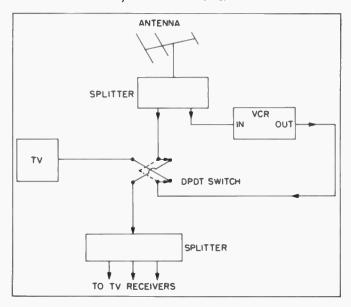
This is a diagram of a fancy home VCR system. It feeds up to four separate sets, and can be switched to provide live TV, "canned" video or programming. Without getting into elaborate and expensive equipment like metal towers or cable TV grade hook-ups this system will give a great deal of satisfaction for a reasonable pricetag.
