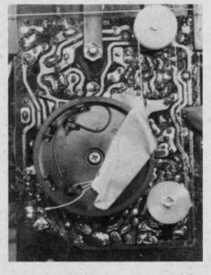
Fig. 7. If the dial drum must be moved during service, lock the cord onto the drum with tape to avoid unwinding the cord.
