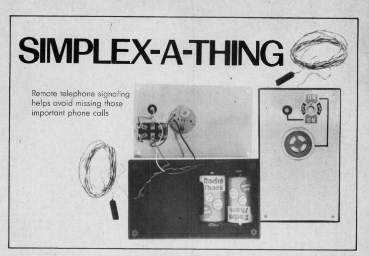
You won't Miss any more phone calls when out of hearing range of your telephone, if you add this simple remote signalling unit which alerts you to incoming calls by means of either a buzzer or blinker light. The unit is self powered for easy placement in any room in your home, or even outdoors where there are no AC outlets.
