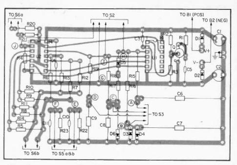
This is the component location guide used with the printed circuit board. Just about all of the components used in Imagician, with the exception of the switches, jacks and R24, are mounted directly on the board. Use IC sockets and be sure to orient them properly. Take special note of the takeoff points that lead away to the switches.
