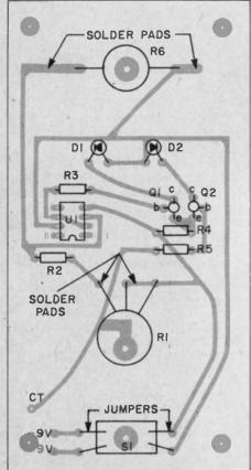
You'll note that parts layout diagram is viewed from foil side. This is done to aid in orienting the R1 and R6 connections.
