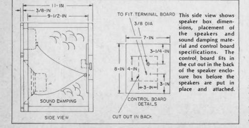
Properly assembled, the speaker box should fit inside the opening in the night table with no space at sides.
