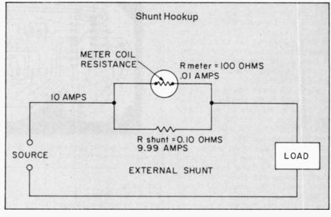
solving Ohm's Law for resistance the proper shunt can be found. This derivation is shown below:
