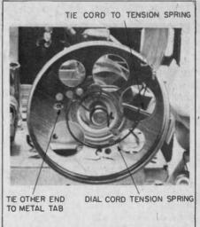
Fig. 5. Start the re-stringing by securing the cord to a tab or hole on the drum. End by securing the cord to the tension spring.
