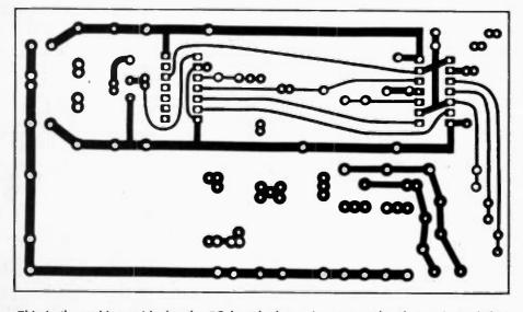
This is the etching guide for the PC board, shown in exact scale. If a project of this magnitude is beyond your abilities, you can obtain a ready-made circuit board from LEC-TROGRAPHIX. Their address and ordering information is shown beneath the parts list.
