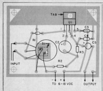
The component placement guide above shows the SPST switch mounted on the back of volume control R1 (dotted line box). External switch can be substituted for R1/S1.
