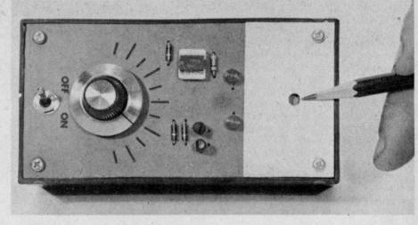
To make the front panel anti-glare mask, make a 3/16-inch hole in a piece of stiff oaktag apply cement to one side, center over the hole and press into position.
