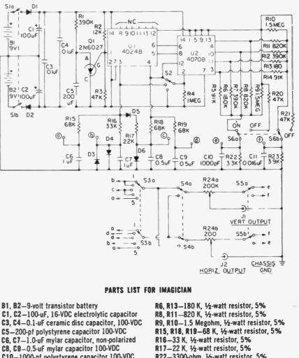
C10-1000-pf polystyrene capacitor 100-VDC C11-0.016-uF mylar capacitor 100-VDC D1 thru D6-1N914 diode J1, J2-BNC jack Q1-programmable unijunction transistor-2N6027, 2N6028 (Note: 2N6028 Available from SOLID STATE SALES. BOX 74A, Somerville, MA 02143.) R1. R7. R12-390 K, 1/2-watt resistor, 5% R2-12 K, ½-watt resistor, 5% R3, R20, R21-47 K, 1/2-watt resistor, 5% R4-1 Megohm, 1/2-watt resistor, 5% R5, R14-91 K, 1/2-watt resistor, 5%
