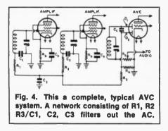
strength carrier, the voltage across C3 is constant regardless of the audio variations. The grid bias of any tube is the bias voltage measured from grid to cathode. If a stronger signal is tuned in the DC voltage across R4 rises, increasing the total bias applied to the tubes which reduces the amplification of the tube. Conversely, if the signal drops in strength the total bias applied to the tube decreases which increases the amplification of the tube.
