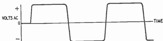
Fig. 107. Most square waves have rounded edges, sides are not truly vertical.
