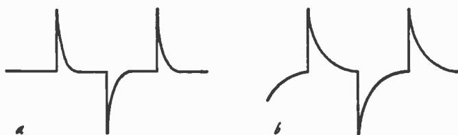
Fig. 810-a, -b. The shape of the pulse waveform can be altered by modifying the time constant of the r-c network.
