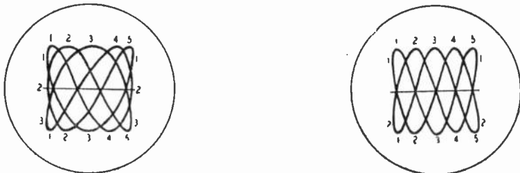
Fig. 806 and Fig. 807. In the illustration at the left (Fig. 806) we have a 5:3 ratio. Fig. 807 at the right shows a 5:2 ratio.
