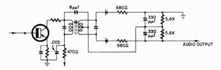
Fig. 714. In transistor FM, receivers, a pair of crystal diodes, are used in the detector circuit.
