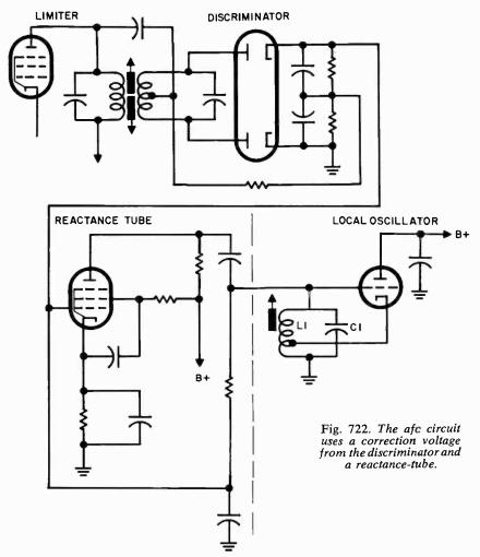
ment and then suddenly note that you are almost off the highway. An FM receiver (or an FM tuner) can be like that. Its front end can drift in frequency. It won't do this right away. It will wait until you are nice and comfortable in some easy chair listening to a good program.
