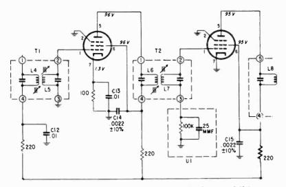
Fig. 718. If stages in a typical FM receiver. While the second if is not truly an if amplifier it is not completely a limiter either, since the plate and screen voltages are high. Some receivers use two stages like this for limiting, with amplification. The negative portion of the signal is clipped in the first stage, phase reversed in the tube and the positive portion of the signal (now negative) is clipped in the second stage. (Zenith Radio Corp.)
