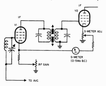
Fig. 921. S-meter circuit. The S-meter must first be adjusted to zero by means of the S-meter potentiometer.
