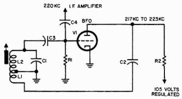
Fig. 905. This bfo is a Hartley oscillator.
