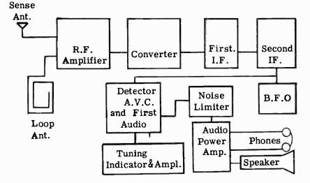
Fig. 1004. Block diagram of a marine radio receiver.
