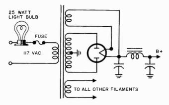
Fig. 708. Simple test to learn if power transformer has a shorted turn.
