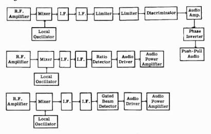
Fig. 701. FM receivers can use a number of different detector circuits.
