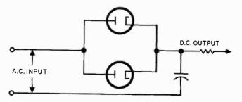
Fig. 706. Rectifier tubes can be connected in parallel. The trouble here is that the tubes won't wear out at the same rate.
