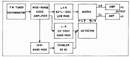
Fig. 724. Block diagram is typical of one multiplex stereo system. Circuitry and alignment procedure can vary from one manufacturer to another. Always follow manufacturer's instructions. (Philco Corp.)
