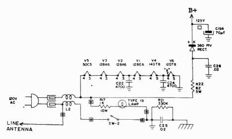
Fig. 702. Transformerless supply. The series filaments are bypassed by two capacitors. Capacitor C26 protects the rectifier from transient surges in the power line. (Arvin Industries, Inc.)
