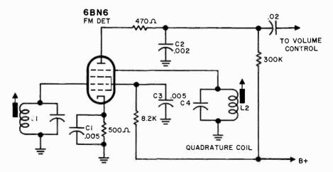
Fig. 716. Circuit of a gated beam detector. The input is coupled through an if transformer to the preceding stage.
