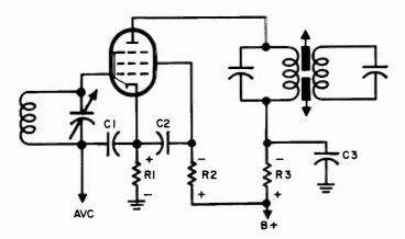
Fig. 812. If a circuit uses resistors, voltage analysis can be used to supply considerable information about all the components.
