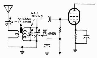
Fig. 917. Antenna trimmer is also helpful in separating stations.
