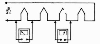
Fig. 603. Ac voltmeter method of locating an open filament. If the filament is good, the meter will read zero. If the filament is open, the meter will give a reading.
