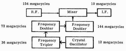
Fig. 1107. The local oscillator has a crystal and a number of frequency multipliers.
