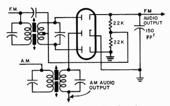
Fig. 815. This tube is a combined AM and FM detector. The FM section is a discriminator. The AM is the usual diode type detector.
