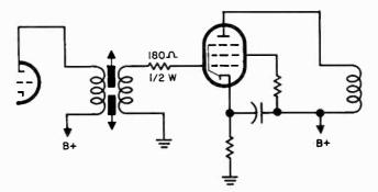
Fig. 719. A small resistor inserted in the grid circuit of an if stage will help stop oscillation. If the if tubes are shielded, make sure the shield fits well and makes good contact with chassis, ground, or B-minus bus. Try not to disturb the wiring in high-frequency circuits. Lead dress is important.
