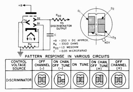
Fig. 822. Basic circuit of dual tuning indicator tube. Electron beam is spread by positive voltage and compressed by negative voltage applied to D2. (Sylvania Electric Products Inc.)
