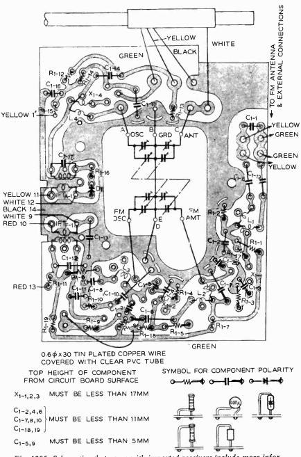
Fig. 1205. Schematics that come with imported receivers include more information than we are used to seeing. Here component polarity is indicated. In compact units component size and height are important. (Sony)
