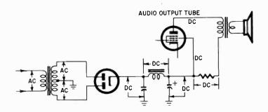
Fig. 703. Ac and dc voltage points in a power supply. All voltages, starting at the cathode of the rectifier, are dc. All voltages, starting at the rectifier plates and going back to the power line, are ac. The voltage drops across the filter capacitors, the filter choke and the filter resistor are dc. All tube voltages (no signal input) are dc.
