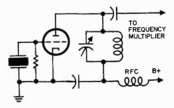
Fig. 1112. In this circuit the frequency is controlled by a quartz crystal. The tuned circuit must be able to resonate at the frequency of the crystal.
