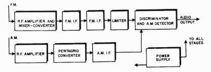
Fig. 808. In some tuners, the FM and AM sections are separate units.
