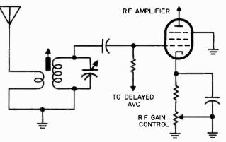
Fig. 919. Rf gain-control circuit.
