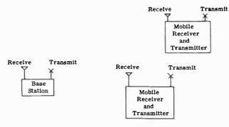
Fig. 1103. In this system, all units, base and mobile, can receive and transmit.
