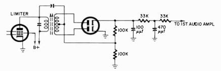
Fig. 713. The discriminator uses a double-diode as the detector.
