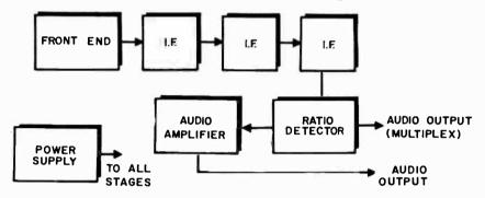
Fig. 806. FM tuner with three if stages, ratio detector and two audio outputs.
