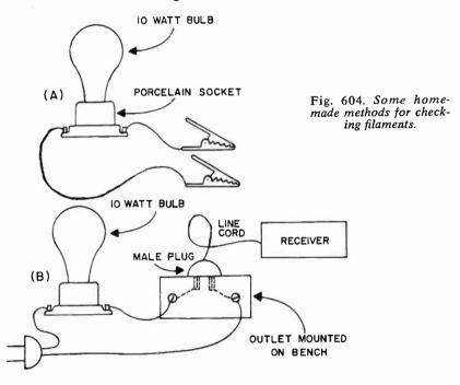
The quickest and easiest test is to connect a lamp or use a neonlamp tester. Even if this shows power at the outlet, don't take it for granted. The contacts in the outlet may be spread, or else the male plug on the line cord may have its prongs pushed apart.
