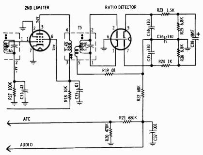
Fig. 715. The ratio detector does not eliminate AM completely. In some receivers one or two limiters are used ahead of the ratio detector. The detector supplies audio and also automatic frequency control voltage (afc). (Motorola Consumer Products, Inc.)
