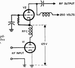
Fig. 1115. Cascode rf amplifier circuit. The two tubes are connected in series.
