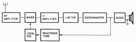
Fig. 721. Block diagram of FM receiver using afc.
