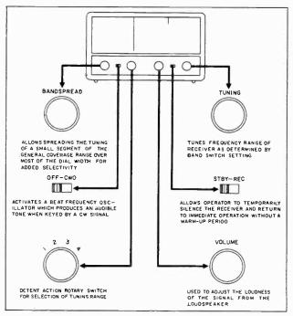
Fig. 906. Communications sets have a large number of controls. (National Radio Co. Inc.)
