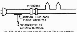
Fig. 608. If the receiver uses the power line as an antenna, try reversing the power-line plug if you have a hum problem. Removing the U-connector from the antenna terminal may help.
