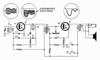
Fig. 1211. Reflex receiver gets maximum effort out of transistors.
