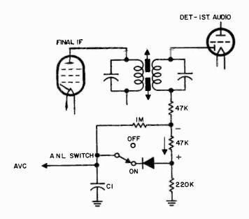
Fig. 1014. Anl (automatic noise limiter) circuit.
