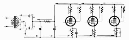
Fig. 705. The tubes in most circuits are connected in parallel. The current that flows through the tubes must also pass through the rectifier. The more tubes, the heavier the load (that is, the greater the amount of current). As you remove tubes, less current will pass through the rectifier. The arrows show the direction of electron current flow.
