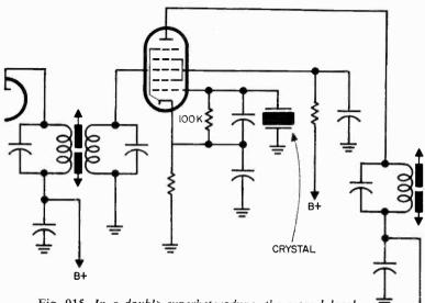
Fig. 915. In a double superheterodyne, the second local oscillator is fixed-tuned. In this case, a crystal oscillator is used.
