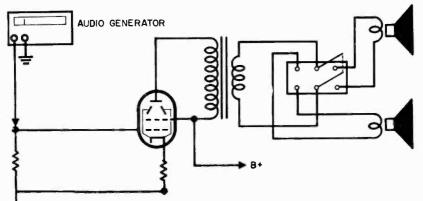
Fig. 614. To see if a speaker needs to be replaced, connect the old speaker and a new one to a double-pole double-throw switch. Operate the switch and listen carefully. If you can hear a definite improvement, replace the old speaker.
