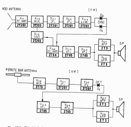
Fig. 1203. This block diagram of the AM-FM transistor portable shows that more stages are used for FM broadcast reception (top) then are required for AM broadcast listening. (Sony)
