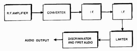
Fig. 807. This FM tuner has two if stages and a limiter, followed by a discriminator-type detector.
