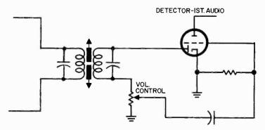
Fig. 1011. Volume control works as the diode load.
