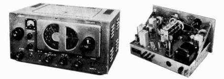
Fig. 910. With 9 tubes and 10 controls this communications receiver chassis is not crowded. Speaker is in separate cabinet. (Lafayette Radio Electronics Corp.)
