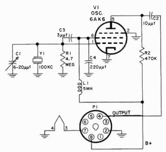
Fig. 913. Crystal calibrator helps make the receiver a precision frequency instrument. (National Radio Co., Inc.)
