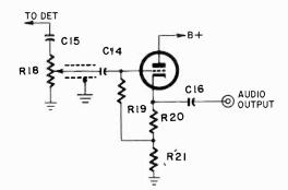
Fig. 817. In some tuners, a cathode follower is the audio output stage. The signal at the output of the follower is less than at the input.
