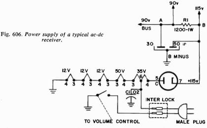
it in only one direction. The result isn't pure dc but with the help of a filter, we get a voltage that's smooth enough for our tubes.
