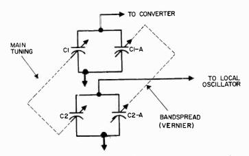
Fig. 907. Communications receiver tuning and bandspread capacitors operate independently of each other.
