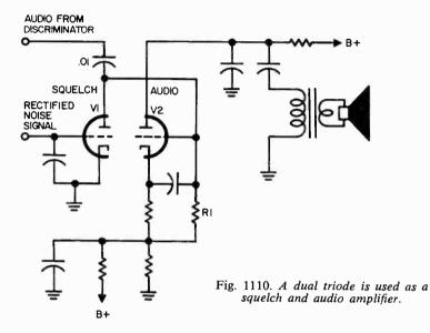
voltage is produced. As a result, V1 runs hog wild since there is nothing to restrain its plate current. It has no bias on it and so the plate current of V1 manages to reach the top of its limit.
