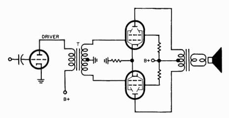
Fig. 711. Push-pull output stage. Interstage push-pull transformer T couples the driver of the push-pull tubes. Good interstage transformers are expensive, take up room. Most sets use a tube (or a transistor) as a phase inverter to take the place of the transformer.
