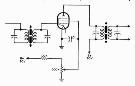
Fig. 1013. Volume control in the screen circuit of an if tube.
