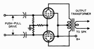
Fig. 618. A properly designed push-pull stage produces less distortion than a single-ended audio amplifier.
