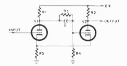
Fig. 614. Basic Schmitt trigger circuit is used to generate uniform pulses from various input waveforms.
