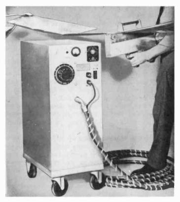
Fig. 311. This impedance-matched generator uses a long cable to take the work head to the job.
