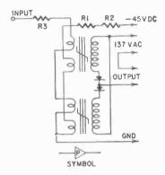
pleted. This is, of course, nothing new in industrial controls, but usually this sort of thing has been handled with relays which are subject to wear, mechanically, and to contact failure, etc. With the nonmoving CYPAK or similar units, the system is dependable as long as there is power to operate. (Relays would also fail with power failure, of course.)
