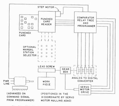
Fig. 921. This block diagram has a punched-card reader to program numerical positioning system. Only lead screw-drive portion of system is shown.
