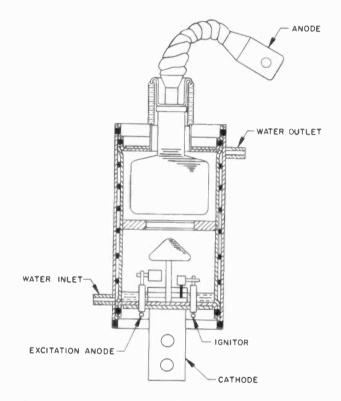
Fig. 210. Drawing of a typical mercury-pool rectifier shows location of connections. Tube is enclosed by a water jacket.
