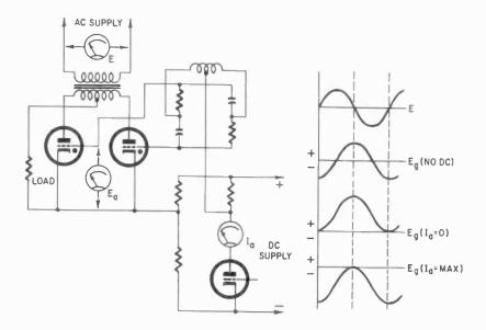
Fig. 723. This thyratron circuit has a fixed phase shift and a variable dc bias controlled by the vacuum tube. Waveforms show effect of bias variations and relation to thyratron plate voltage.
