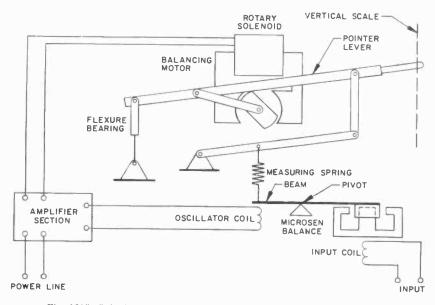
Fig. 1015. Principle of operation of the Microsen recorder is simplified in this diagram.
