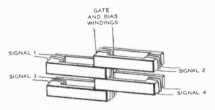
Fig. 835. Stacked cores for and unit have common gate and bias winding but separate signal windings.
