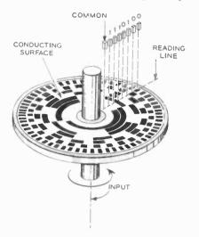
Fig. 914. Shaft-position transducer is used to convert rotation into binary-digital form.
