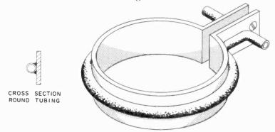
SINGLE-TURN COIL WITH COOLING TUBE SOLDERED TO OUTSIDE
