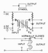
Fig. 818. Ramey not circuit with symbol and relay equivalent. As in the relay circuit, if an input is present, there is no output.
