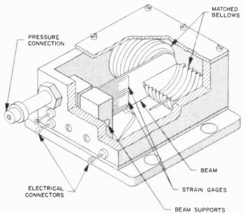
Fig. 1105. This pressure transducer uses bonded strain gages attached to the beam, which is flexed by the bellows. Vacuum gages are also built using this principle.
