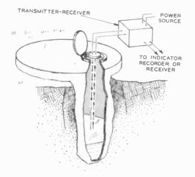
Fig. 1110. Sonic level indicator sends high-frequency sound pulse to boundary layer where it is reflected. Time difference between pulse and echo is measurement of level. Sound can also be sent through liquid but this is less likely to be accurate.
