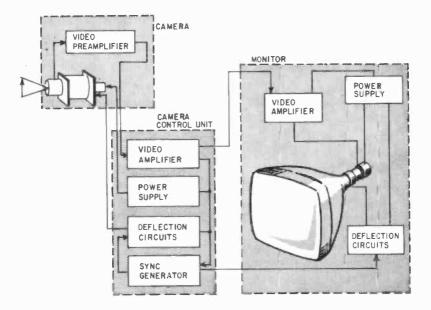
Fig. 1122. This block diagram shows the simplification when rf carrier is eliminated.
