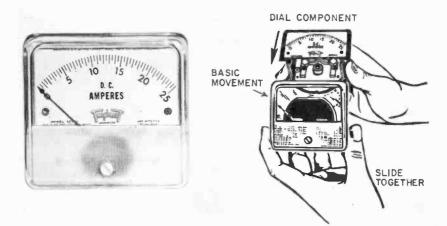
Fig. 1204. Handy for laboratory and bench test setups, the interchangeable units are useful in industrial electronics servicing. (Triplett Electrical Instrument Co.)
