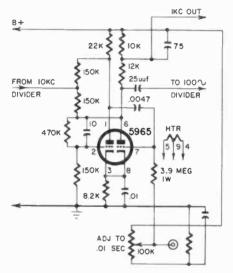
Fig. 603. Typical frequency-divider stage can be used in many timing devices.
