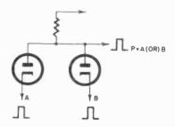
Fig. 810. Gates for and and or functions can be made with either diodes or multi-grid tubes.
