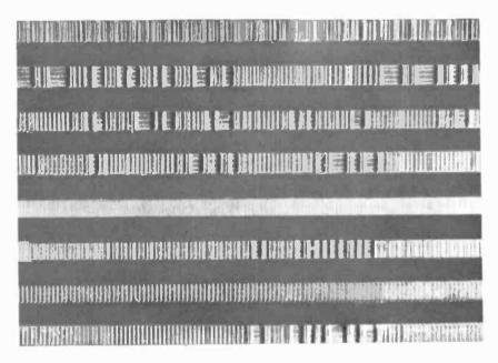
Fig. 809. Information stored on magnetic tape can be made visible with fine iron powder.
