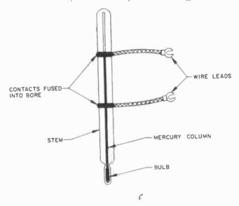
Fig. 1107-c. Contacts inserted through the glass during the manufacture of this highly accurate thermostat complete the circuit through the mercury column.
