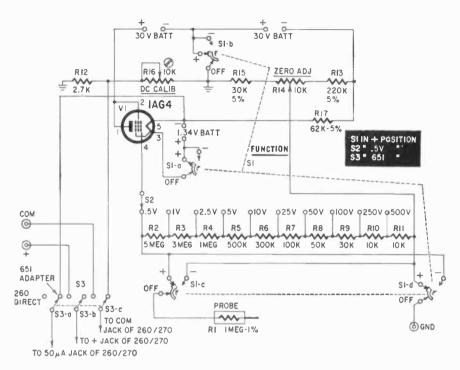
Fig. 1206. Schematic of vtvm adapter shows single tube and switching circuit that allow vom operation without removing adapter.
