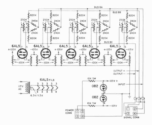
Fig. 927. Pacuum-tube diodes have economically sound characteristics for this function generator.
