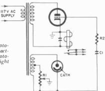
Fig. 715. Typical ac-powered photoelectric relay circuit. Triode grid, acting as diode plate, charges C1. Phototube discharges capacitor when light strikes cathode.
