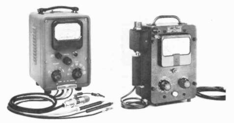
Fig. 1210. Laboratory vtvm (a) performs all the familiar functions with greater accuracy while the unit at (b) only indicates voltage. (Hewlett-Packard Co. and General Radio Co.)
