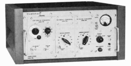
Fig. 604. It is necessary to hetrodyne a high frequency that is not within the frequency range of a counter. Stable oscillators can be included in the same case. (Beckman, Inc.)
