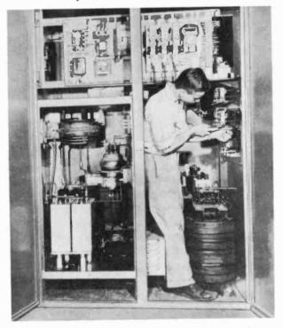
Fig. 103. Large induction generator being adjusted by technician. (General Electric Co.)
