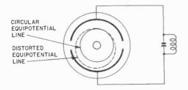
Fig. 1127. Distortion of equipotential lines by lowering the B-plus on one anode will cause electrons to "fall" toward that anode.
