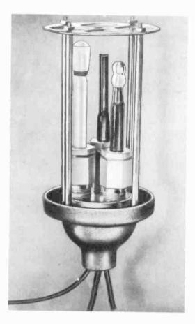
Fig. 1114-a. Glass electrode assembly used in pH measurements.
