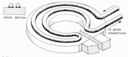
FLAT SINGLE-TURN COLL WITH REVERSED LOOP OF COOLING TUBE SOLDERED TO INSURE ADEQUATE COOLING
