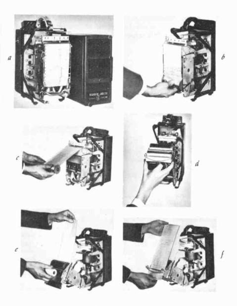
Fig. 1020. The chart-removal sequence: remove case (a), full out takeup spool (b), remove unused chart paper (c), remove empty spool (d), start new roll (e), thread new paper through guides (f). Procedure is similar for most recorders and is detailed in their individual maintenance manuals. (General Electric Co.)
