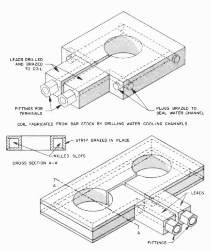
COIL FABRICATED FROM BAR STOCK BY MILLING WATER COOLING CHANNELS.
