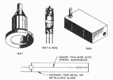
Fig. 213. Geiger-Muller tubes have a variety of shapes. The basic internal construction is shown. (Victoreen Instrument Co.)
