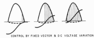
Fig. 724. Comparing pure phase-shift and combination phase-shift voltage firing of thyratrons. Note that in both cases the grid voltage curve passes the firing point at a very obtuse angle.
