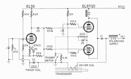
Fig. 318. Generator for ultrasonic soldering tool.
