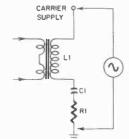
and, with the proper values in the circuit, this can be a saturation current. This then is a ferroresonant point. The core will be maintained at saturation. However, although a trigger can start the swing toward saturation, it is not possible to desaturate the core with a pulse, at least not directly through the control winding. To achieve this the voltage of the carrier must be lowered, which is analogous to extinguishing a thyratron.
