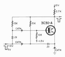
Fig. 507. One-shot multivibrator (upper left) provides delay between input and output. Basic memory circuit (right) gives either positive or negative output pulses. Flip-flop in binary stage (lower left) is also simplified by PNPN transistor. Other accessories to the electronic decade type of counters will be discussed in the next chapter under applications. The electronic counter can be a very versatile instrument.
