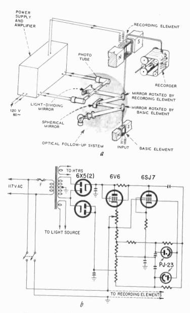
Fig. 1001. The mechanics of the deflection type photoelectric recorder are diagrammed at (a) and the electronic portion is detailed in the schematic at (b).
