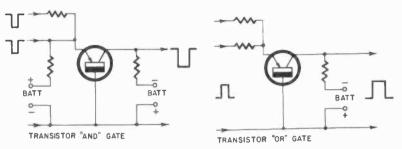
Fig. 811. Transistors are preferred for most computer applications. Their use reduces the need for cooling equipment as well as making a more compact device.
