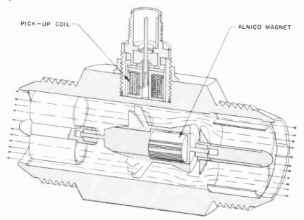
ELECTRONIC FLOW SENSING ELEMENT
