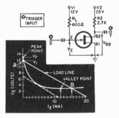
Fig. 906. Basic Unijunction transistor circuit is bistable. Emitter characteristic curve is typical.
