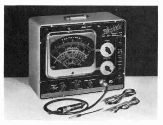
Fig. 1209. This medium-priced vtvm will measure inductance, capacitance, resistance as well as ac and dc voltages. (Hickok Electrical Instrument Co.)
