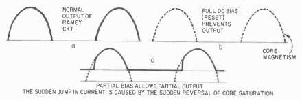
Fig. 814. Output currents from Ramey unit with dc reset.
