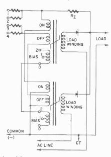
Fig. 829. Switching unit made from conventional magnetic amplifier can be used for logic functions.
