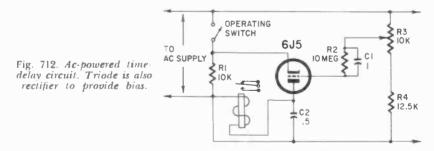
out after a sufficient *charging* time had elapsed. Such circuit variants are also available commercially.
