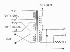
Fig. 834. Pulsed memory circuit.
