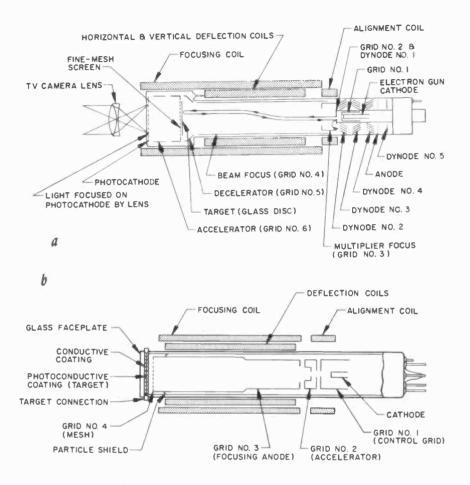
Fig. 212. The vidicon (a) and orthicon (b) are used with lens systems as signal pick-up tubes in industrial and broadcast TV.
