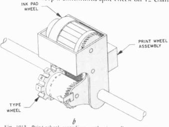
Fig. 1013. Print-wheel recording mechanism allows many channels to be "read". Only samples are recorded. Most transients go unindicated.
