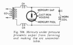
gap distance considerably, and thus would affect the output of the generator. In fact, the accepted way of adjusting the current through the work coil is to change the gap, so that the spark will persist over more or less of the half-sine wave from the power transformer. The earlier the gap breaks down, the longer it persists, and the greater the average power produced by the generator.
