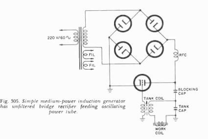
a typical induction-heating generator of moderate power. Notice that there is a power supply with a full-wave bridge rectifier but no filter. In communications, we would not want to tolerate 60cycle modulation (or, in this case, 120 cycles) of the generated rf, but in heating, it is of no concern.
