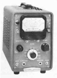
Fig. 1214. Direct-reading frequency meter needs no adjustment or interpolations to determine frequency. Counters are also used for this type of measurement. (Hewlett-Packard Co.)
