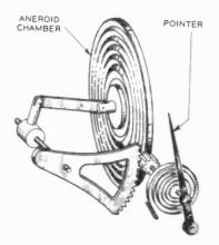
Fig. 1101. Aneroid chamber responds to air pressure. A potentiometer in place of the pointer would make this a barometric transducer.
