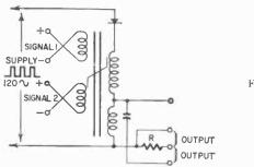
Fig. 832. Pulsed not circuit.
