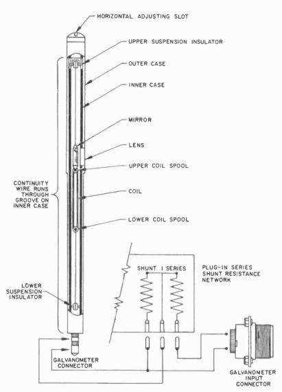
Fig. 1024. This subminiature galvanometer movement is shown nearly twice its normal size. Some models will indicate at 5,000 cycles.
