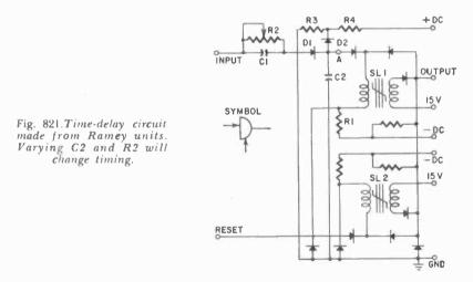
As long as the input continues, without this clamping action C2 would continue to charge and would require a higher voltage capacitor. Also, it is possible to discharge C2 faster if the voltage on it is lower. Functionally, the clamp D2, R3 and R4 would not be absolutely necessary. Discharge of C2 takes place when a signal is applied to the "reset" unit, and clamped at zero by D3 (otherwise it would go negative from the reset input). If a simultaneous
