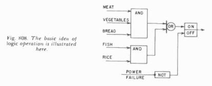
AND, OR and NOT gates we can delineate any complex set of conditions about anything we wish, so long as the conditions are clear-cut. Ambiguous conditions would simply be unclassifiable in our logic machinery.
