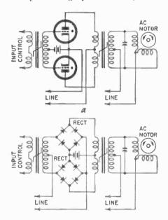
Fig. 841. Thyratron and magnetic-amplifier circuitry to control a split-phase motor are quite similar.
