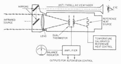
Fig. 1107-e. Infrared radiation pyrometers are useful in determining surface temperatures without actual contact.
