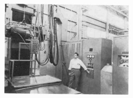
Fig. 917. Tape drive mechanism housed in cabinet at right is only a small part of the elaborate electronic control system needed to program machine process.
