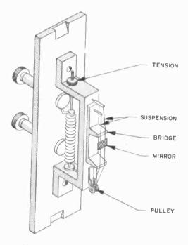
Fig. 1023. String galvanometer assembly depends on the magnetic field around the wires to twist the mirror when in place in their normal permanent magnetic field.
