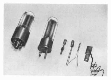
Fig. 714. Photosensitive devices have many forms.
