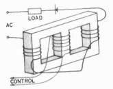
Fig. 802. Basic magnetic amplifier. Ac fields cancel in central core section.
