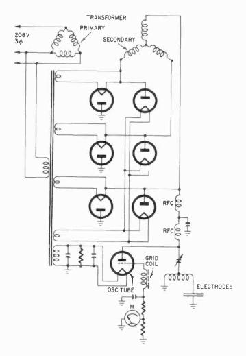
Fig. 308. Simplified schematic of a typical directloaded dielectric generator has dc supplied by a three-phase full-wave rectifier.
