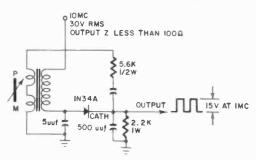
Fig. 516. Pulse feedback makes a freerunning multivibrator of the basic ferristor circuit.
