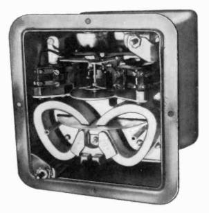
Fig. 706. Eddy-current disc motor is strong enough to operate contacts in this time-delay device.
