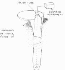
Fig. 1111. Radioactive level measurement uses low-grade radioactive source, measures absorption by column of liquid.
