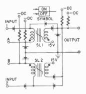
Fig. 820. This memory is made with two combination or and not units. See text.
