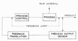
Fig. 729. Block diagram shows principal components of a servo system.
