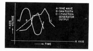
Fig. 928. Function generator can create waveforms for special conditions that cannot be satisfied with sawtooth and sine waves.
