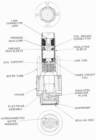
Fig. 1106. The capacitive transducer has plates connected to some form of tuned circuit. High pressures produce minute capacitance changes. External circuitry for this transducer is more complicated than for the potentiometer type.
