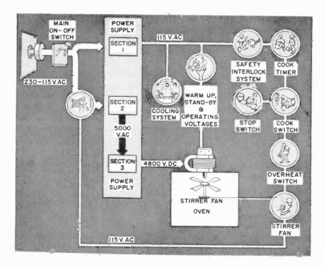
Fig. 1123. All microwave cooking devices have circuitry similar to this, outlined in block form. (Raytheon Corp.)
