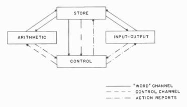
Fig. 922. Block diagram of basic digital computer.
