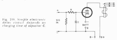
Timing by charging capacitors is a relatively old subject to most readers who understand electronics. Thus the circuit of Fig. 710 is quite familiar. In this circuit, the capacitor must be charged by dc until the voltage on it is sufficient to overcome the negative grid bias, whereupon the tube will conduct and energize the relay. This same operation can be made linear in time by using a charging tube (Fig. 711) but the principle is basically the same.
