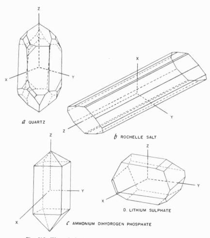
Fig. 316. The principal transducer crystal materials and their crystallographic axes.
