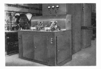
Fig. 307. A 25-kw induction heater is used to harden valve stems. (General Electric Co.)
