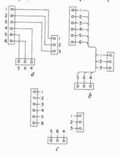
Fig. 203. Schematic in (a) indicates wire connections between terminals. Connections in (b) and (c) could indicate individual wires or multiple wire cables. Additional data on the print would clarify this.
