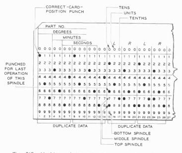
Fig. 919. Machine-tool program instructions may be punched into cards. Both cards and tape may be used in one system.
