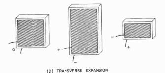
Fig. 315. Piezo-electric crystals distort when subjected to a dielectric field. This change of shape is dependent upon the crystal type, cut and field polarity.
