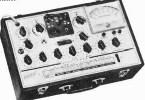
Fig. 1208. A transconductance type tube tester is essential for preventive maintenance. (Hickok Electrical Instrument Co.)
