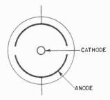
Fig. 1125. Basic structure of magnetron is simple, with two plates and a heated cathode.
