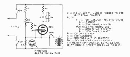
Fig. 716. Ac-powered thyratron photoelectric relay circuit energizes relay when light hits phototube.
