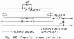
duces one type of interference while the capacitors grounded to fixture remove most of the hash.
