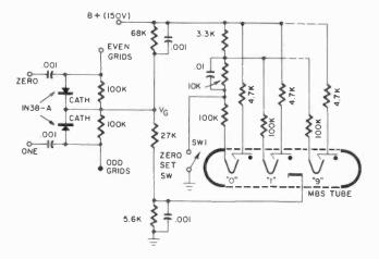
Fig. 512. Schematic of basic beam switching drive circuit.
