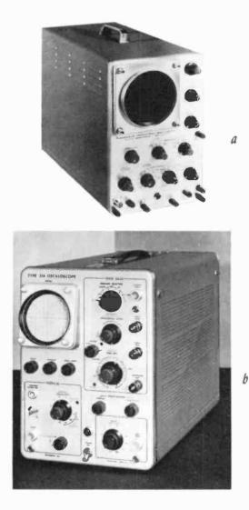
Fig. 1211. Scope (a) built from kit can handle most industrial electronics jobs. More expensive portable 3-inch scope (b) has wide range. (Heath Co. and Tektronix, Inc.)
