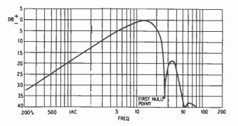
Fig. 326. Effect of gap width upon output of a high-quality record-playback head at 7.5 ips. (Source: Otto Kornei, "Structure and Performances of Magnetic Transducer Heads," Journal of the Audio Engineering Society, July, 1953.)
