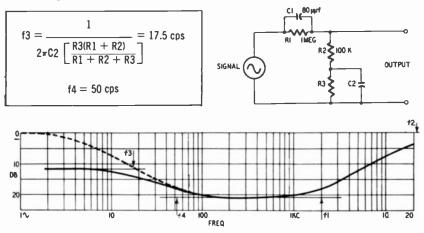
Fig. 722. Modification of response curve in Fig. 721 to produce less bass boost below 20 cycles. The dashed line is the response in Fig. 721.
