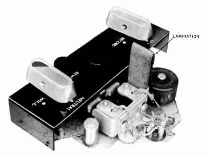
Fig. 1005. "Gimmick" used to minimize hum pickup by playback head of a moderate-price tape recorder.
