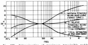
Fig. 605. Approximation of maximum permissible treble and bass boost in recording.
