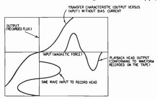
Fig. 502. Reproduction of a sine wave without bias current.
