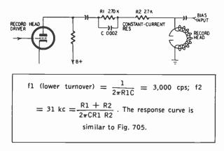
Fig. 720. Example of treble boost produced by an R-C losser circuit.
