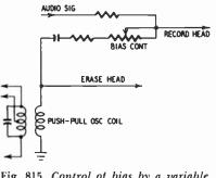
Fig. 815. Control of bias by a variable resistance.
