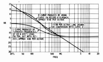
Fig. 707. Response curve having a slope of about 3 db per octave.
