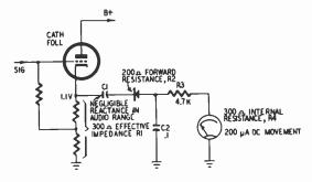
Fig. 911. Circuit of a peak-reading meter.
