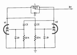
Fig. 805. Typical push-pull oscillator. Oscillator frequency typically 30,000 cps.
