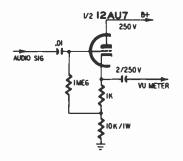
Fig. 909. Cathode follower suitable for driving a VU meter.
