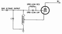
Fig. 802. Single-ended oscillator employing cathode-to-grid feedback.
