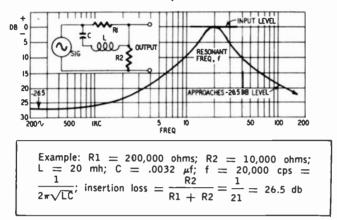
Fig. 703. Response of an R-L-C circuit.
