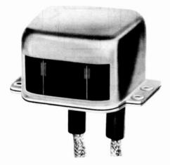
Fig. 108. Combination record-playback and erase head (half track.) Courtesy, Shure Brothers, Inc.
