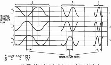
Fig. 325. Magnetic potentials scanned by a playback head for three wavelengths (A, B, C) at different phases (1, 2, 3).
