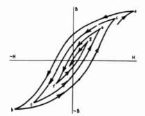
Fig. 327. Behavior of a magnetic particle in the tape during the ac erase process.
