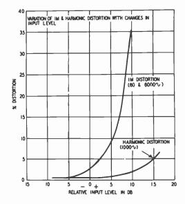
Fig. 401. Measurements of input level are based on the peak value of the test signals. The bias current is approximately optimum for the machine and tape used in making these measurements. 0-db input level corresponds approximately to a 0 reading on the tape recorder's VU meter. (Source: Audio, October, 1956.)
