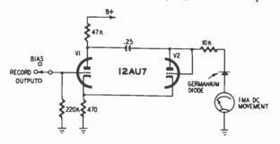
Fig. 910. Vtum type record-level indicator.
