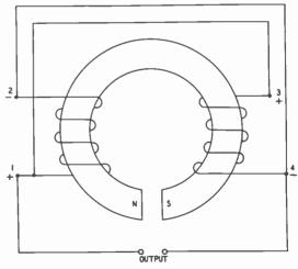
Fig. 317. Parallel connection of dual windings.
