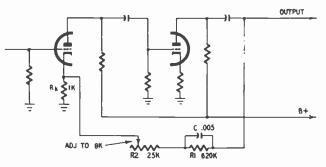
Fig. 726. Bass-boost circuit using voltage feedback over two amplifier stages.
