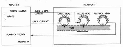
Fig. 102. Fundamental units of a tape recorder.
