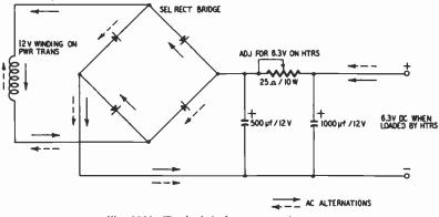
Fig. 1011. Typical dc heater supply.
