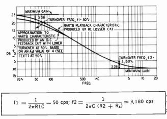
Fig. 727. Comparison of bass-boost curves produced by R-C losser and feedback circuits.
