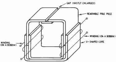
Fig. 315. Structure of a nonlaminated head with a removable pole piece.
