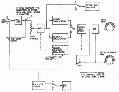
Fig. 107. Basic elements of a tape amplifier for use with a record-playback head. Many two-head recorders use the same equalization in record and playback. In the diagram shown above, all switches operate simultaneously. (R means record, P is playback.)
