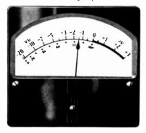
Fig. 901. Volume-unit (VU) meter showing A scale.
