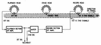
Fig. 103. Elements in sound-on-sound recording.
