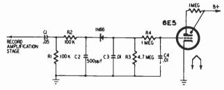
Fig. 915. Use of an electron-ray tube as a record-level indicator with "floating action." (Viking RP61 tape amplifier)
