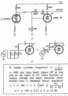
Fig. 729. Interstage plate-to-grid feedback circuit producing bass boost.
