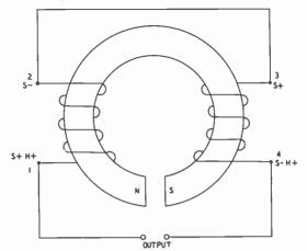
Fig. 316. Hum-bucking effect produced by series connection of dual windings. S denotes instantaneous signal polarity. H denotes instantaneous hum polarity.
