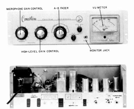
Fig. 206. Two views (front and rear) of a tape recorder amplifier. (Courtesy, American Electronics, Inc.)
