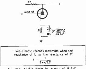
Fig. 711. Treble boost by means of R-L-C current feedback.
