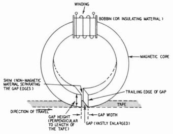
Fig. 312. Basic structure of the tape recorder head.
