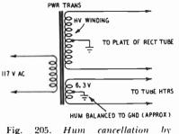
Fig. 205. Hum cancellation by grounding the heater winding.
