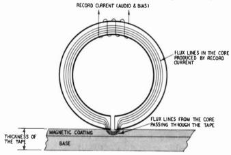
Fig. 320. Operation of the record head.
