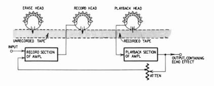
Fig. 104. Method for production of an echo effect.
