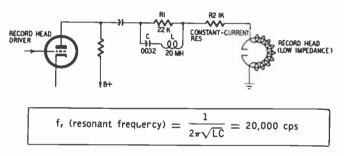
Fig. 718. Example of treble boost produced by an R-L-C- losser circuit.
