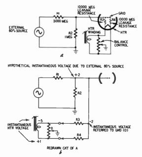
Fig. 1010. How the balancing potentiometer cancels hum.
