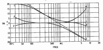
Fig. 611. Ampex equalization of a tape recorder operating at 3.75 ips. 1: Ampex bass boost: 2-2: equalized response: 3'-3' required record characteristic; 4: required treble boost to compensate treble record losses.
