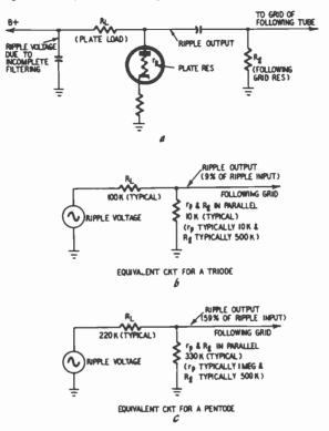
Fig. 1008. Reduction of 120-cycle hum by use of a triode.
