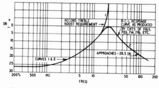
Fig. 712. Use of an R-L-C- response curve to match record treble-boost requirement of a tape recorder operating at 7.5 ips.
