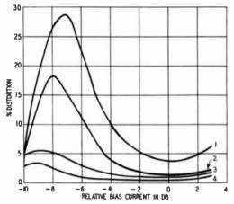
Fig. 503. Variation of IM and harmonic distortion with changes in bias current. Curve 1: IM distortion at playback level corresponding to +3 on VU meter. Curve 2: IM distortion at playback level corresponding to 0 on VU meter. Curve 3: Harmonic distortion at playback level corresponding to +3 on VU meter. Curve 4: Harmonic distortion at playback level corresponding to 0 on VU meter. (Source: Audio, October, 1956.)
