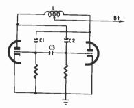
Fig. 806, Variation of the pushpull oscillator. C3 is appreciably larger than C1 and C2.
