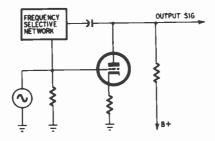
Fig. 708. Plate-to-grid voltage feedback.
