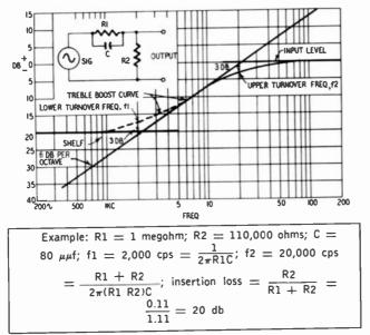
Fig. 705. Treble boost produced by an R-C losser circuit.
