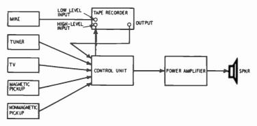
Fig. 101. Basic arrangement of a tape recording system.
