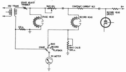
Fig. 921. Typical bias and erase metering circuit.
