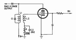
Fig. 801. Single-ended oscillator, employing plate-to-grid feedback.
