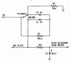
Fig. 1003. Method of preventing switching transients.
