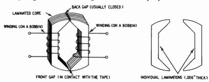
Fig. 313. Details of a laminated head.
