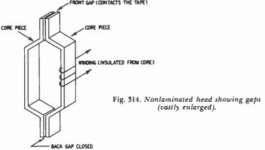
head can be made of two C-sections (Fig. 314) or it can be made of two sections as shown in Fig. 315. Here one of the sections
