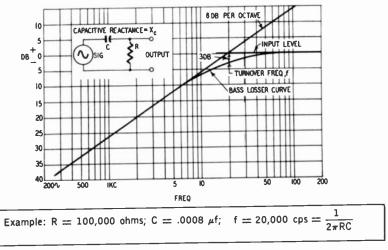
Fig. 702. Bass droop produced by an R-C losser circuit.
