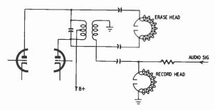
Fig. 811. Direct coupling of the push-pull oscillator to the erase head.
