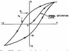
Fig. 309. Hysteresis loop of a magnetic material.
