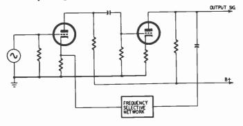
Fig. 709. Plate-to-cathode voltage feedback.
