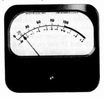
Fig. 902. I'U meter with type B scale.
