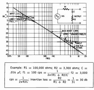
Fig. 704. Bass boost produced by an R-C losser circuit.
