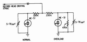
Fig. 917. Use of dual neon lamps as a record-level indicator. (Wilcox-Gay 4A10)
