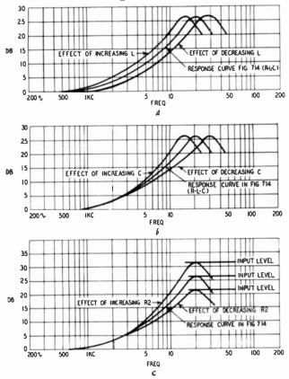
Fig. 716-a. Effect of varying L in Fig. 714; b) effect of varying C in Fig. 714; c) effect of varying R2 in Fig. 714. Input levels are actually the same for all curves, but are shown differently for clarity of presentation.
