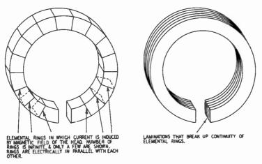
Fig. 322. Cause and reduction of eddy-current losses.
