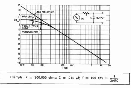
Fig. 701. Treble droop produced by an R-C losser circuit.
