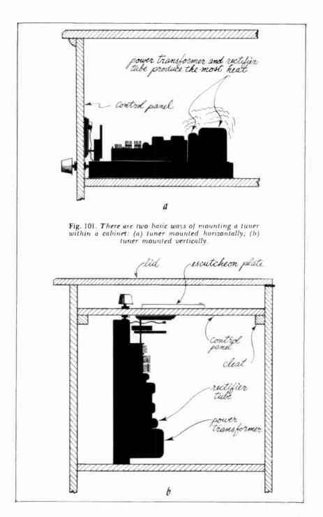
reduction in height or width of tuners simplifies cabinet installation since it reduces the amount of control panel space required by the unit. Considerable reductions, particularly in height, have been made in the physical size of tuners. Tuners are now made in such a way that heights of over  $41/_2$  inches are relatively uncommon. This has made it possible to stack tuners and amplifiers, resulting in extremely compact control panels.
