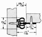
Make sure that the drawer slide will be able to carry the weight of the equipment. The drawings at the left show ballbearing catches—a few of the many different types that could be used.
