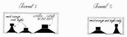
Fig. 121. Stereo setup using different speaker systems.
