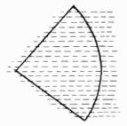
Fig. 519. A variation of plain-slicing uses quartered logs. Called quarter-slicing, this method results in grain patterns composed of narrow straight stripes.
