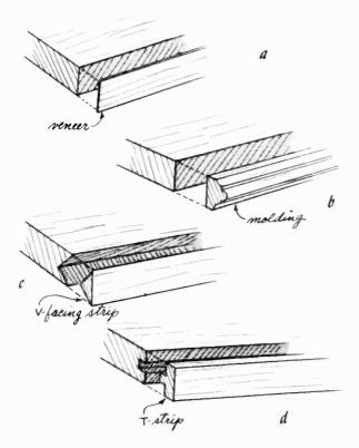
Fig. 623. Edging is available in a variety of forms: a) simple veneer stripping; b) decorative molding; c) V facing strip; d) T facing strip.
