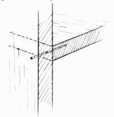
Fig. 616. Internal partitions can be fixed in place with plain butt joints. However, this is the least desirable method
