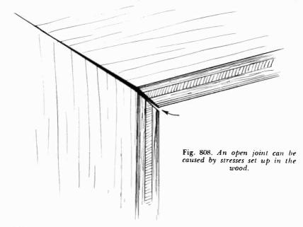
reinforce and pull the joint back together. If, however, the open joint is in a readily visible area, they cannot be used, and you'll have to rely entirely on glue and pressure.
