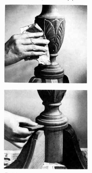
Fig. 703. Curved and carved portions of the cabinet must be finished by hand. Do not use a sanding block. (Courtesy Grand Rapids Varnish Corp.)
