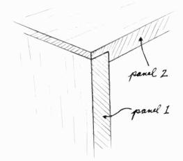
Fig. 610. The shoulder butt joint is stronger than the plain butt and makes finishing easier by eliminating much of the exposed end-grain of the wood.
