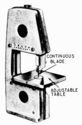
Fig. 606. The band saw is especially suitable for cutting curves. (Courtesy Delta Power Tool Div., Rockwell Manufacturing Co.)
