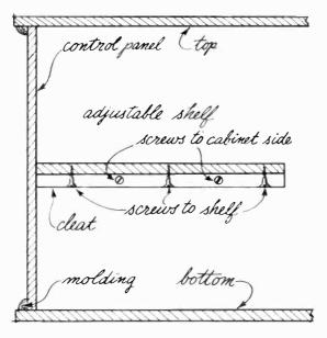
Fig. 111. Construction of a tuner-amplifier compartment.
