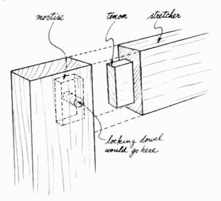
Fig. 621. The mortise and tenon joint, although a bit more difficult to handle, is much stronger than the doweled joint.
