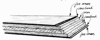
Fig. 521. Cut-away view of the internal construction of \$4-inch veneer-core plywood.
