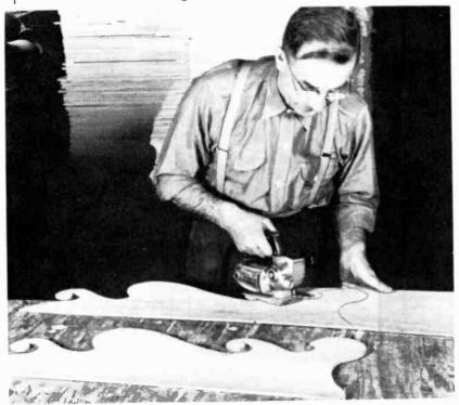
Fig. 607. The sabre saw is another machine which is excellent for culting curves. (Courtesy Porter-Cable.)
