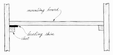
Fig. 106. When a cabinet is not level, the turntable can be adjusted by inserting a shim between the mounting board and the cleat supporting it.
