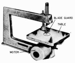
Fig. 608. Another useful machine for curved work is the power jig saw. (Courtesy Delta Power Tool Div., Rockwell Manufacturing Co.)
