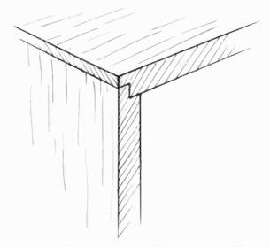
Fig. 611. The double-shouldered butt-joint, although stronger than the shoulder-butt, is not often used. Its complexity defeats its advantages.
