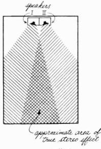
Fig. 217. Sound distribution pattern in a rectangular room.
