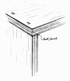
Fig. 609. One of the simplest methods of joining wood is the butt joint.
