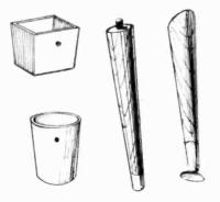
Fig. 529. Ferrules for wooden legs are available in brass. They are primarily designed for round tapered legs.
