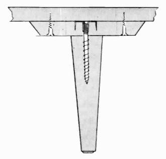
Fig. 626. A mounted leg showing T-nut, wood plate and hanger bolt.
