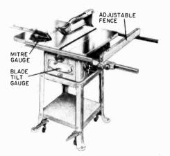
Fig. 602. The table saw (tilting arbor circular saw) complete with adjustable fence and mitre gauge. (Courtesy Delta Power Tool Div., Rockwell Manufacturing Co.)
