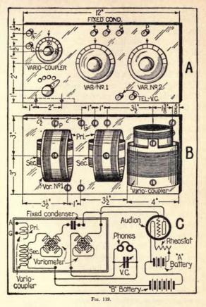
and from  $\frac{1}{8}$  to  $\frac{3}{8}$  inches thick. The measuring and drilling for the necessary holes should be done
