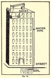
ser, in other words, cuts down the wave-length to a point where it counter-balances the excessive wave-length of the ground. Such a condenser should always be used when there is a long ground, as for instance, in apartment houses, high office buildings etc.
