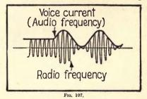
often spoken of as the carrier wave, because it carries the speech waves with it. This is shown in Fig. 107, schematically where the speech waves will be seen carried along with the continuous waves, which are emanating from the oscillating circuit.
