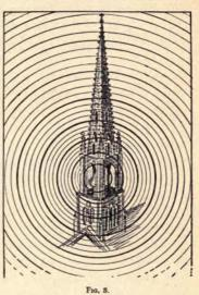
would be a sort of invisible globe all around it. The wave rapidly branches out, becoming larger and larger, always remaining, however, in the form of a sphere, as seen in Fig. 3. If the sound waves do not go out in the form of spheres, it would not be possible for us to hear them in all directions as we have seen in Fig. 2. We, therefore, come to the conclusion 2
