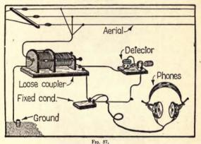
will describe presently. When the connections are made, as shown in Fig. 37, we must keep the secondary all the way in, and then adjust the slider on the primary until we hear the signals well. We now slide the secondary in and out, more or less, and in doing so, we move the slider upon the secondary also, until we reach a point where signals are loudest. This point is different for every station to which we are listening.
