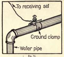
to use an ærial without a ground for short distances, in which case it becomes a sort of loop. For ordinary purposes, however, it would be impossible to use a radio outfit without a ground connection. Fig. 75 shows the simplest and perhaps the best. It is simply a wire fastened to the cold water pipe, which is found in almost every house and apartment. In order to make a good connection, we use a ground clamp, as shown in Fig. 76. This ground clamp is simply a piece of metal band wrapped around
