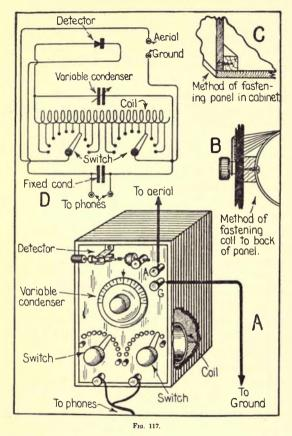
The tuning coil is of No. 24 enamel insulated magnet wire, wound on a cardboard tube
