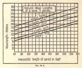
The accompanying charts shown in Figs. 74A and 74B have been compiled by taking the average wave length of several ærials of the same size erected at different places and give sufficient accurate measurements for the ordinary types of antennæ used by amateurs. Fig. 74A shows the natural wave length of an ærial of the "T" type, that is, those of which the lead-in is taken from the exact center. Above each curve is marked the height
