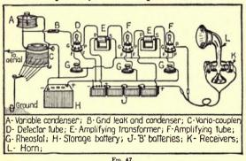
termed the secondary. The ratio of these transformers is usually such that, electrically speaking, the value of the secondary is about ten times as much as that of the primary. The audio frequency transformer is in principle the same as the loose coupler, which we studied before, and the purpose of the audio frequency transformer is to transform the energy from a low level to a high one. The purpose of this transformer, as shown in Fig. 47, is to boost up the weakest signals, trans-
