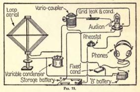
instruments. Fig. 72 shows the simplest connection of a loop ærial, with the simplest regenerative vacuum tube hook-up.
