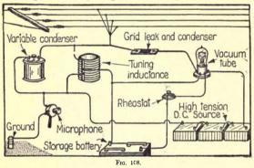
reason that we now make use of the vacuum tube. Even the simplest telephone transmitter such as used on your house telephone can be used in the modern radio telephone, and the main reason is that the vacuum tube sender acts as a valve, which amplifies many thousand times the voice current, sending it out over the ærial without having a strong current passing through the microphone.
