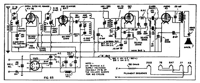
The A.C.-D.C. principle of operation is illustrated by the RCA-Victor model R-22 set.
