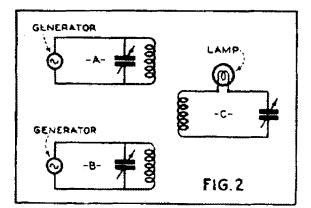
Electrical circuits for mixing frequencies.
