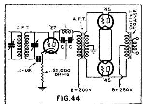
Second detector and audio amplifier circuit. In a later receiver, we might find the 27 tube replaced by a 56 and the 45 tubes by 2A3s. Similar changes without difference in operation may be included in Fig. 45 and 46.
