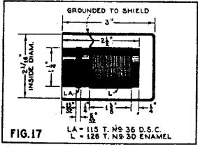
Antenna coil data for circuit Fig. 15.
