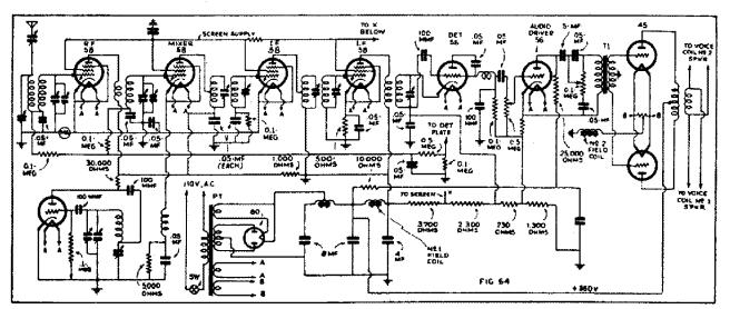
The circuit diagram of the Bosch model 250 receiver demonstrating A.V.C. and resonance indicator.
