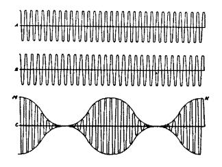
Fig. 1. Showing how a beat note is produced by adding two currents of different frequencies.
