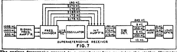
The various frequencies present in a superheterodyne receiving the station illustrated in Fig. 6.
