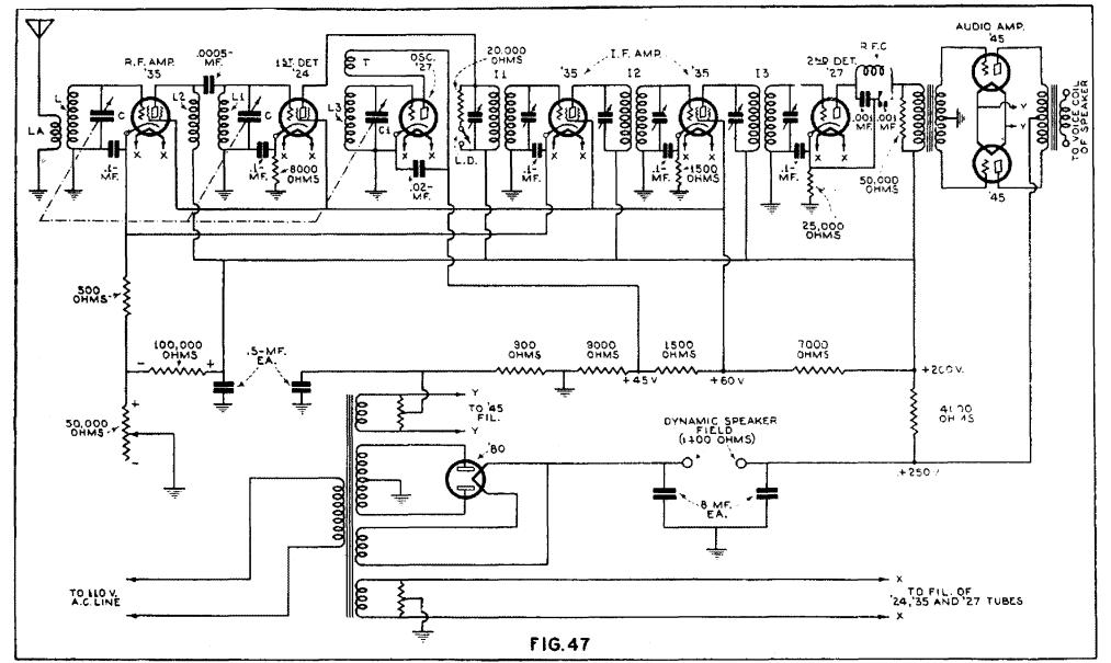
A complete superheterodyne circuit incorporating the design features described in the various preceeding chapters.
