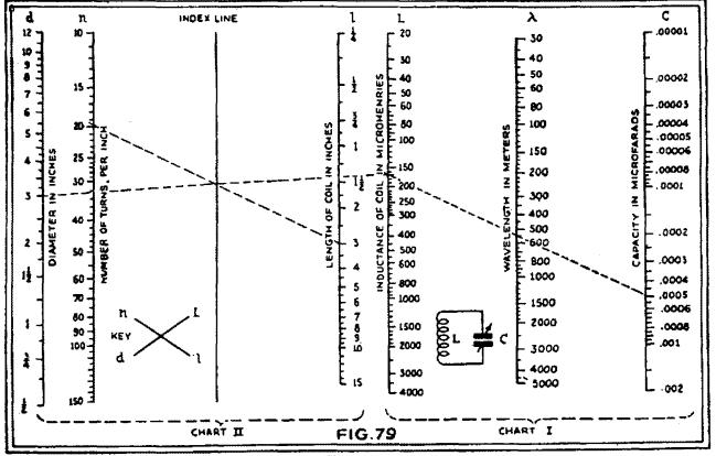
An automatic coll-condenser calculator. Knowing the value of either a coil or a tuning condenser, the other may be determined, for any wavelength by reference to the chart.
