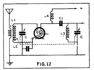
Antenna input circuit for uniform gain.
