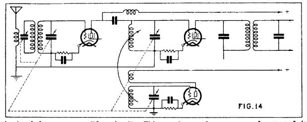
A signal frequency amplifier circuit. This requires a four gang condenser and is very selective.
