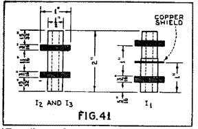
F. coils used in the circuit of Fig. 37.
