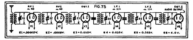
An elementary circuit illustrating how a signal is increased through an amplifier.
