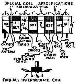
Fig. 58. Coil data for the midget super-het.
