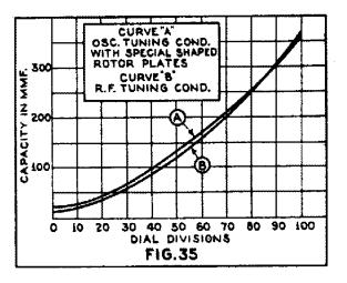
Typical capacity curve of oscillator condenser.
