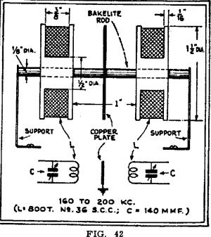
FIG. 42 Data for a home built I.F. transformer.
