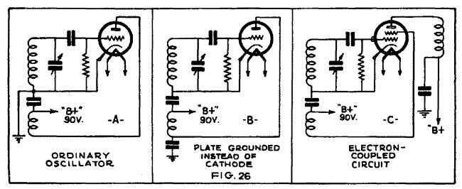
In the electron-coupled oscillator, the oscillatory circuit itself has not changed, the screen-grid merely taking the place of the plate used in A and B. This leaves the plate free to act as explained in the text.
