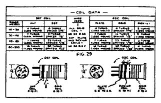
Coil data for oscillator and detector coils for a S.W. superhet.
