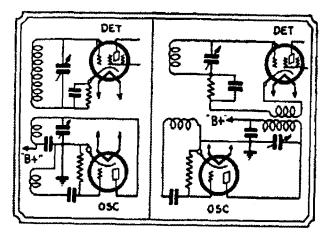
Fig. 21, left, illustrates magnetic coup-ling of detector and oscillator. Fig. 22, right, oscillator pick-up coil linked with a coil in cathode lead of detector.
