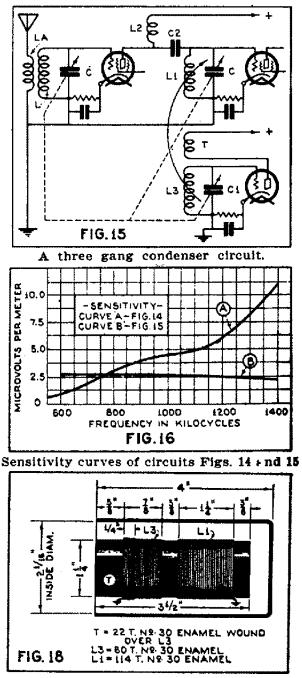
Oscillator coil data for circuit Fig. 15.
