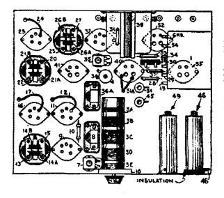
tors, are soldered in place during the process of wiring. In order to facilitate the wiring, the transformer (39) and the special coil (3-A-B-C-D-E) are mounted after wiring in most of the other parts.
