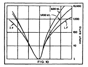
Selectivity curves. The curves are shown in the usual manner, the lowest point being at resonance and the two extremes 30 kc. off to either side. The height of the curve indicates the ratio in which input must be increased to maintain the same output which was obtained at resonance. This is, of course, an indication of the degree of discrimination against unwanted signals.
