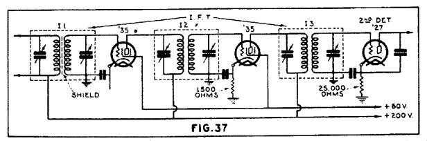
... two stage I.F. amplifier circuit. Note that three tuned I.F. transformers are employed.
