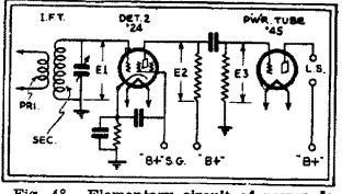
Fig. 43. Elementary circuit of power detector and output tube.
