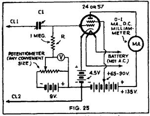
A V.T. voltmeter for adjusting the output of the oscillator to optimum value.
