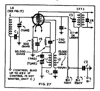
The method of connecting the pentagrid converter as a frequency changer.
