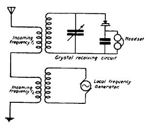
Fig. 3. A simple heterodyne receiver.
