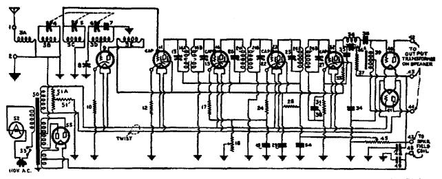
Fig. 53. Circuit of a homemade midget superheterodyne designed by Mr. H. G. Cisin.
