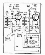
FIG. I—Circuit of frequency-doubling Idea. Lower right, frequency quadrupled.
