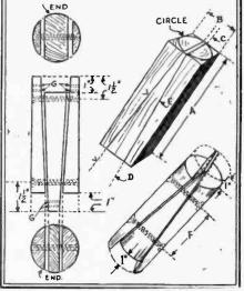
FIG. 6, 7 and 8—The various steps for form making are evident in this drawing.
