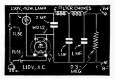
FIG. 10—A novel A.C.-D.C. "B" power supply, using a filament-type tube as rectifier.
