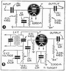
FIG. 5-Uses for old "tuning eye" tubes. target should be grounded when not used.
