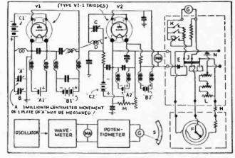
FIG. 7—Circuit of Electrical Ultra-Micrometer.
