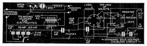
FIG. 6-Circuit for use of "tuning eye" as Indicator for condenser analyzer.
