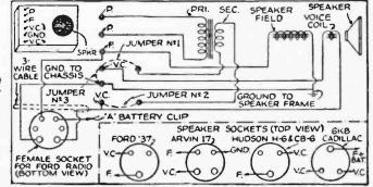
FIG. 2—A universal test speaker circuit and mechanical arrangement.
