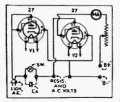
FIG. 4-Low-capacity condenser tester.
