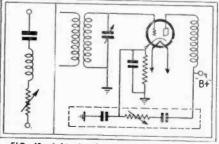
FIG. 13, right—Another hum-control connection. FIG. 14, left—Tone-control unit.
