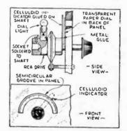
FIG. 2-Sketch of the dial shown in Fig. 2 A.
