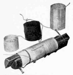
FIG. 10—Coils completed and in the course of construction are illustrated above.
