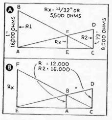
FIG. 4—Simple graphic calculating of parallel resistances.
