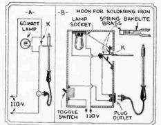
FIG. 6—A novel soldering iron holder. A, its electrical circuit; B, mechanical arrangement.
