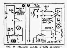
Important: Proper polarity must be observed in connecting the infinite resistance voltmeter in the circuit under test.
