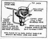
FIG. 6, above-Re-making a tip jack.
