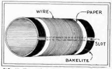
FIG. 12—The method shown makes it possible to prepare coils with lessened dialectric losses.
