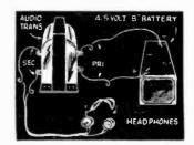
FIG. 6-Testing for noisy audio transformers.
