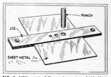
FIG. 8—With a set of jigs and punches of this kind, large, clean holes may be punched in fairly stout sheet metal.
