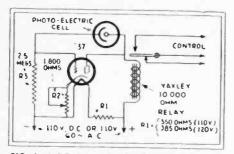
FIG. I-A P.E. tube relay for A.C. or D.C. mains.
