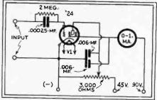
FIG. 15-Circuit of a Dynatron V.T. Voltmeter.
