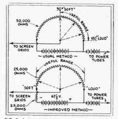
FIG. 2—Just as tuning is spread by adding another condenser, so volume control may be made less critical by a series fixed resistor.
