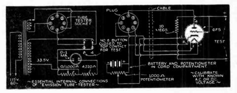
FIG. 13-Any emission-type tube tester may be used as a vacuum-tube voltmeter.
