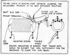
FIG. 14-A novel 3-circuit tuner.
