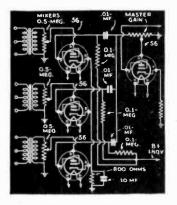
FIG. 4-Circuit of the low-cost mixer.
