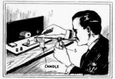
FIG. I—Blowpipes are obtainable from laboratory supply houses; but Mr. Kitchin takes this ingenious way to make one of light weight. (The bottle may be retained as a handle!)
