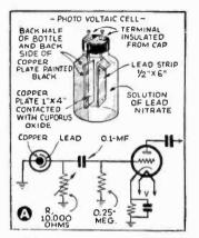
FIG. 22-Home-made photo-voltaic cell.
