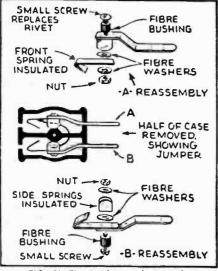
FIG. 21-The test-lamp adapter unit.
