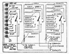
FIG. 24—A resistance-capacity box which saves time.
