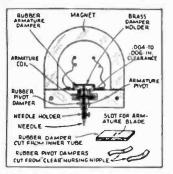
FIG. 6—Illustrating the method of repairing a pickup.
