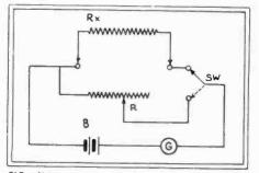
FIG. 25A—A good wire-wound potentiometer, a galvanometer, some calibrated resistance standards, and a few odds and ends, compose this handy instrument.
