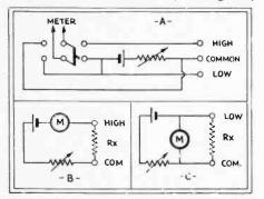
FIG. 23—In this ohmmeter the D.P.D.T. switch may be part of a larger unit.
