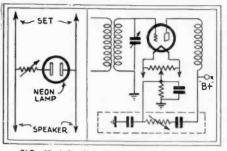
FIG. 11, left-Circuit of the static reducer. FIG. 12, right-Hum-control circuit.
