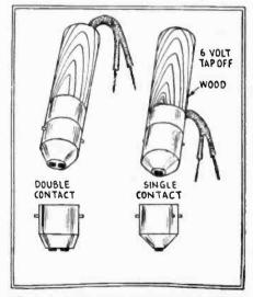
FIG. 7—A simple tap to the automobile storage battery will operate a receiver efficiently.
