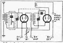
FIG. I-Design for a good volume control.
