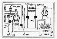
FIG. 21—This oscillator, with home-made power transformer, is an extremely-compact and convenient device, modulated by the A.C. hum of the light line. A jumper is put across the lower tip jacks when the meter is not in circuit.
