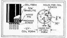
FIG. 11-Mounting coil-tubes to a plug-in base.
