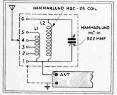
FIG. 15—The combination of low-loss tapped inductance and variable condenser makes this wavetrap adjustable for varying conditions.
