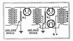
FIG. 4—These resistors give a solution of the persistent hum problem.
