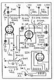
FIG. 14-A Veniatile V.T. Voltmeter.
