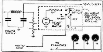
FIG. 16—A 6-volt supply for dry shaver from a car radio,
