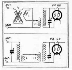
FIG. 3—Two band-pass arrangements which may be applied to give greater selectivity to a receiver.
