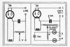
FIG. 26A, left—Theoretical circuit of the resistance calculator.
