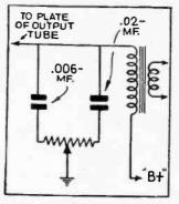
FIG. 4-A novel tone-control circuit.
