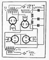
FIG. 11-Circuit of novel high-voltage power supply.
