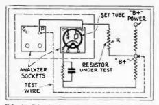
FIG. 18—This simple method of measuring voltage on both sides of a resistor, when the current is known, quickly gives its ohmage. (A high-resistance meter is needed.)
