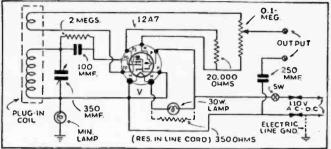
use, the 5-W miniature lamp is used as shown in Fig. 29. If the lamp lights when the plug is put in the socket, the plug should be reversed. Of course, a ground is needed on the oscillator for this test. This test should always be made; since if the plug is not inserted in the correct manner, the tuning condenser and some of the other parts of the unit will be "hot" and unless
