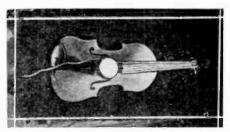
FIG. 8—The radio-violin. The improvised speaker unit, on the violin bridge, facilitates radio accompaniments.
