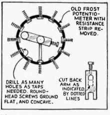
FIG. 9—A selector switch made from a volume control.
