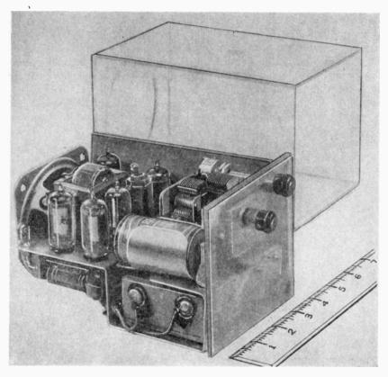
The "Miniport"-a 5-tube battery portable.
