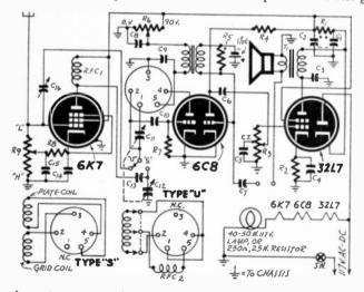
Fig. 1 — Schematic shows switching and plug-in combined.
