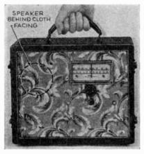
Panel of 4-tube broadcast band portable.
