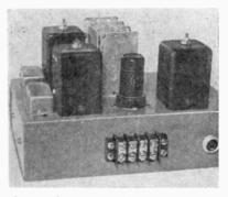
Fig. 3—Rear view of broadcast tuner, showing aerial connection (right) and terminal block for power and output.
