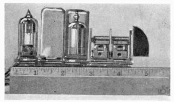
Chassis of the receiver — less than 41/2 inches long.
