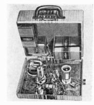
Above—Interior of ell-wave portable. Left—Portable battery set works loudspeaker.
