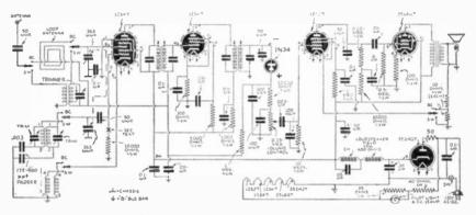
Fig. I—"Hook-up" for the "carry-around" A.C.-D.C. receiver.
