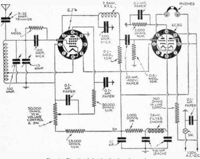
Fig. I—Circuit of 2-tube beginner's receiver.
