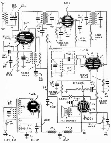
Fig. I—The 5-tube superhet circuit is simple and easily followed.
