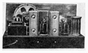
Rear view of 5-tube line-operated superheterodyne.
