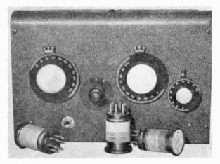
Fig. I—Front view of the Den receiver. Set is fitted with red and white dial knobs, which enhance its appearance. Set uses doublet single-wire antenna.
