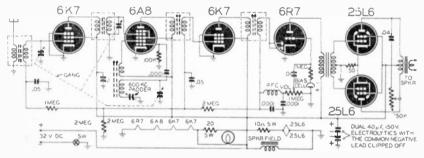
Fig. I-Schematic diagram of the 32-volt receiver.
