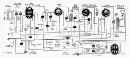
Fig. 2-Optional circuit for 110 volts A.C.-D.C.
