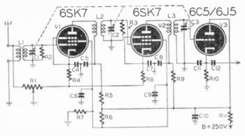
Fig. 5—Tuner is e 3-tube t.r.f. with infinite-impedance detector.
