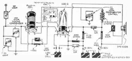
Fig. 2-Diagram of one-tube receiver.
