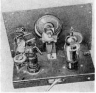
Using a 50,000 ohm potentiometer as the regeneration control, connected in series with a 50,000 ohm  $\frac{1}{2}$  watt resistor, and a bypass condenser of .1  $\mu$ f, ground to the buss, gives smooth operation.
