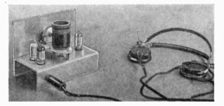
Rear view of 3-tube battery receiver.
