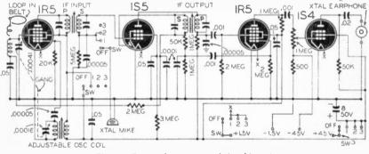
Fig. I—Four tubes are used in this set.
