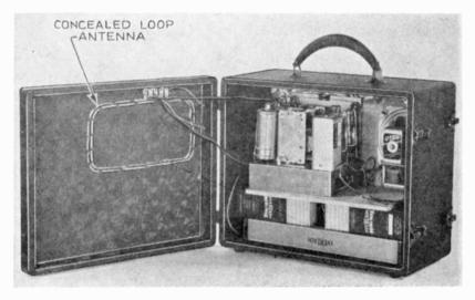
Rear view, with lid open, showing batteries.
