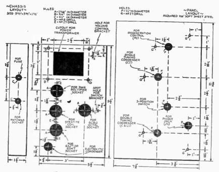
Fig. 4—Layout details for panel and chassis.
