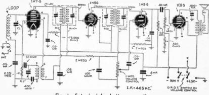
Fig. I—Set wired for battery operation.
