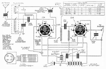
Fig. I-Circuit for 2-tube all-wave receiver.
