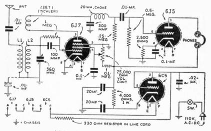
Wiring diagram of the "Midget 3-Tuber".
