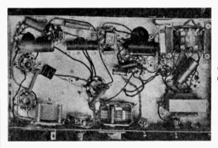
Bottom view of short-wave superhet receiver. Wiring and parts are not crowded. The low cost of the parts is rather due to the use of double-purpose tubes, and to the design of the circuits around tubes which require a minimum of circuit components.
