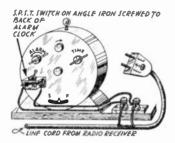
Radio cut-off switch made from alarm clock.
