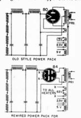
Rewiring power supply for 6.3 v tubes.
