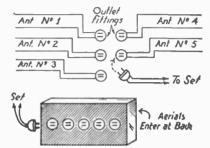
Plug-in switch for using different antennas.
