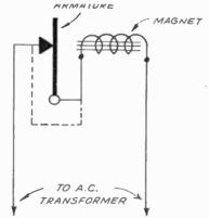
Doorbell noise eliminated by converting to a.c.
