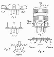
Plug-in coil from battery plug and socket.
