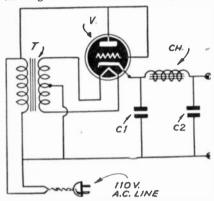
Simple power supply for test bench.
