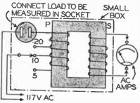
Using a transformer and an a.c. voltmeter to measure alternating current.
