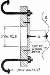
Simple jig for winding coils.
