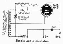
Actually it is nothing but a simple self-pulsing oscillator with the pulse rate falling in the desired part of the audio spectrum. The one I have at present is adjusted to oscillate at 800 cycles which is a standard m.c.w. (modulated continuous wave) frequency. If the coil specifications are followed, it will transmit a modulated c.w. signal which can be picked up on any broadcast set within 20 or 30 feet. No connections between the broadcast set and the oscillator are necessary.
