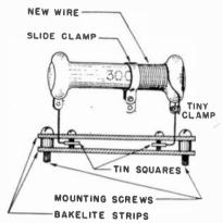
Odd-sized resistors from old insulated units.
