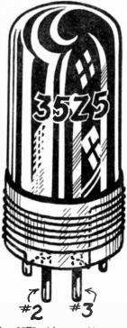
Repairing 35Z5 with open filament tap by winding resistance wire on base.
