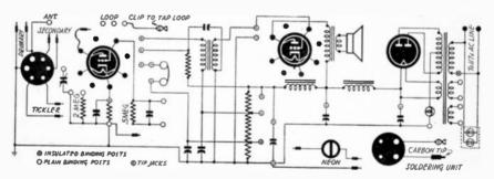
Layout with plug connections for making various tests—even a soldering iron is provided.
