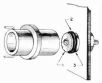
Rubber washer holds coil on chassis.
