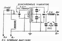
Power pack from vibrator and filament
