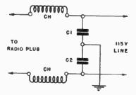
Simple line filter to eliminate noise.
