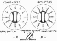
Capacity-resistor substitution box.
