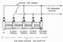
Increasing wattage capacity of resistor.
