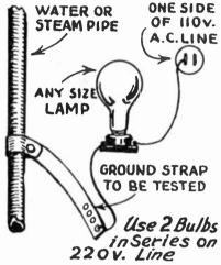
Simple ground test, using light bulb.
