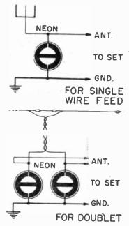
Neon lamps connected as lightning arrestors.
