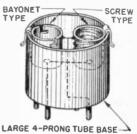
Pilot lamp tester from 4-prong tube base.
