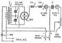
Capacity and leakage taster for condenser.
