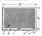
Portable antenna — A, copper screening. B, plywood strips. C, mounting screws. D, solder. E, lead to Ant. post.
