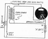
Charger from ignition coil and Tungar tube.
