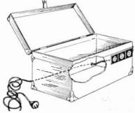
Multiple outlets on tool box permit plugging in radio set, soldering iron and tester at same time.
