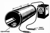
Circuit tester from coil and magnetic compass.
