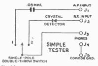
Flexible set tester for use with voltmeter.
