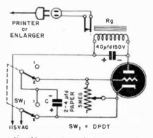
Adjustable time-interval circuit controller.
