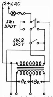
Auto-transformer hook-up to control line voltage.
