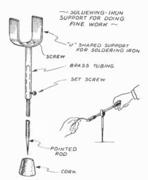
Soldering iron support for fine work.
