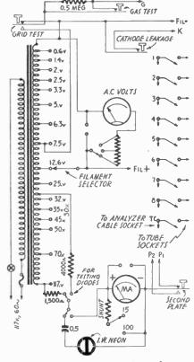
Handy tube tester with special transformer built from a power transformer. Tests all tubes. Uses neon "short" indicator.
