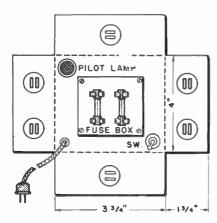
Pilot lamp and fuse for "test" outlets.
