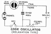
Code practice oscillator utilizing neon tube.
