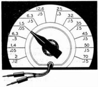
Resistance substitution box locates open filaments.
