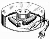
Noise filter built into outlet box.
