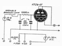
Volt-ohmmeter power supply, using 117Z6-GT tube.
