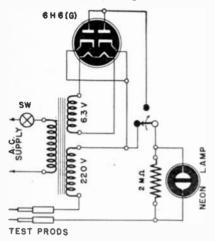
Condensers, including electrolytics, may be tested on a.c. or d.c. with this rig.
