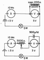
"Lag" and "lead" of current are demonstrable with these simple circuits.
