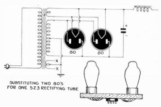
Using two 80's as a substitute for a 5Z3 rectifier.
