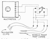
Quick reverser-switch for condenser tests.
