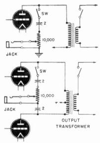
Top—adding phone jack to single tube output; Bottom—push-pull hook-up.
