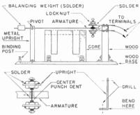
Audio transformer converted into sensitive relay.
