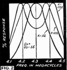
characteristics, which are symmetrically loaded with shunt resistors across the primary and secondary. These resistors have the two-fold purpose of providing (a) the proper Q and (b) a dissipative circuit which prevents the rapidly changing frequency from setting up transients. The latter may be heard as a "fuzz," particularly on loud, high-frequency passages.
