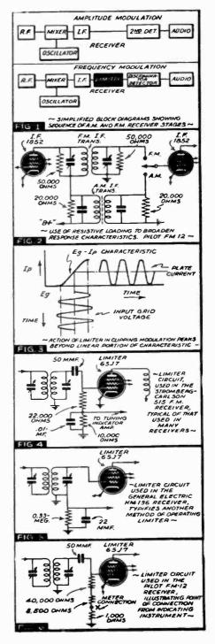
the voltage; and, the number of times per second, or Yate at which the I.F. signal swings above and below the resonant frequency, produces the audio signal.
