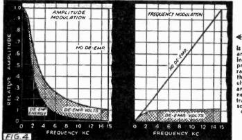
✓ Fig. 4. High-frequency pre-emphasis is used in the transmitter and de-emphasis is used in the receiver to improve the signal/noise ratio. The importance of this characteristic in ultra - H.F. broadcating and its greater effectiveness in F.M. are illustrated at left. Comparison is on the same scale of relative amplitude.
