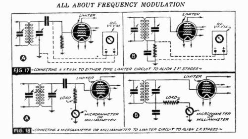
precaution mentioned in connection with matters without zero center must be observed. It is possible to change the zero adjustment of the meter to read up-scale to avoid slamming of the needle off-scale when the secondary trimmer is adjusted.
