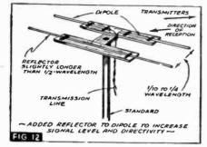
obtain the requisite rigidity, only wire of a heavy gauge, either No. 10 or No. 12, should be used, supported by low-loss insulators. The transmission line must be run at right-angles to the dipole for at least a 4-wavelength, at least 5 feet, before any bends in the line are made.
