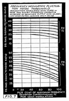
when the noise peaks equal or exceed the peaks of the carrier. The result is a rapid increase of the noise level or decrease of the signal-to-noise ratio with modulation.
