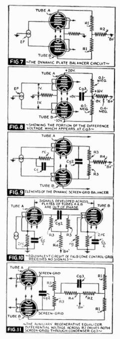
of both tubes, while R2 becomes the common degenerative resistor. If both tubes A and B have identical voltage amplification characteristics, the voltage which appears across R2 will be 0. On the other hand, if A has twice the voltage amplification of B, then a portion of this difference will appear across R2.
