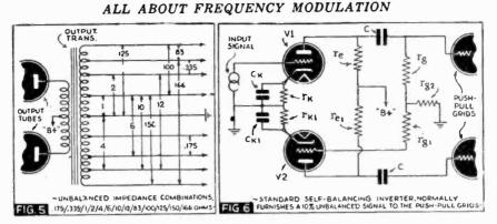
riety of impedances, which are obtained either by balanced or unbalanced loading. A balanced loading circuit is illustrated in Fig. 4. Figure 5 shows the unbalanced output terminals available, ranging from 0.175ohm to 166 ohms. It will be noted that a total of 16 impedance combinations are available, ranging from 0.175-ohm to 500 ohms.
