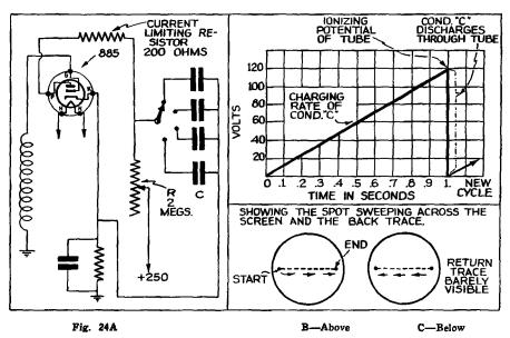
While Fig. 24B shows a linear charging rate for condenser C, this does not hold true in practice. Actually, the charging rate varies as the condenser approaches full charge, producing a bend at the top of the cycle. In practice, this bent part of the cycle is not used, only the linear portion being allowed to actuate the spot.
