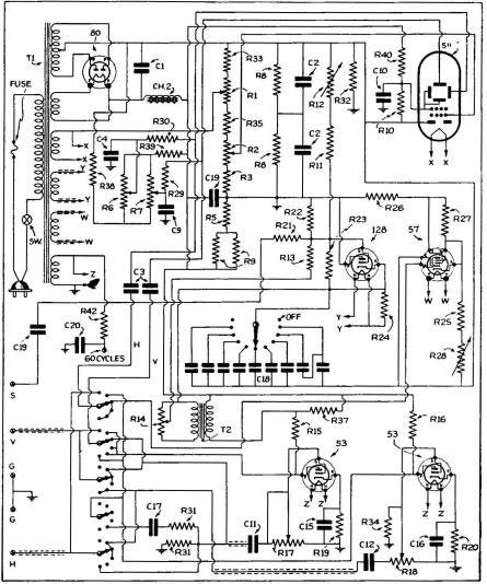
Fig. 29A. Schematic of Model 148 Dumont 3" Oscillograph
