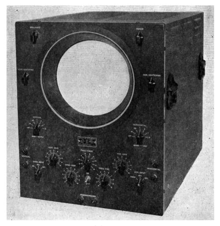
Fig. 30. RCA 9" Oscillograph Model TMV-168A
