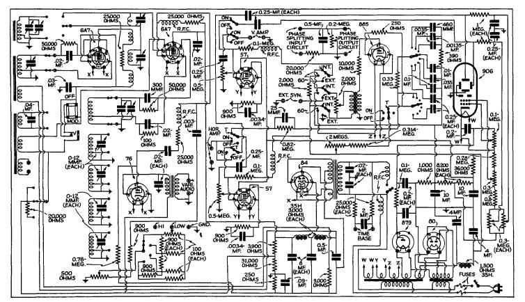
Fig. 12. Diagram of Model 555 Supreme Diagnomoscope.
