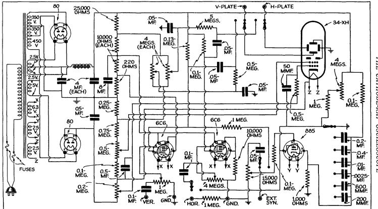
Fig. 22. Schematic of Model 546 Supreme 3"
