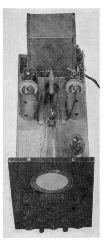
Fig. 19 RCA 3" Oscillograph with Cover Removed
