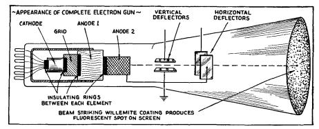
In Fig. 5 is shown the appearance of a complete tube. Note the two pairs of Deflecting
