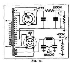
the same circuit with the high-potential side grounded.Then, in Fig. 15, we add the lowvoltage rectifier, which supplies current to all the other tubes in the circuit. Finally,
