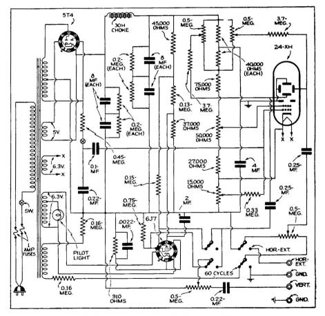
Fig. 11. Schematic of Model 530 Supreme Oscilloscope.
