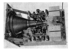
Fig. 31. Interior View of 9" RCA Oscillograph—Schematic on Page 25
