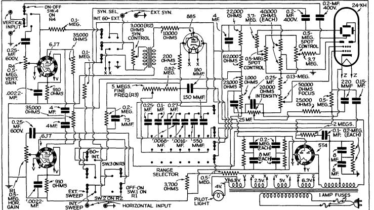
Fig. 21. Schematic of Model 535 Supreme 2".
