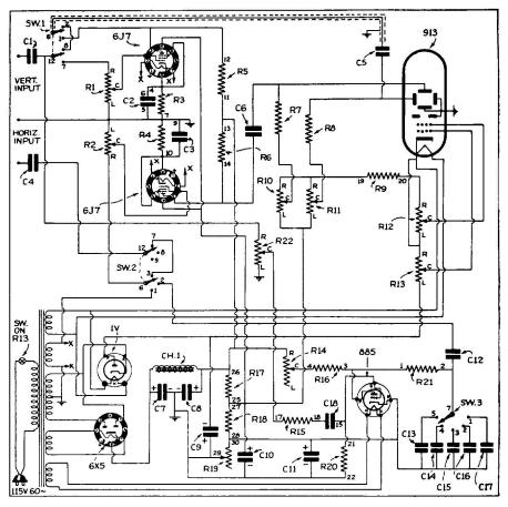
Fig. 37 Schematic of Thordarson Oscilloscope
