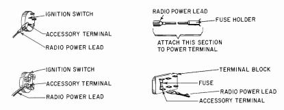
Fig. 325. Radio power-lead connecting points.
