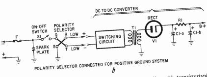
Fig. 305. Polarity-reversing circuits used in universal auto radios with transistorized
