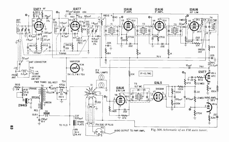
universal models with isolated common chassis, this ground return was provided by the mechanical connections between the radio and the auto chassis.
