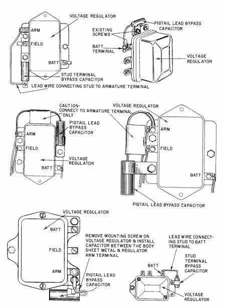
Fig. 804. Installation of bypass capacitors at voltage regulators.
