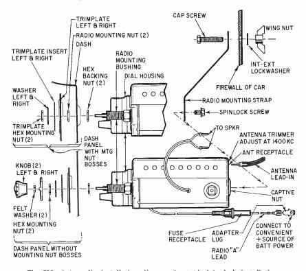
Fig. 318. Auto radio installation diagram for typical in-dash installation.
