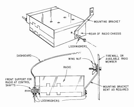
Fig. 316. Basic mechanical connections for in-dash installations.
