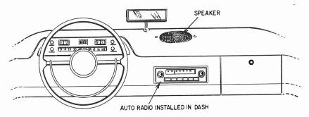
Fig. 301. Typical in-dash installation of an auto radio.
