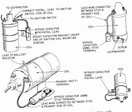
Fig. 805. Installation of bypass capacitors at ignition coils.
