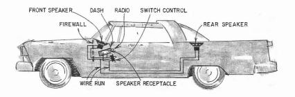
Fig. 401. Typical rear-speaker installation includes the speaker, a wire run and a switching device located in the dash.
