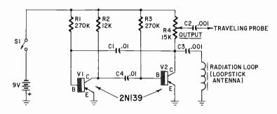
Fig. 213. Schematic diagram of a noise generator.
