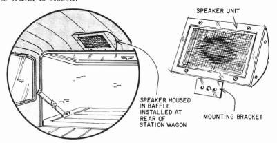
Fig. 410. The rear-speaker unit for a station wagon comes equipped with a mounting bracket.
