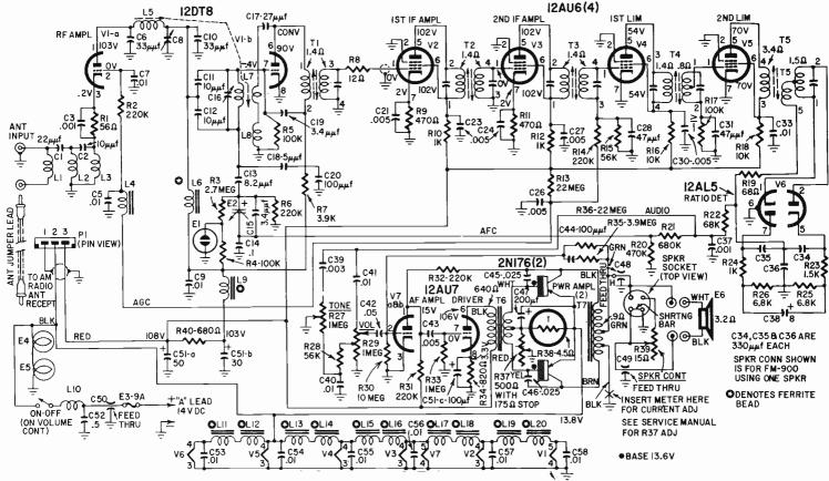
Fig. 902. Circuit diagram of the FM-only auto-radio receiver.
