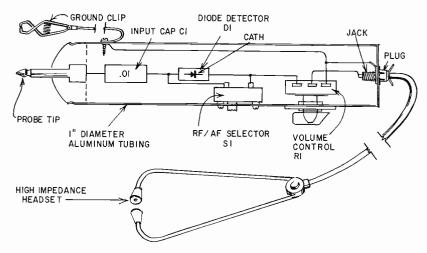
Fig. 216. Physical layout of the signal tracer probe.
