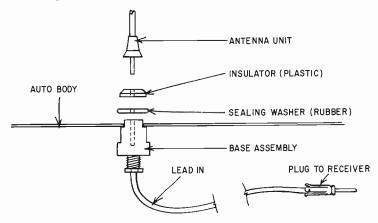
Fig. 309. Typical auto radio antenna assembly.
