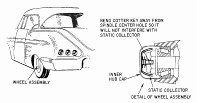
Fig. 813. Typical wheel-assembly static-collector installation.
