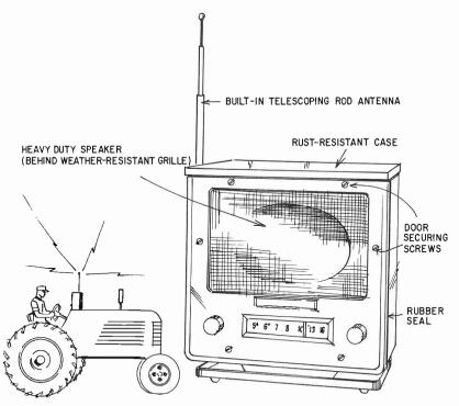
Fig. 209. Weatherproof auto radio for use in open vehicles has a rust-resistant case with rubber-sealed doors.
