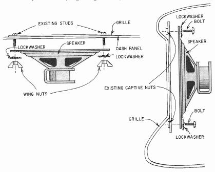
Fig. 314. Installing speakers using existing hardware on dashboard panel.
