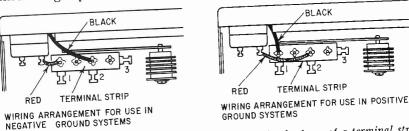
Fig. 308. A polarity selector for universal auto radios in the form of a terminal strip that is wired per instructions.
