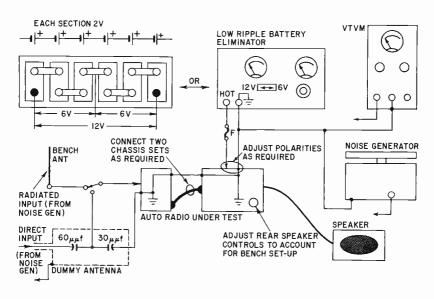
Fig. 510. Bench setup for servicing auto radios.
