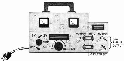
Fig. 212. Battery eliminator used with L-C filter.
