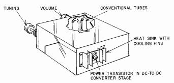
Fig. 203. Transistor-powered dc-to-dc converter auto radio (rear view) with cutaway showing conventional tubes.
