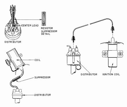
Fig. 809. Typical installation of suppressor resistors at the distributor. Caution: some cars have an ignition interference suppressor built into the distributor cap or ignition leads. Do not install a second suppressor as high resistance affects engine performance. To put in a suppressor, cut the center distributor lead and screw the suppressor resistor in series with the two pieces of wire.
