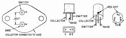
Fig. 512. How to locate and identify transistor electrodes.
