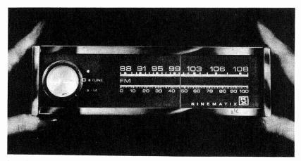
Fig. 207. FM tuner for use in autos with an existing AM radio system. (Kinematix, lnc.)
