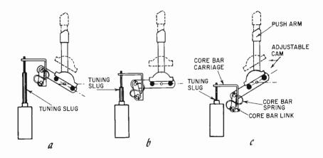
Fig. 604. Three different angles of cam action in pushbutton tuning.
