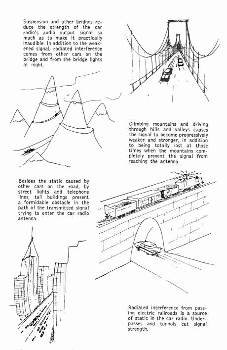
Fig. 105. The auto radio must provide an adequate audio signal that remains relatively constant in strength under varying road conditions.
