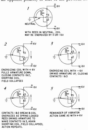
Fig. 702. Typical vibrator operation.
