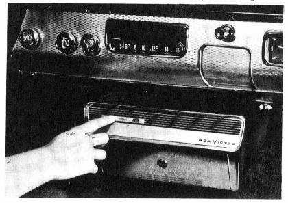
Fig. 911. The 45-rpm record changer automobile phonograph.
