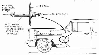
Fig. 807. Feedthrough capacitor installed in the firewall.
