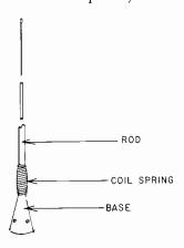
Fig. 310. Anti-vandal antenna incorporating a powerful coil spring between base and rod.
