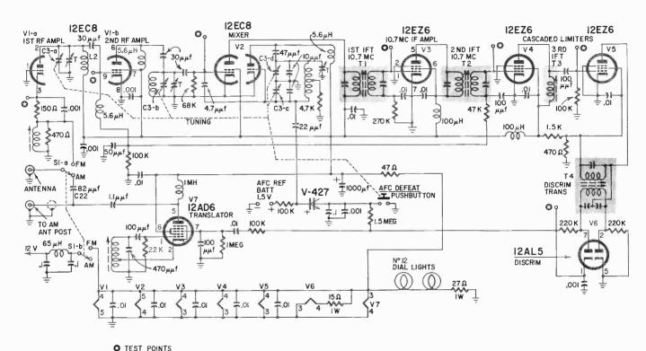
Fig. 509. Schematic of FM converter for use with an AM auto radio.
