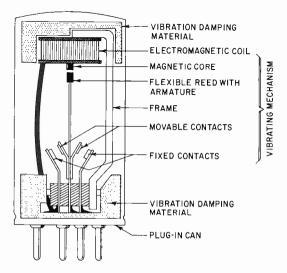
Fig. 701. Internal construction of a non-synchronous vibrator.
