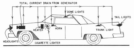
Fig. 102. For auto radio operation, available current drain is determined by the number of accessory units operated from the same generator.
