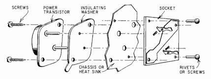
Fig. 516. Exploded view of power transistor mounting. Mica washer coated with silicone grease electrically isolates transistor case from chassis.
