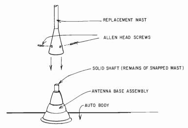
Fig. 311. Installing a replacement mast.
