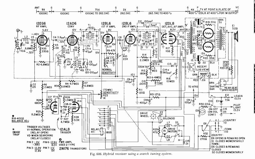
hybrid auto radios). This typical electronics section includes trigger tube V1-a, relay tube V1-b, search relay RY1, country pushbutton S1, town pushbutton S2, drive motor B1 and reversing switch S3. The circuit also shows the radio's first and second if stages, and the detector—avc—first audio stage. These stages provide the lock-in control signal for the search-tuner electronics section.
