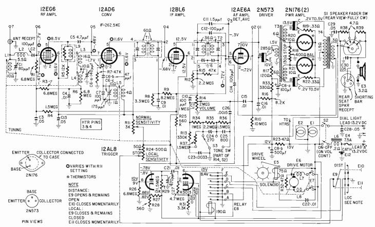
Fig. 507. Schematic diagram of a hybrid auto radio having a search tuner and push-pull output stage.
