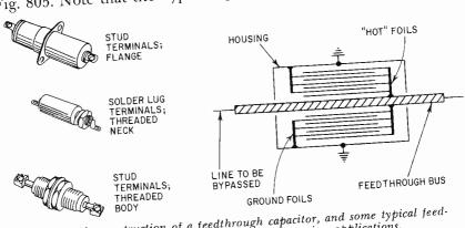
Fig. 806. The construction of a feedthrough capacitor, and some typical feedthrough capacitors for interference suppression applications.
