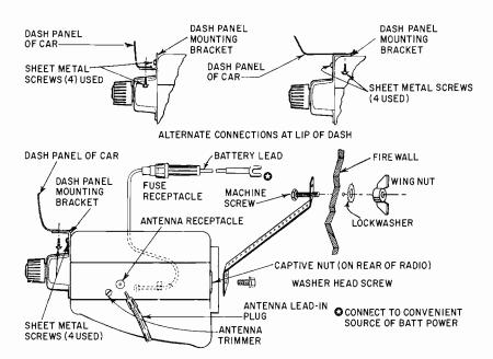
Fig. 322. Auto radio installation diagram for alternate under-dash installation.
