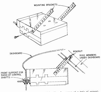
Fig. 317. The receiver can be held in place by means of a pair of mounting brackets. The brackets supply rear support for the radio, while the controls (going through the dashboard) give front support. The mounting brackets have holes punched in them. Select that pair of holes which will permit the receiver to be mounted in a horizontal position. If this isn't done, the control shafts will be tilted up or down.
