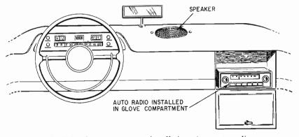
Fig. 303. Glove-compartment installation of an auto radio.
