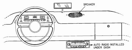
Fig. 302. Under-dash installation of an auto radio.
