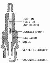
Fig. 808. Cutaway view of a resistor spark plug.
