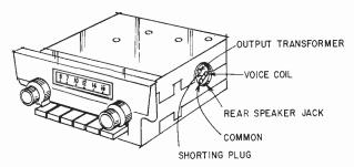
Fig. 406. Auto radio has built-in rear-speaker jack equipped with a shorting plug.
