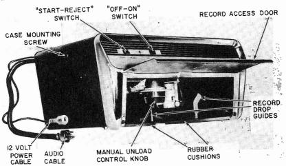
Fig. 913. Internal view of the 45-rpm automobile phonograph.
