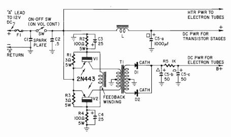
Fig. 706. Secondary power supply for a 12-volt negative-ground electron tube autousing a transistorized dc-to-dc converter in multivibrator configuration.
