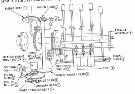
Fig. 607. Detailed mechanical analysis of a search tuning system.
