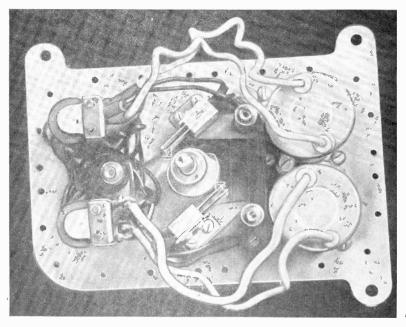
Fig. 704—Cam-type limit switches and neutralizing relays. The relays are shown at the left; servomotors at the right.
