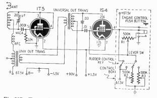
Fig. 907-Transmitter designed for use with a reed decoder.
