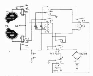
Fig. 506—Relay chain used to control operation of a motor.
