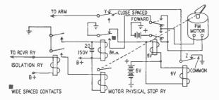
Fig. 1021-Relay system for numerical-sequence decoder.
