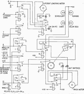
Fig. 1025-Circuit for control of lights, winch, and lifeboat.
