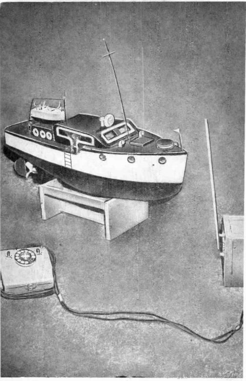
Radio-controlled model boat using a telephone dial coder.
