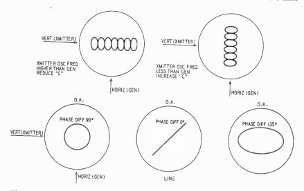
Fig. 906-Lissajous figures obtained in checking frequency of tone modulators.
