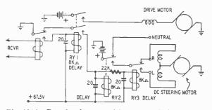
Fig. 1014-Decoder for use with pulse-variation coder.
