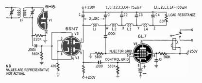
Fig. 520-Representative delay line circuit used as a decoder. Action of the decoder depends upon pulse timing.
