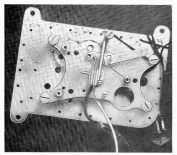
Fig. 1010—Pulse-variation coder. Note that the tip of the nut closes the switch contacts.
