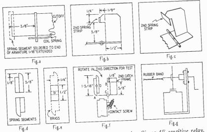
Fig. 1006-Construction details of escapement using Sigma 4F sensitive relay.
