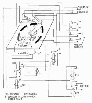
Fig. 1030-Pulse-presence pulse-omission coder.
