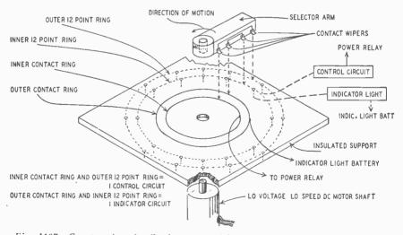
Fig. 1107-Construction details for snotor-driven, two-circuit, 12-point selector switch.
