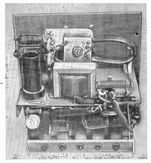
Fig. 905—Parts layout for the tone-modulated transmitter using push-pull 6C4's.
