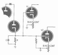
Fig. 521-Counting circuit decoder.
