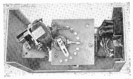
Fig. 1023-Top view of numerical-sequence decoder, showing contact arm assembly.
