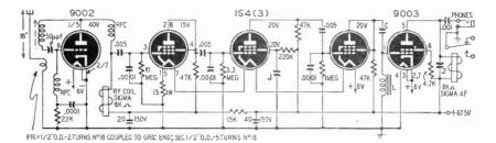
Fig. 807—Tone-operated receiver using band-pass filter in grid circuit of relay tube.
