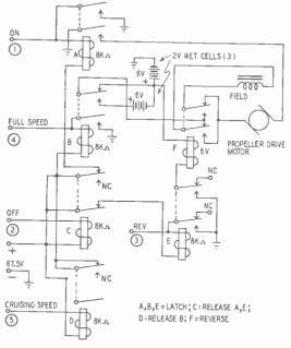
Fig. 1024—Motor control circuit for model boat.
