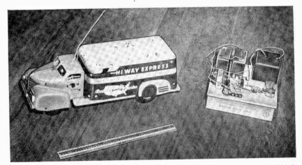
Fig. 1106—The transmitter is shown at the right. The receiver is concealed in the truck at the left.
