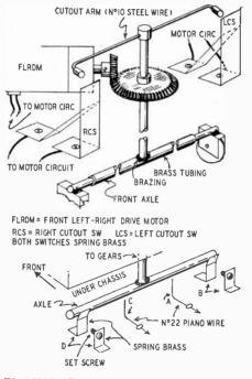
Fig. 1110—Details for building steering mechanism.
