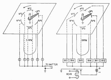
Fig. 511-Motor-driven commutator-type coder and decoder.
