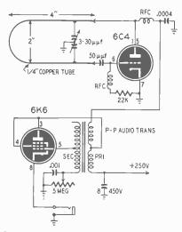
Fig. 902—Transmitter including a tone modulator.
