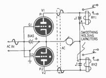
Fig. 604-Power control using gas tubes.
