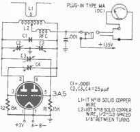
Fig. 901—Simple transmitter for use with Aerotrol or Goode receivers.
