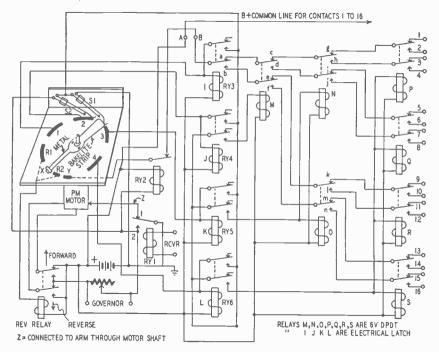
Fig. 1031—The decoder routs power through points A and B. Speed of rotation of the decoder arm can be controlled by a governor.
