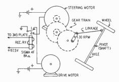
Fig. 1102—Details of the axle to gear linkage.
