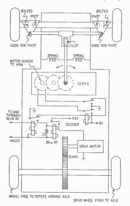
Fig. 1012-Delay decoder used in model car.
