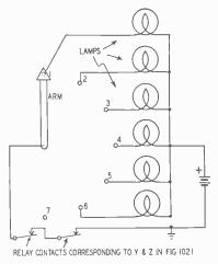
Fig. 1022—Test unit for numericalsequence coder.
