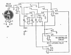
Fig. 507-Relay chain decoder using only one relay tube.
