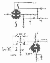
that it has a common ground for input Fig. 515-Twin-T in grid circuit of and output and is more adaptable than second half of duo-triode. Fig. 516-Typical Twin-T used in input stage. drawings courtesy of McGraw-Hill. ground potential. A representative circuit employing the twin-T appears in Fig.
