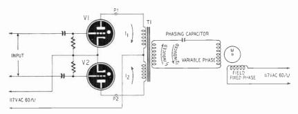
Fig. 605-Bidirectional and speed control of a motor using push-pull thyratrons.
