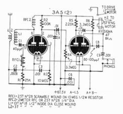
Fig. 1103-Superregenerative receiver using a pair of 3A5's. If set does not superregenerate, increase C2 and substitute 2.5 mh choke for RFC1. For model plane use, increase R2 and R5 to 470,000 ohms for greater stability.
