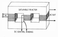
Fig. 606—Saturable reactor type transformer.
