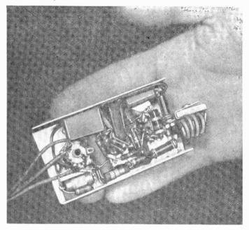
Fig. 805-Wiring and parts layout for the three-tube receiver.
