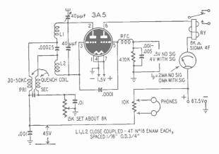
Fig. 803-Modified Goode receiver using Sigma 4F relay.
