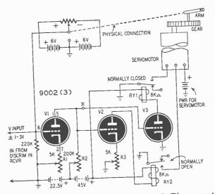
Fig. 706—Circuit for proportional control. The amount of turn is proportional to the deviation in frequency.
