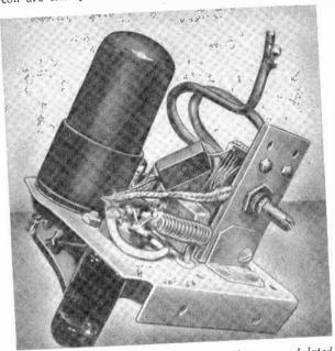
Fig. 903—Compact physical layout of tone-modulated transmitter.
