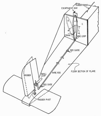
Fig. 1008-Rudder control in model plane by means of an escapement.
