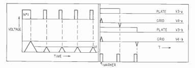
Fig. 528—Timing of marker, rectangular, and triangular pulses.
