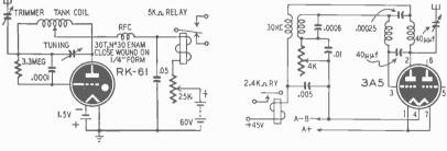
Fig. 801—The Aerotrol one-tube Fig. 802—The Goode one-tube receiver.
