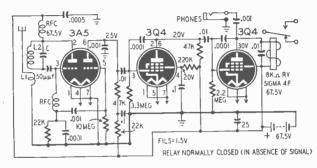
Fig. 804—Tone-operated receiver using superregenerative detector.
