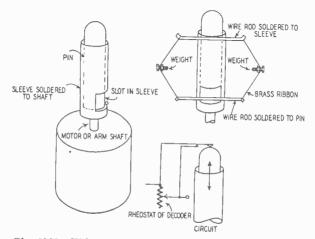
Fig. 1032—This governor is connected to the rheostat of the decoder shown in Fig. 1031.
