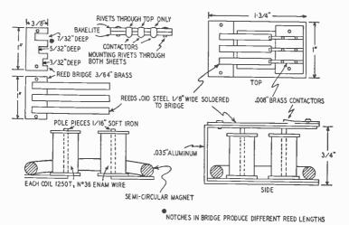
Fig. 1026—Details for construction of resonant-reed decoder.
