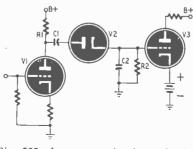
Fig. 525—Integrator circuit used with diode.
