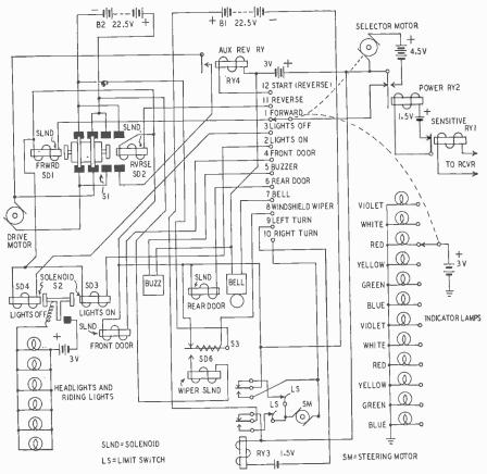
Fig. 1108—Master control diagram. Solcnoids and relays in this circuit are controlled by the receiver output.
