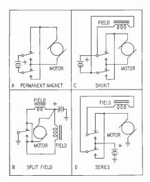
Fig. 603—Reversing relays can control motor rotation.
