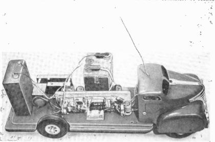
Fig. 1104-The receiver, batteries, and motor are mounted on the truck frame.
