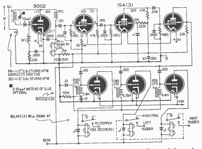
Fig. 808—Tone-operated receiver using three band-pass filters and three relay tubes.
