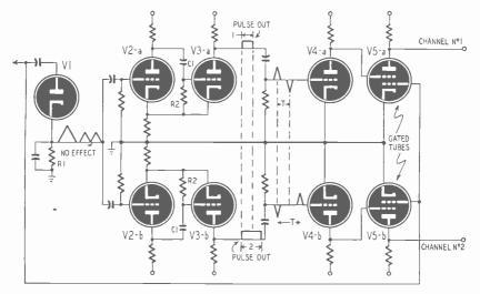
Fig. 527—Complete gating circuit, including a differentiating and an integrating network.
