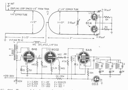
Fig. 904—Tone-modulated transmitter using 6C4's in push-pull. The modulator is a transitron oscillator.
