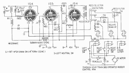
Fig. 810-Receiver using three vibrating reeds as decoders. The reed coil forms the plate load for the 1S4.
