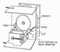
Fig. 509-Relay-driven stepper.
