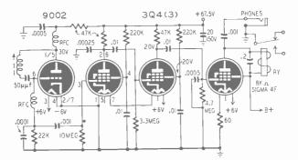
Fig. 806—The use of a 9002 in the superregenerative stage increases the sensitivity.
