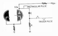
Fig. 526—Differentiator used with vacuum tube. The tube is part of a multivibrator circuit. The differentiator is shorted when the tube conducts. The tube produces a rectangular pulse which is differentiated into a triangular trigger pulse.
