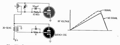
Fig. 403—Superregenerative receiver using a separate quench oscillator. The r.f. voltage increases with signal.
