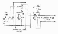
Fig. 505-Relay chain using two relays.
