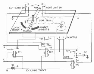
Fig. 703—Neutralizing switch controlled through the use of a moving arm and a pair of limit switches.
