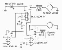
Fig. 1011-Decoder using a delay relay.
