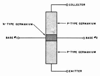
Fig. 1207. Cross-section of the tetrode transistor.
