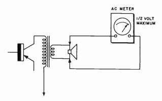
Fig. 1010. The maximum voltage indicated by your output meter should be about 0.5 volt. If it is more than this, your generator output is too high or one of the stages in the receiver (such as an if) is oscillating.
