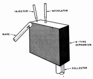
Fig. 1216. The Spacistor resembles a vacuum tube in its operation.
