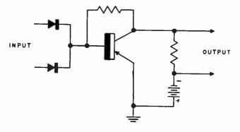
Fig. 1217. Simple transistor gate circuit.
