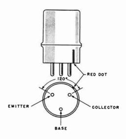
Fig. 1205. Surface-barrier transistor.
