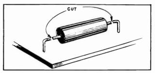
Fig. 1104. To remove a resistor or capacitor, cut the leads as close to the body of the component as possible.
