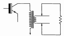
Fig. 816. Put a dummy load across the secondary of the audio output transformer if you want to make tests with the speaker disconnected.
