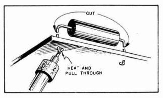
Fig. 1106. To remove a component such as a resistor or capacitor, cut the ends as shown and then heat the remaining leads, pulling them through the board when they become sufficiently loose.
