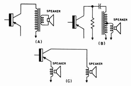
Fig. 917. Three methods of coupling a speaker to the output stage. That shown in (A) is most common. (B) is rarely used while (C) is a possibility being explored for future sets.
