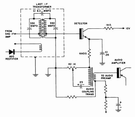
Fig. 910. Transistor detector. Note the use of a separate age rectifier.
