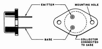
Fig. 1210. P-n-p high-frequency power transistor for use in television deflection circuits.
