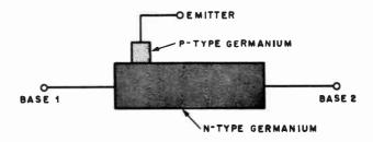
Fig. 1215, Cross-section of the Unifunction transistor.
