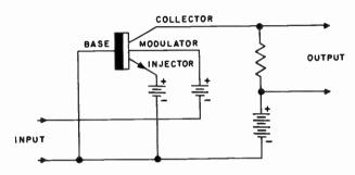
Fig. 1220. Simple Spacistor amplifier circuit.
