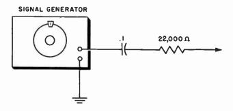
Fig. 817. Use a blocking capacitor in series with the hot lead of the generator. A 22,000-ohm 1/2-watt resistor will provide isolation when checking in rf or if stages. The resistor isn't needed for audio circuit testing.
