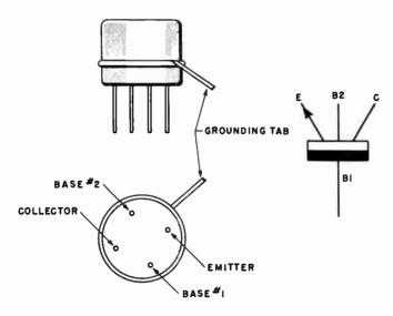
Fig. 1208. The tetrode transistor and its electronic symbol.
