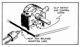
Fig. 1110. Method of removing a volume control.
