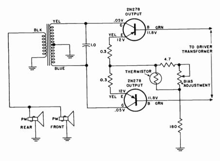
Fig. 916. Push-pull power output circuit.
