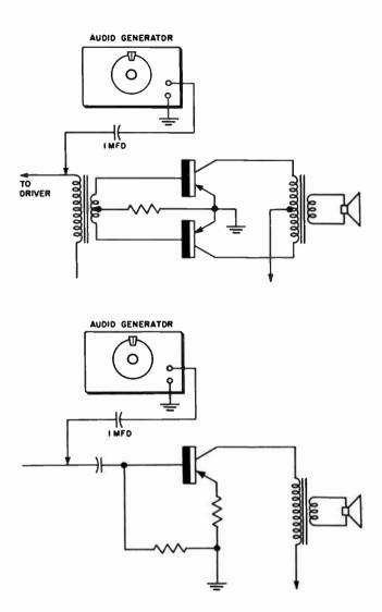
Fig. 807. Methods for checking single-ended and push-pull audio output stages.
