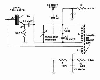
Fig. 907. Local-oscillator stage.
