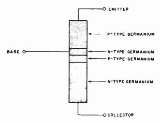
Fig. 1212. The hook transistor is a two-layer unit.
