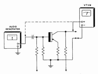
Fig. 712. Checking the gain of a suspected transistor stage.
