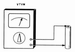
Fig. 704. To check the low-voltage scales of your vivm, set the range switch to read low volts dc and then use a fresh penlight cell (or other type of dry cell) as a calibrating voltage. Low-voltage measurements in transistor receivers are very important.
