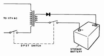
Fig. 709. A dry rectifier type charger can be used to keep the the test storage batteries in ready operating condition. The double-pole single-throw (dpst) switch should be in the off position when the battery is in use.
