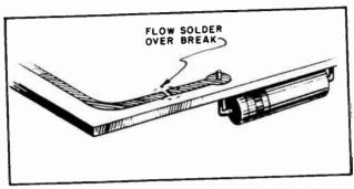
Fig. 1107. If the break in the conductor is small enough, you can repair it by flowing some solder between the two open ends.
