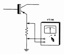
Fig. 1017. Methods of connecting the vtvm across the emitter resistor for n-p-n and p-n-p transistors.
