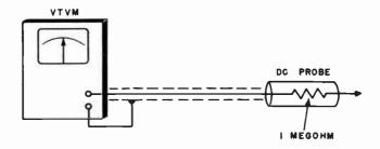
Fig. 1004. The dc probe contains a 1-megohm resistor. This is part of the input resistance of the instrument.
