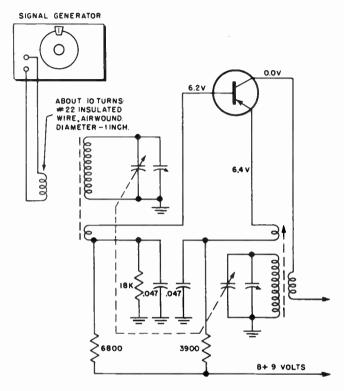
Fig. 812. Method of checking the converter stage.
