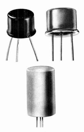
Fig. 1014. Some transistor types.
