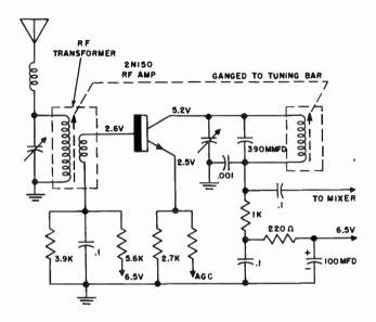
Fig. 905. Typical auto radio rf amplifier stage.
