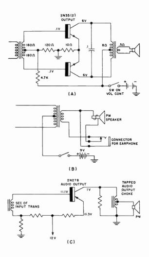
Fig. 805. Some transistors have loudspeaker output only. Others have one or more jacks for earphones. Impedance coupling is used in Fig. 805-C. The choke is tapped down to match the impedance of the voice coil. In some radios, the phone jack is placed at the output of the driver stage instead of the push-pull stage.
