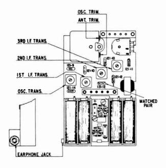
Fig. 1009, Layout of alignment adjustments in a typical receiver.
