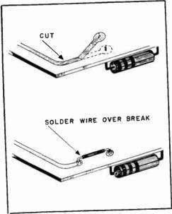
Fig. 1108. If a small bit of the printed-circuit conductor lifts up, cut it away and replace it with some wire.
