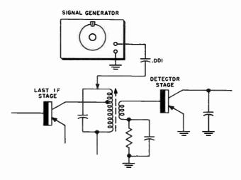
Fig. 808. Method for checking the transistor detector stage.
