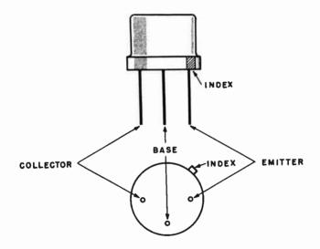
Fig. 1206. Silicon transistor.
