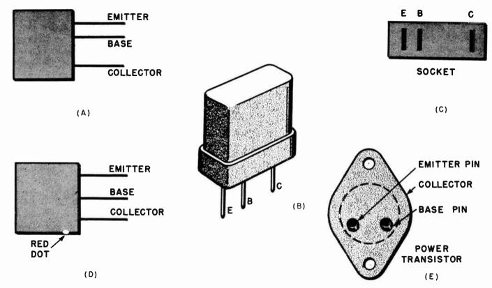
Fig. 1013. These drawings represent some examples of transistor pin arrangements; others are used.
