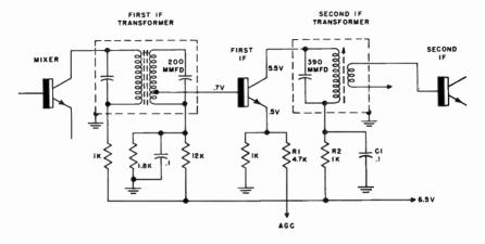
Fig. 909. Typical if stage in an auto receiver.
