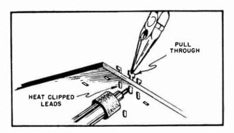
Fig. 1111. This drawing illustrates the method for removing volume-control connecting terminals.
