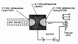
Fig. 1203. Cross-section of the phototransistor.
