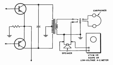
Fig. 1008. Five types of indicators that can be used during alignment: speaker, earphones, vivm, scope or low-voltage ac meter.
