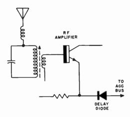
Fig. 914. A crystal diode can be used to delay the application of age voltage to the rf amplifier.
