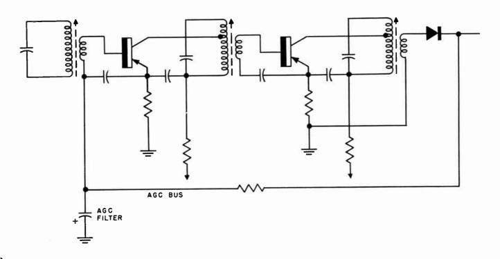
Fig. 810. Defective resistors and capacitors in the agc bus can result in oscillation.
