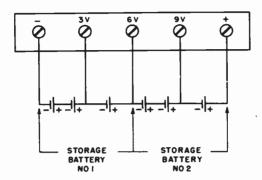
Fig. 708. A pair of 6-volt storage batteries or a single 12-volt battery will supply all the voltage and current needed for testing transistor receivers.
