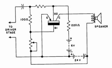
Fig. 1221. Amplifier circuit using a tetrode transistor.
