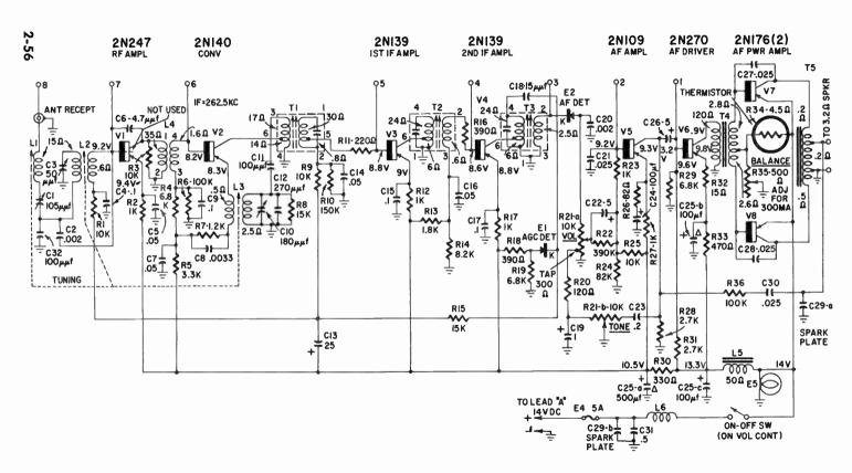
Fig. 903. Auto radio using transistors only.
