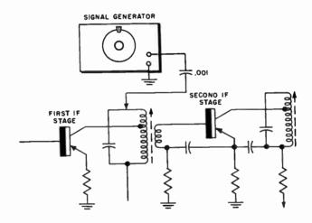
Fig. 809. Method for checking the if stages.
