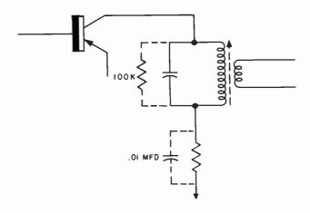
Fig. 811. A 100,000-ohm resistor shunted across the primary of the if transformer and an additional decoupling capacitor (.01 μf) will help kill oscillation.
