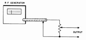
Fig. 701. Some signal generators have an audio output connection but no provision is made for controlling the audio level. You can make a simple control unit with a 500,000-ohm potentiometer as shown.
