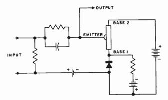
Fig. 1218. Pulse amplifier using Unijunction transistor.
