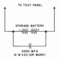
Fig. 1006. A high value of capacitance shunted across the test storage battery keeps the overall impedance low.
