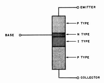
Fig. 1213. Intrinsic junction transistor.
