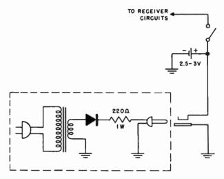
Fig. 1007. Charging unit is used in receivers having nickelcadmium batteries.
