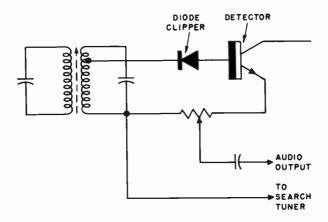
Fig. 911. A diode is sometimes placed in series with the base of the detector transistor.
